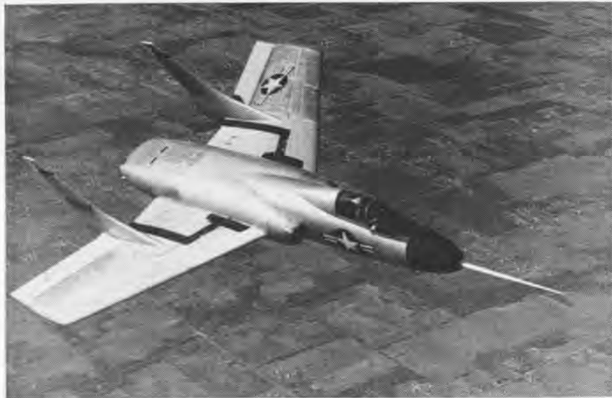
ONE OF several airplanes the Navy has in the mill which will run rings around the Soviet MIG-15 is the twin-jet streak pictured here, the F7U-3 Cutlass, shown here for the first time from above. This Chance Vought carrier fighter is the heaviest fighter plane in Navy history, eclipsing even the twin-jet F3D which carries two men. The long tail houses afterburners which give the Cutlass plenty of extra speed in a pinch, if needed
