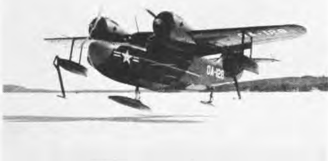
SAME JRF-5 PLANE SHOWN WITH SKIS MODIFIED FOR SNOW, ICE WORK
