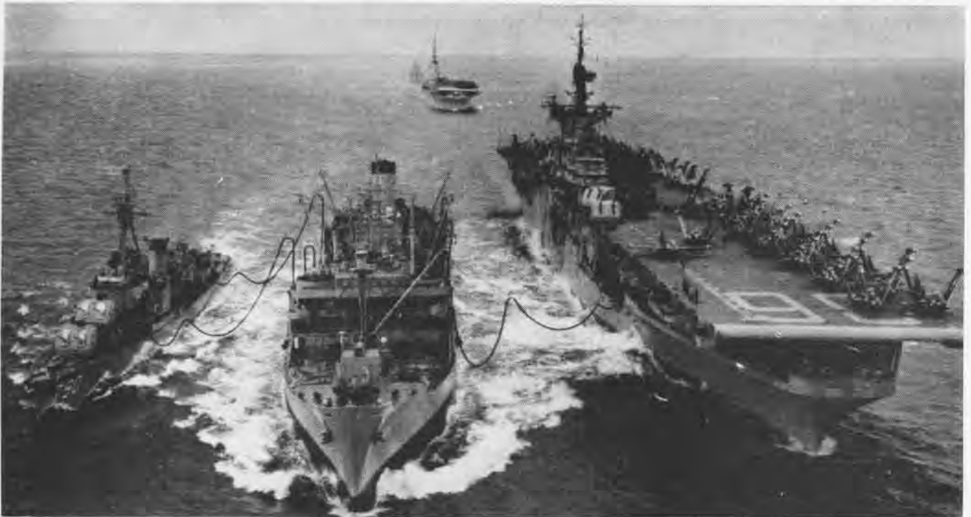
ANTIETAM AND DD REFUEL FROM TANKER WHILE ESSEX WAITS TURN. SUCH OPERATIONS AT SEA PROVIDE UNLIMITED TASK FORCE RANGE
