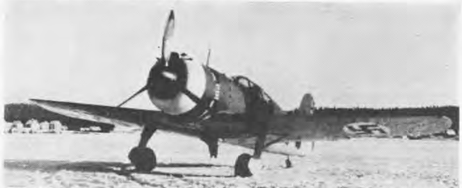
FRONT VIEW OF FINN'S MYRSKY FIGHTER RESEMBLES F-47, AIRPLANE HAD P&W 1,065-HP ENGINE
