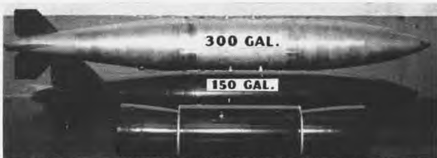
NEW STYLE TANKS, WITH A 150-GALLON ONE DISASSEMBLED AND NESTED, SHOW SPACE SAVING
