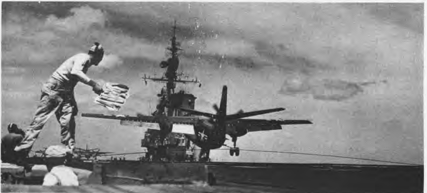
GREATER PERFORMANCE OF MODERN AIRCRAFT LIKE THIS AJ-1 CATCHING THE MIDWAY'S WIRE DEMAND GREATER CARRIER PERFORMANCE
