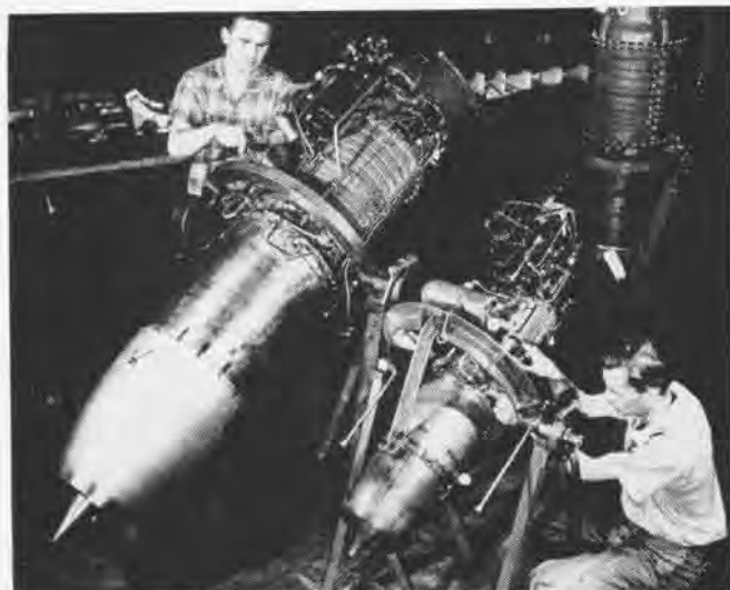
PROGRESS that has been made in development of Navy jet engines in the past seven years is graphically shown in these two pictures, showing 1945 and 1952 versions of Westinghouse axial-flow jets. On the left is the first jet to power an operational aircraft, the J-30 Phantom. This J-30 jet developed 1650 pounds thrust and was about seven feet long. Beside it is the midget J-32, with 9 1/2" diameter and 275 hp, used in guided missiles. Compare those two trail-blazers with the giant J-40 Westinghouse jet, latest in the Navy's fold. This will
