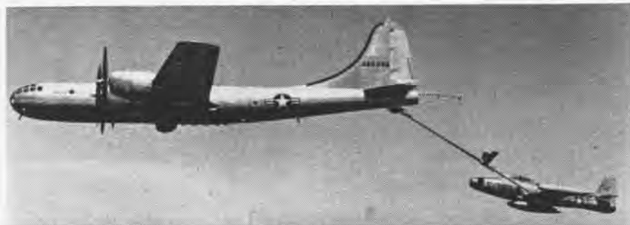
FLYING BOOM FROM RB-29 HOOKS ONTO WING EDGE REFUELING SNOUT ON SLOWED-DOWN F-84
