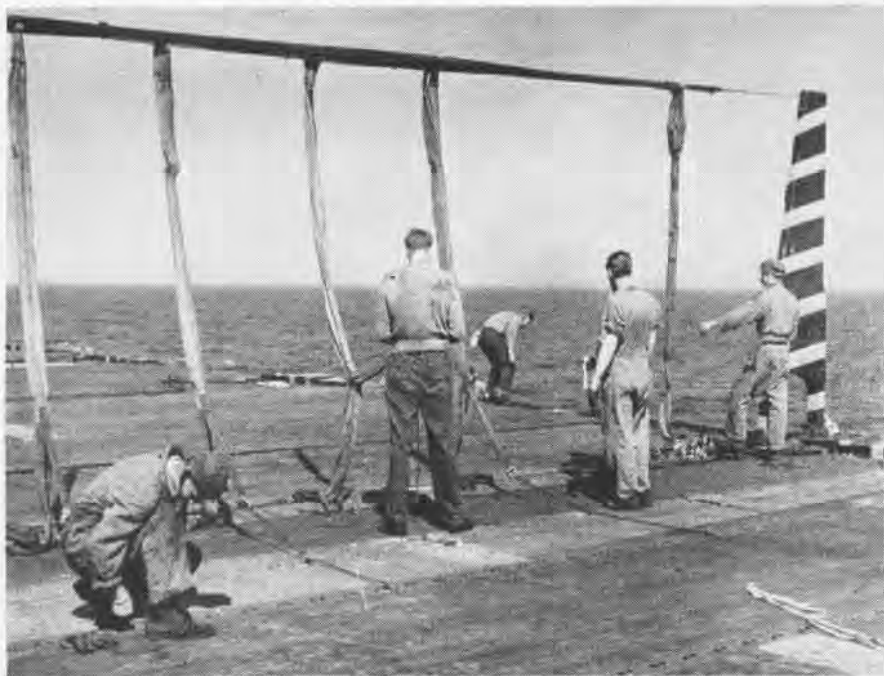
STOPPING a wild-running airplane which careens up a carrier deck without catching an arresting wire has long been a worry in naval aviation. Barriers did the trick for years until pointed-nose, tricycle landing geared jets came along. Then the Davis barrier was developed, arranged to raise the lower wire after the nose wheel had gone over it. To augment this barrier, a retardation barricade has been developed, employing long vertical risers of nylon to catch the plane's leading edge of the wing. Shown here is one of the barricades being rigged by flight deck crewmen aboard the USS Boxer , operating off Korea.
