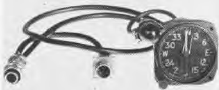
UNIT USED IN VA-45 COMPASS-SWING METHOD
