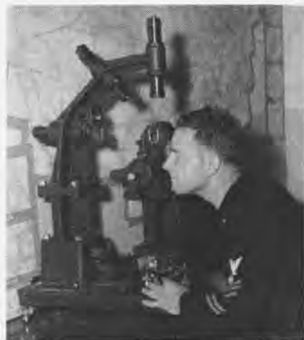
THIS GISMO is a collimator. A. L. Grover, QM01, of VR-3 is giving a sextant the eye
