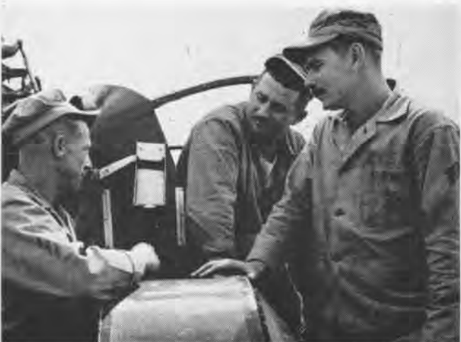
BRACKET on HTL fuselage holds blood plasma bottle during hop; Sgt. Fulcher, Capt McCluen, Sgt. Petruck developed the device
