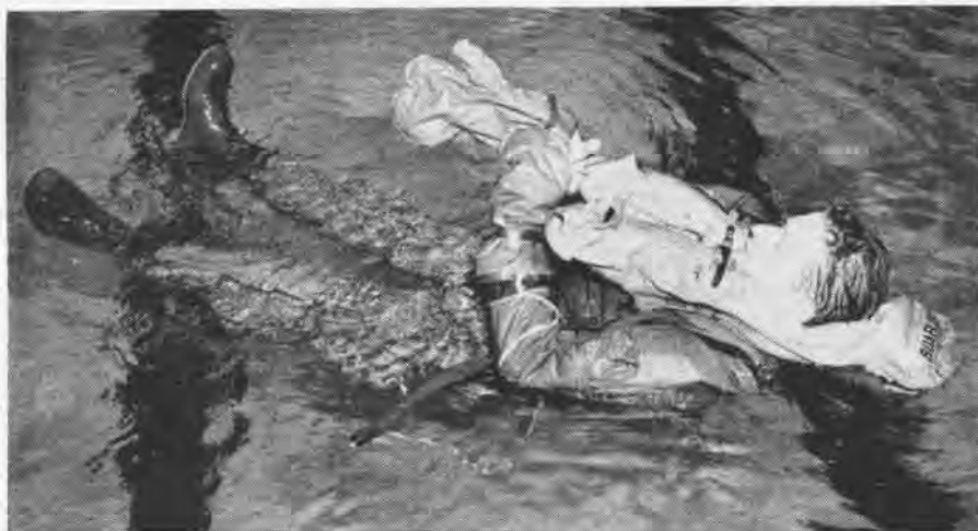
NEW MK 4 exposure suit showing excellent flotation qualities; pilot is putting on the quick-donning gloves; reports from fleet pilots were included in revised model
