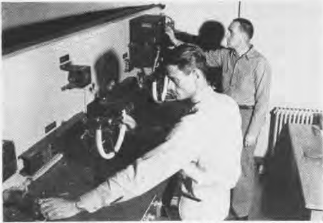
INSTRUCTORS L. E. Callahan, AO1, and Ralph C. Pemberton, ADC, demonstrate the switches to fire rockets on P2V-4 trainer
