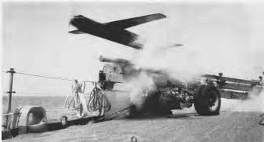
HERE IS SHOWN A DRONE TARGET WHICH IS LAUNCHED FROM USS HELENA, AIRBORNE AT 65 KNOTS
