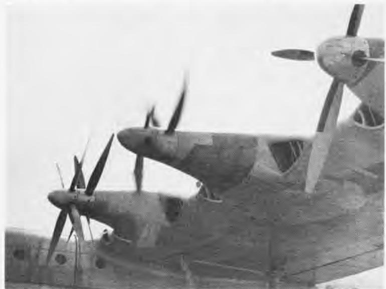
COUNTER-ROTATING 16½' PROPS CAN BE PITCHED THIN TO MAINTAIN THE RPM
