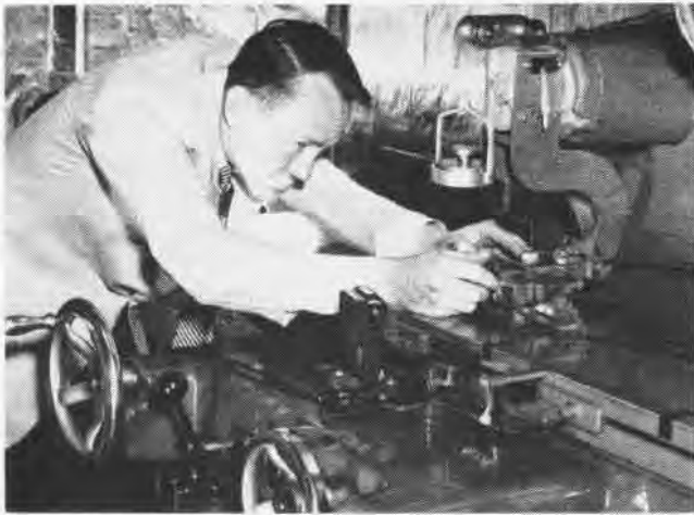
HOW LUBRICANTS work on various metal surfaces is tested by William Clinton in this NRL-designed "slip stick" test machine
