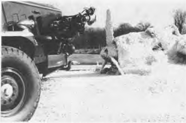
RESEARCH Lab scientists had large hand in developing crash fire fighting trucks which can lay heavy foam or water fog on planes
