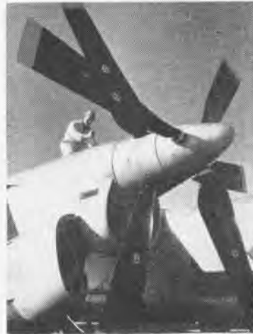
LONG SPINNER ON XA2J TURBOPROP JOB
