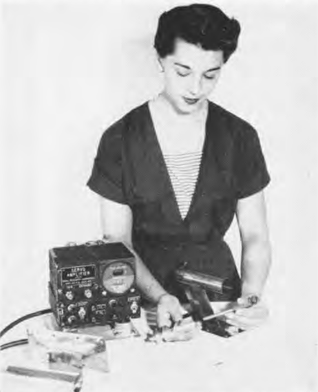
NEW VORTEX thermometer for weather recon planes is inspected by Nancy Monacelli; thermometer will be valuable in weather flying
