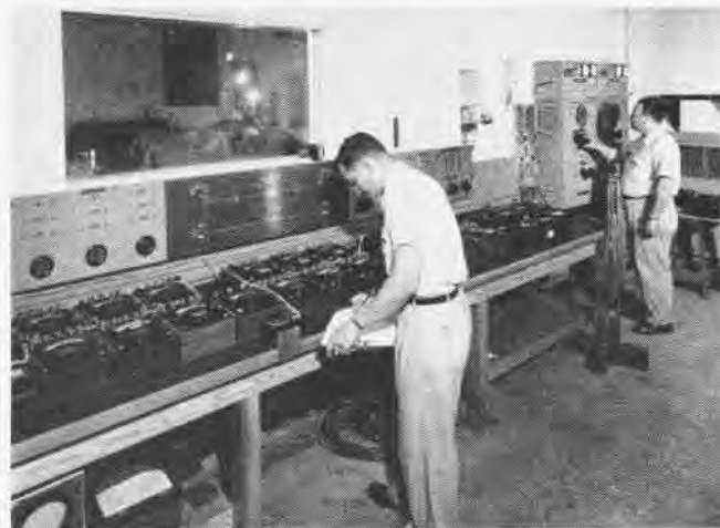
AIRCRAFT generators as large as 120 kva can be tested by Fred Yagerhoffer and David Weiner in this sound-proof control room
