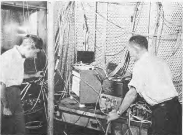
SEEING how flight equipment reacts at simulated 50,000-foot altitude is job of Joseph Marzolf and Edgar Quackenbush of Lab
