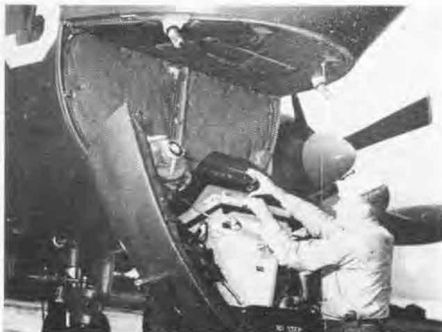
GILL UNLOADS CAMERA FROM CHIN MOUNT OF AN AJ-2P OF VJ-62
