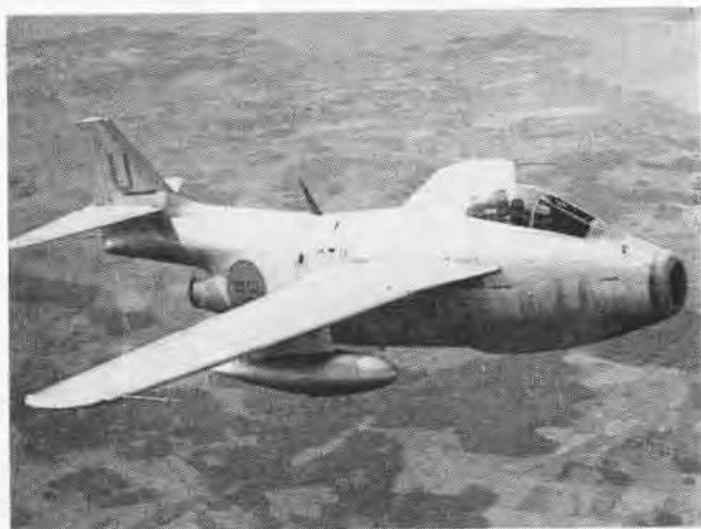
NEW SWEDISH SAAB S-29C JET PHOTO PLANE PACKS SIX CAMERAS
