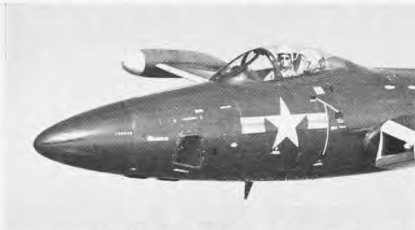
CAMERA BEHIND OPEN PORT IN F9F'S NOSE CAN BRING BACK INTELLIGENCE ABOUT ENEMY
