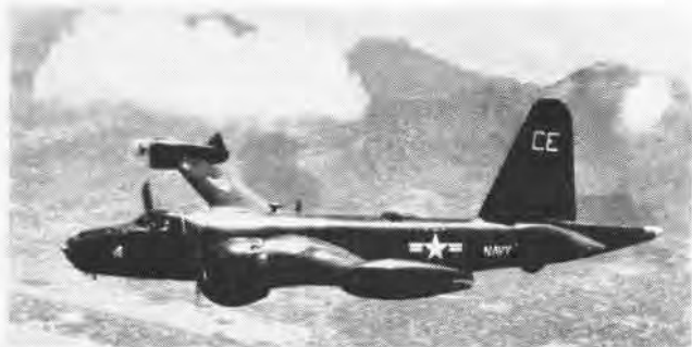
LONG TAIL BOOM OF VP-22 P2V CONTAINS GEAR TO LOCATE SUBS
