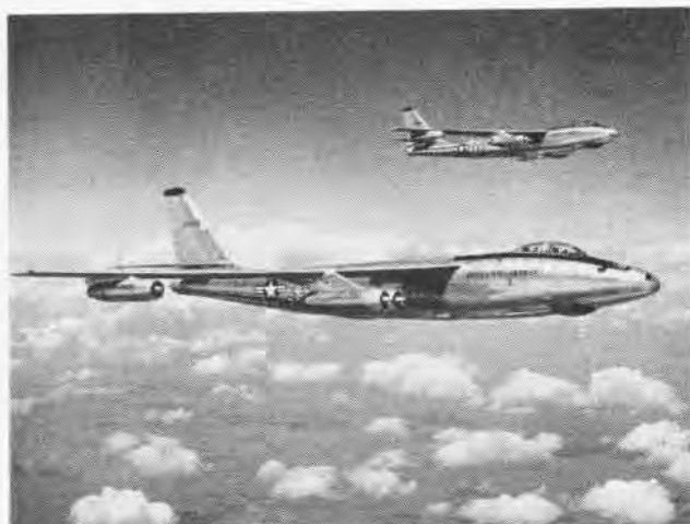
SLEEK BOEING RB-47E STRATOJET HAS CAMERAS IN ITS LONG NOSE
