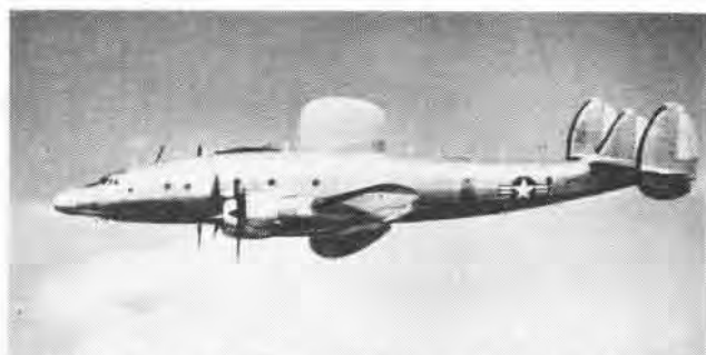
RADOMES TOP AND BOTTOM BREAK SLEEKNESS OF WV-1 ASW PLANE
