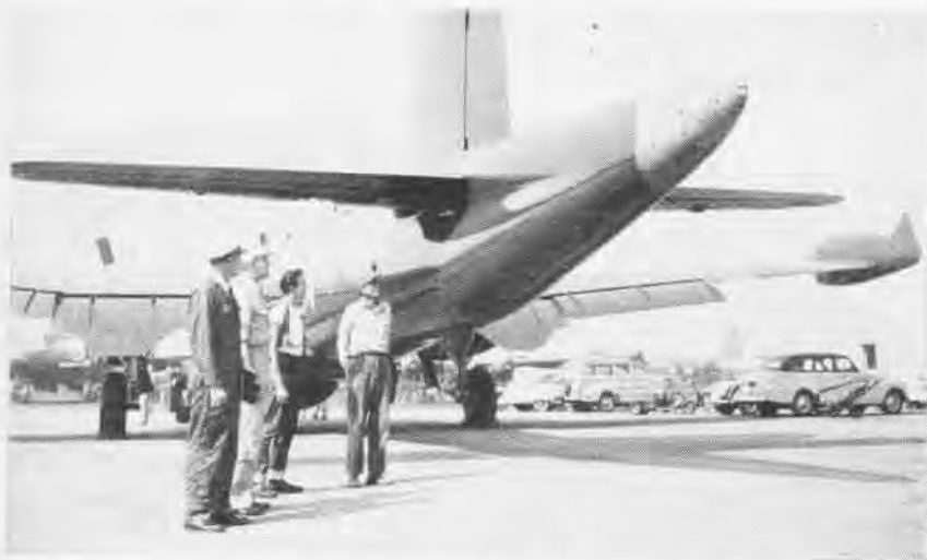
MANY experimental aircraft carry "stingers" on the nose to measure yaw, but the P2V is probably the first to pack a "stinger" on its tail. In this case, the long protuberance is full of electronic searching gear. Most Neptunes carry machine guns or 20 mm cannon in a tail turret. The fairing reportedly increases speed.
