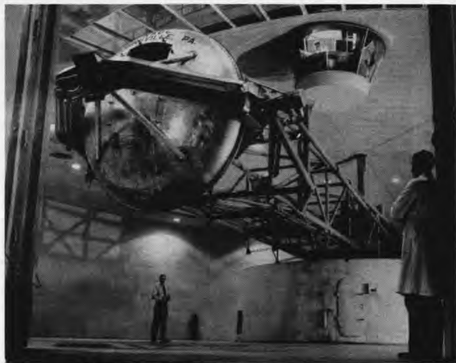
NEWLY-FINISHED human centrifuge at Johnsville whirls men in gondola to check on effects of high G forces on the human body; scientific instruments attached to man record data.
