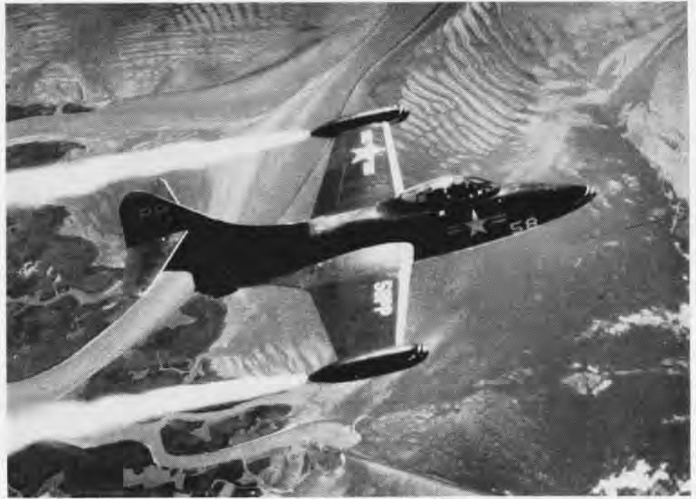
STREAM of gas flows from wing tanks as Lt. J. Harris, photo pilot of VC-61, releases fuel load over Tokyo Bay prior to landing F9F aboard carrier. Note mud flats, fish trap below the Panther's nose
