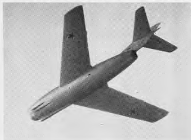
BELLY PICTURE OF FAMED MIG-15 SHOWS LOCATION OF 3 NOSE CANNON
