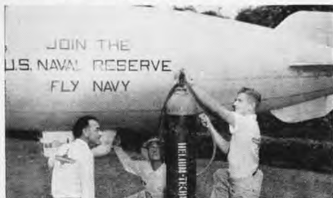
BUILDUP almost finished, the model builders are shown topping airship model with helium. Note recruiting slogans on side
