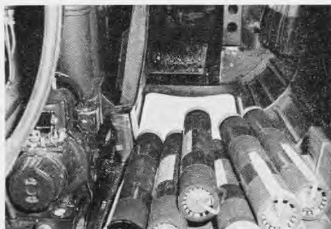
WHEN ACCESS DOOR IS CLOSED, FLARE CHUTE IS IN POSITION FOR USE
