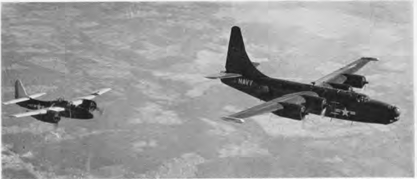
DRONE PRIVATEER WITH CAMERA PODS ON WINGTIPS FLIES UNDER F7F MOTHER PLANE CONTROL; NAVY WILL USE DRONE TO CHECK GUIDED MISSILES
