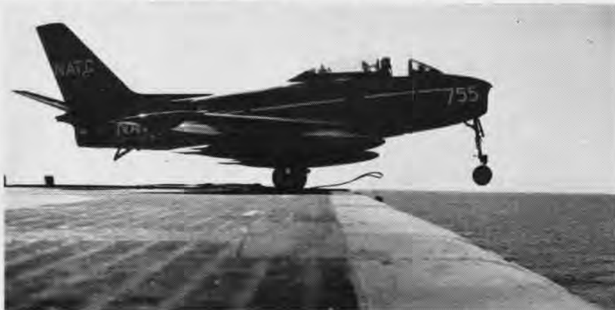
FURY jet is stopped by camera on tip of Coral Sea's flight deck near climax of catapult shot. The FJ-2 completed carquals in 1952, and is in production for fleet squadron use
