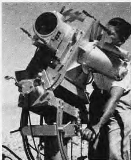
ACCELERATION camera used for tracking first 300 ft. of guided missile flights at Mugu
