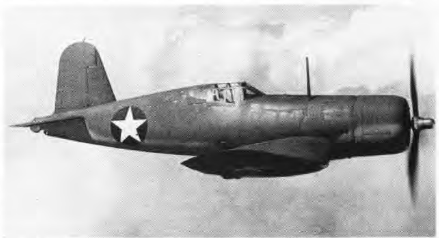
F4U-1 In the production model, the cockpit was shifted three feet aft to make room for fuselage fuel tanks. Low pilot's seat, long nose made for poor visibility
