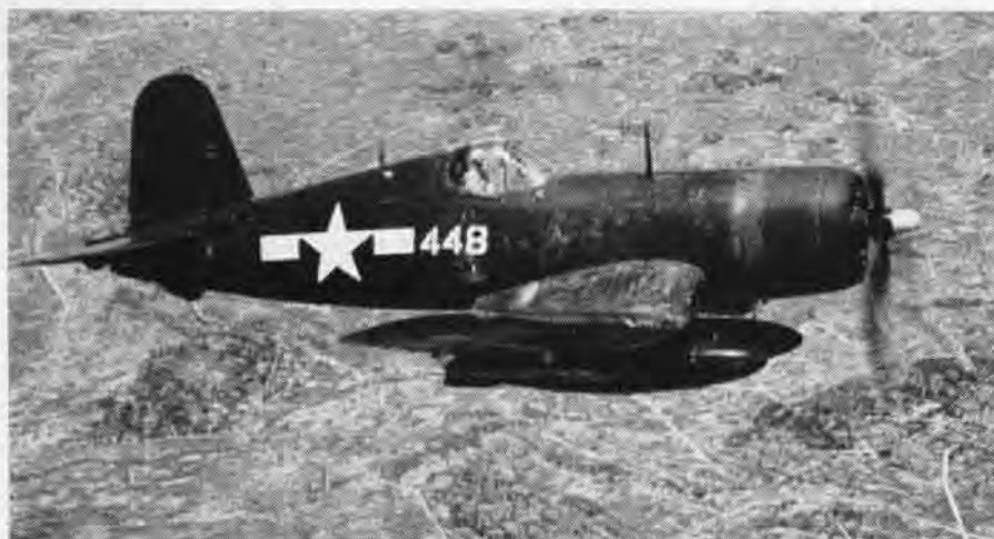
FG-10 Manufactured by Goodyear, this airplane along with F4U-1A and later Corsairs had raised pilot's seat and bubble canopy. Marine in picture is over Okinawa
