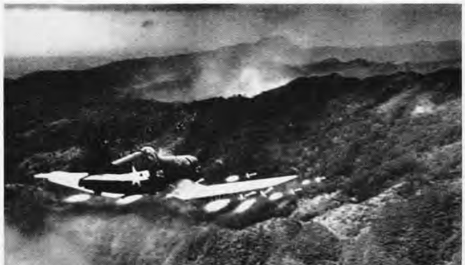
ON OKINAWA close-support mission, Marine F4U demonstrates ability at low-level work with blast of eight five-inch rockets directed at key Japanese ground installations
