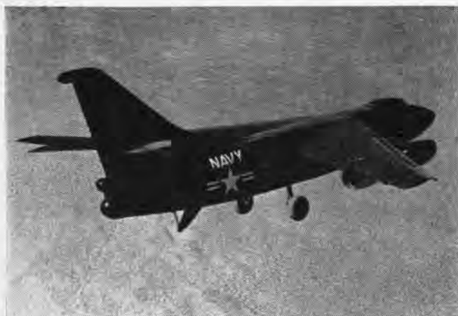
NAVY swept-wing jet attack bomber, the XA3D, is one of latest and largest carrier aircraft. It carries a three man crew
