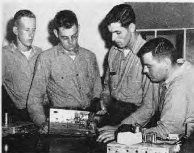
INSTRUCTOR, W. A. Miller, demonstrates use of soldering gun to Hall, Mitchell and Magnani as he installs the "on-off" switch
