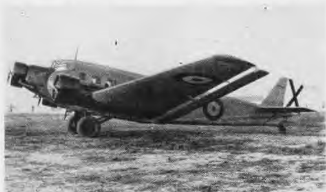
THREE-engined JU-52 transport, borrowed from Germans, got its combat tests during Spanish civil war, flying with Franco units
