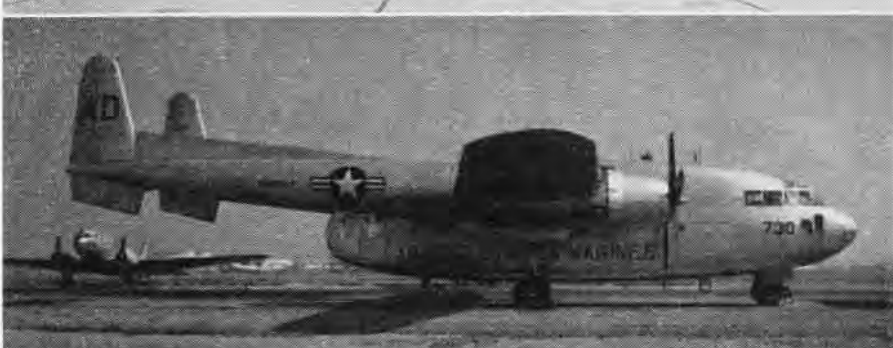
NEW PICTURES of two new Navy and Marine planes, shown here for recognition students, were taken at a recent air show on the West Coast. The top two are the XA2J-1. This big carrier-based plane is powered by two T-40 turboprop engines and counter-rotating propellers. Note the folding tail for hangar deck stowage. The lower plane is the Fairchild R4Q-1 with modified tail, flown by VMR-253. The Packet has elongated fairing on the top of the tail boom and an unusual-shaped projection below the vertical stabilizer. Early models of the R4Q had a semicircular appendage below the boom and later models came out with this eliminated. Tubes on XA2J wings are for scientific measurements in flight.
