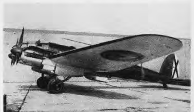
CASA-2111, Spanish version of the feared Heinkel-111 light bomber, was another German fighting plane used by the Francoites
