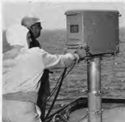
TRODI in use aboard carrier for accurate determination of aircraft rates of descent
