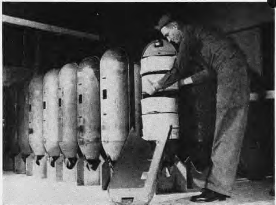
ROLLS OF THOUSANDS OF PSYCHOLOGICAL WARFARE PAMPHLETS ARE LOADED IN MK 105 BOMB CASE
