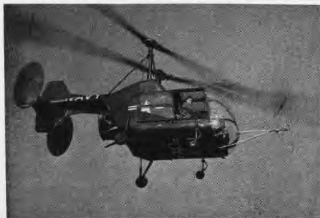
HTK-1 DOUBLE-rotored helicopter built by Kaman presents novel appearance as it flies in BIS trials at NATC Patuxent River
