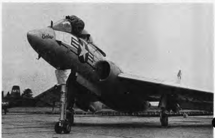
CONTESTANT for the "fastest jet" in the Navy's fighter stable is this F7U-3, which passed preliminary carrier suitability BIS trials of the Coral Sea and is now getting remaining tests
