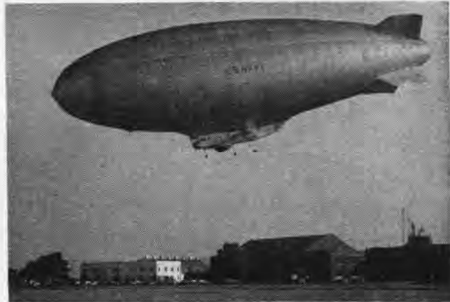
LATEST thing in airships is the ZPN-1 Nan ship which was tested at Lakehurst and got its ASW tactical trials with FAETULant
