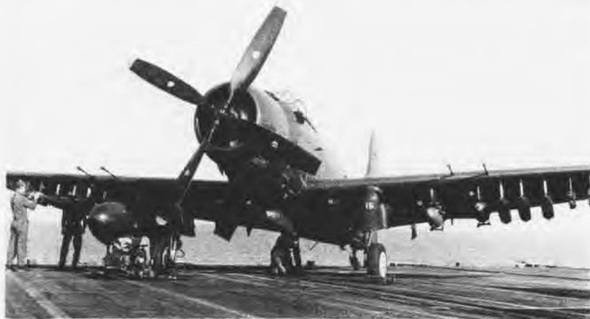
VC-35 GAVE the "Mighty Mouse" 275 folding-fin rocket pods a tryout in Korea and found them effective; this AD-4N carries three bombs, four flares and six of pods.
