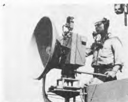
MICROWAVE ANTENNA TRACKS INCOMING JET
