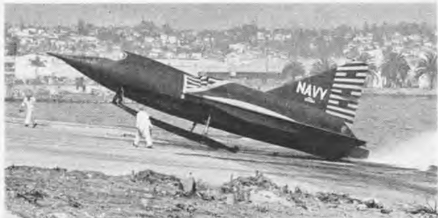
NEWEST photo of the Navy-Convair XF-2Y-1 Sea Dart is this one showing it taxiing out of the water at San Diego on its small hydroski and tail wheels. The plane was given its first public showing recently. Hydroskis enable the delta-wing plane to taxi and break away from the water until takeoff speed is reached. Two J-33 jets with intakes located just aft of the striped area amidships drive the new seaplane.
