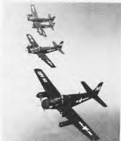
SEARCHLIGHT and radar load the AD-4N's of VC-35, used to hunt out enemy trucks.
