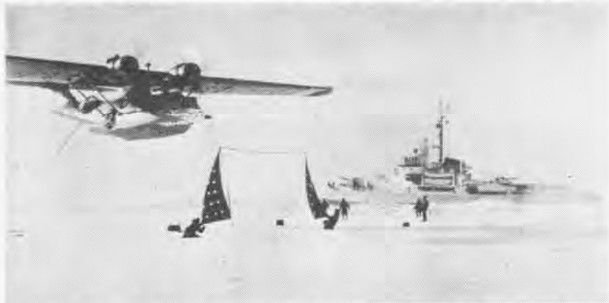
MAIL PICKUP CABLE OF NYLON SUSPENDED BETWEEN TWO UPRIGHTS AS PB-4Y MAKES PICKUP
