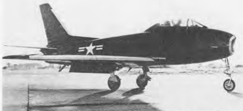
POWERED by a Curtiss-Wright built J-65 Sapphire jet engine, the latest of the line of the Navy's FJ-1 Fury is the new FJ-3 fighter by North American. The 7500-pound thrust axial flow jet replaces the J-47 which has powered the FJ-2 and F-86, with 6,000 pounds thrust. With all this extra power, the FJ-3 is expected to be considerably faster than the earlier versions, which have been flown over 700 mph. The J-65 is the American version of the Sapphire, designed and built by Armstrong Siddeley in England. It also is in the F-84F. Since the engine is larger, the plane's size also was increased slightly.
