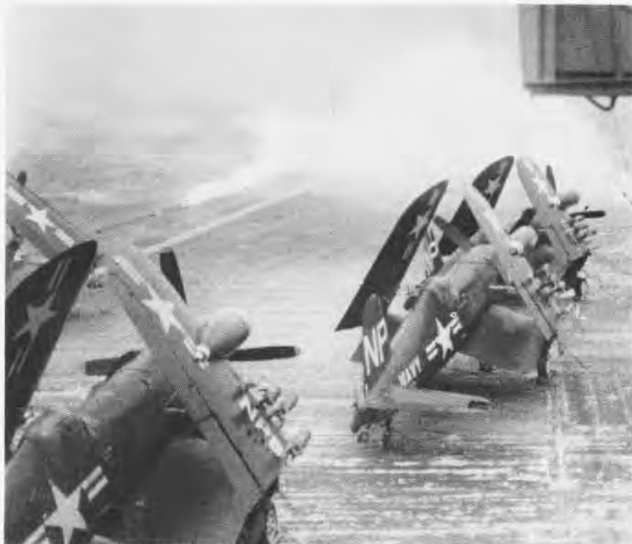
SALT WATER SPRAY DRENCHING CARRIER DECK WOULD PLAY HOB WITH ANY UNPAINTED PLANES
