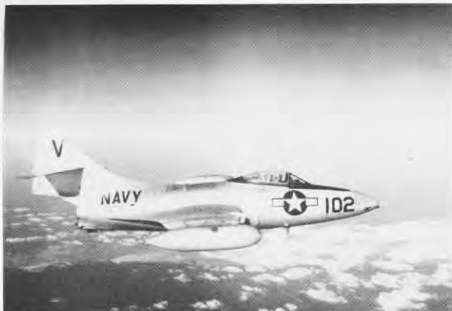
UNPAINTED F2F PANTHER FROM THE BOXER OFF KOREA TESTS BUER NO-PAINT IDEA IN WAR
