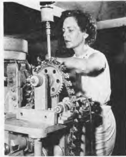
NOTCH painting machine paints silver conductor metal on wafers made in the plant
