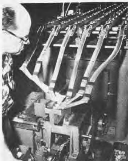
CERAMIC wafers are assembled and soldered into modules under eye of worker at plant
