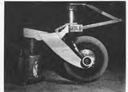
A TAIL wheel jack pad for HUP helicopters has been successfully manufactured by HU-1, Seaplane Base, Key West, Fla. Full details of how the pad was made from scrap material can be obtained by writing the squadron, HS-1.
