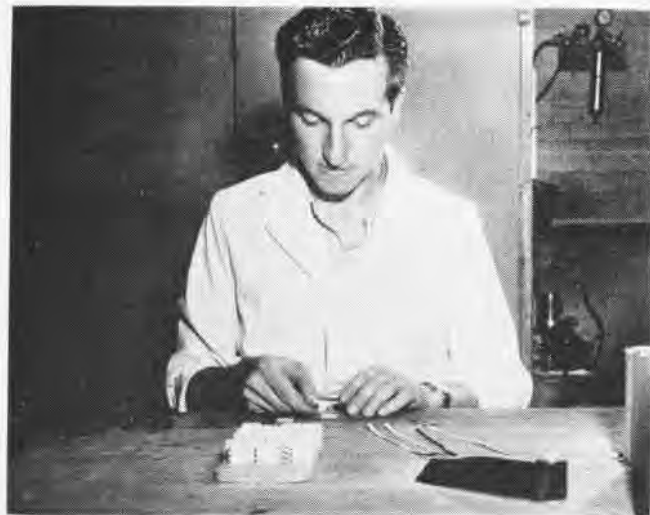
RESISTOR tape is applied to module wafer as a pre-test to evaluate its resistance, correct width before going into assembly
