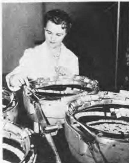
VIBRATOR machines sort wafers which are used to make up modules, a basic component
