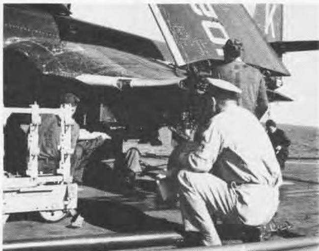
ORDNANCMEN of CAG-3 attach a 5" HVAR rocket under wing of Banshee while ComFair Jacksonville inspector approves how it's done
