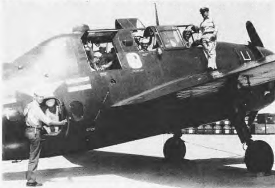
FULL LOAD of seven men and 2,000 pounds of gear in converted TBM-3R torpedo bomber bomb bay ready for takeoff as Chief L. M. Bailey checks pilot to see if he is ready
