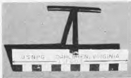
SIMPLE 'T' WRENCH GETS AT BOLTS ON BOMBS
