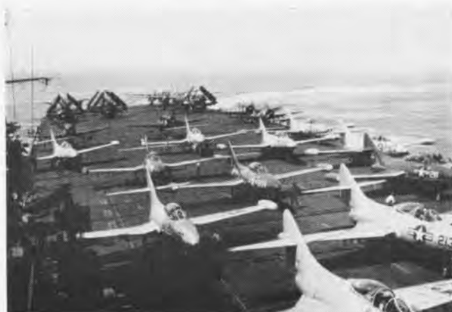
BARE AND PAINTED F9F'S ON FDR'S DECK TEST NO-PAINTING THEORY
