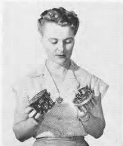
OLD SONOBUOY component (right) shows the complex wiring eliminated in new (left)
