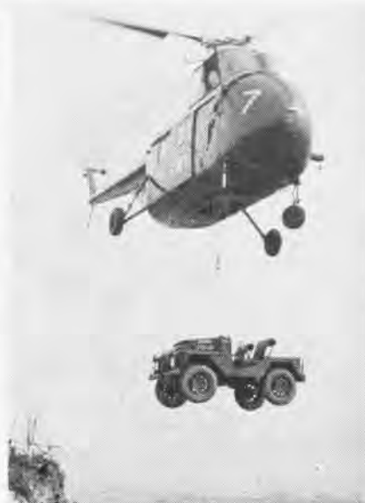
SUCCESSOR to the famed "Jeep" of WWII days is this "Mighty Mite", a 1500-pound vehicle which can be picked up by helicopter. MCAS Quantico demonstrated the car to the public with various combat equipment on it, including a 105 mm recoilless rifle, wire-laying gear, a 4.2" mortar and an ambulance rig. It is 1,000 pounds lighter than the older model jeep.
