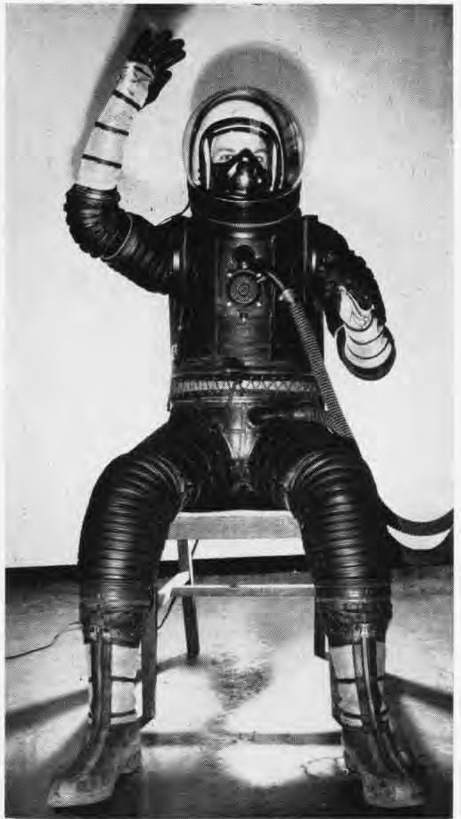
HEAD-ON view of pressure suit which permits pilot to move so he can fly plane and still be safe if cabin is depressurized
