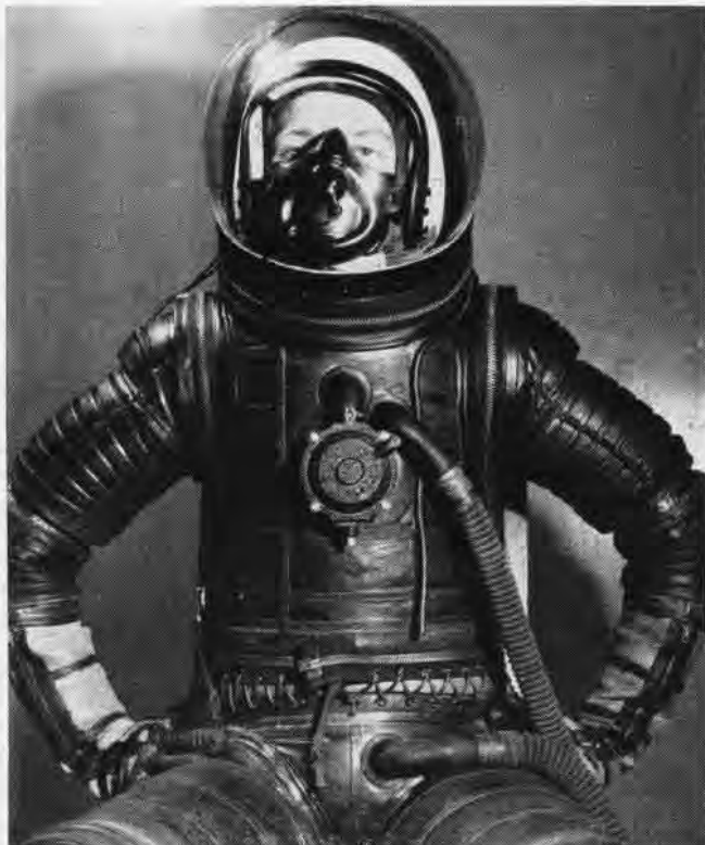
PILOT models the Navy's full pressure flying suit in low-pressure altitude chamber. Note the zipper fastening the 'fishbowl'
