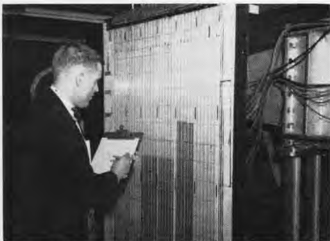
LT. JOHN F. Wester is carefully taking down initial manometer readings prior to commencing a test in transonic wind tunnel.
