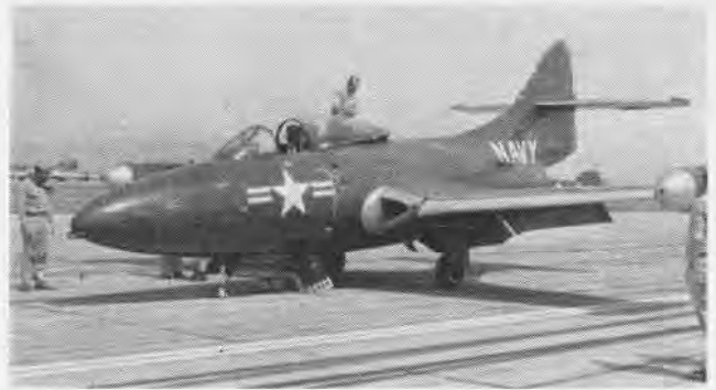
THE NOSE wheel on this Panther fell off because of a mechanic's error. Good organization, supervision and morale help check this.
