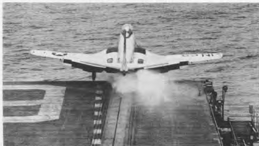
A BANSHEE becomes the first American jet aircraft to be launched by steam catapult from the deck of a U. S. carrier. Ltjg. William T. Brooks piloted the plane on take-off from the Hancock during operations off the Southern California coast. He was also co-pilot for Cdr. H. S. Jackson when their S2F-1 submarine hunter-killer plane was launched by the new system earlier.
