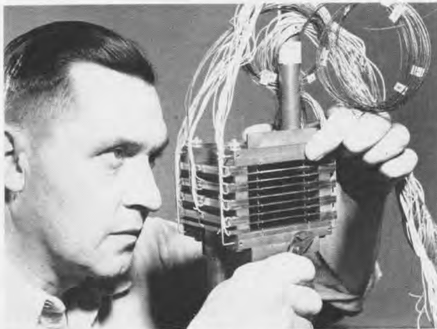
THE MULTIPLE sandwich being adjusted is one of many devices being used to furnish basic data required in designing heat exchangers. Information obtained is useful in designing reactors.
