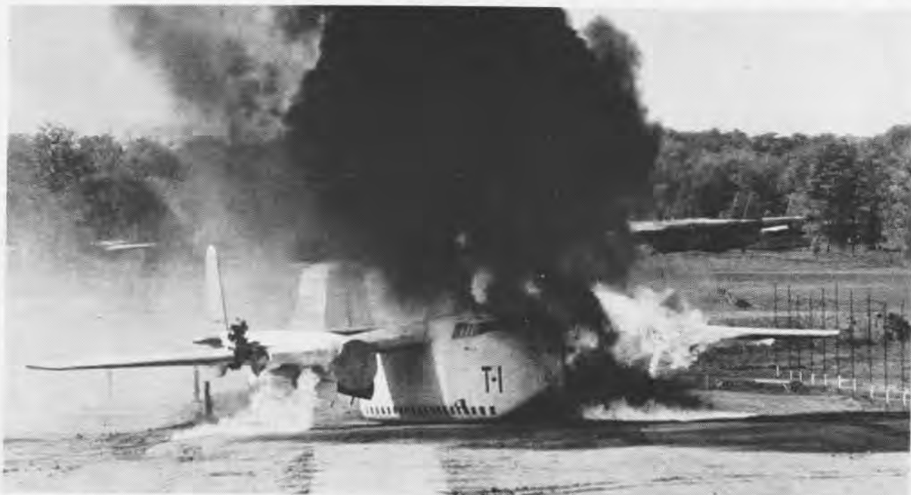
SERVICE-WEARY 0-02 on which reciprocating engines were replaced by pylon-mounted turbojet units is used in experimental crash fire research program. Right engine had a crash-impact released stream of water thrown over the hot tail surfaces at end of launching track.
