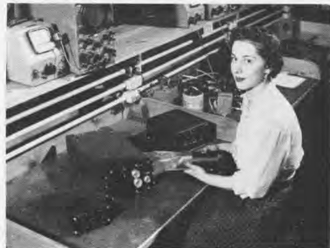
GIRL wraps units in moisture-proof bags before final packaging and shipping. Four units are computer control, amplifier, indicator, computer.
