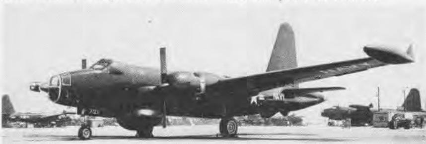
FIRST of a new series of v2v Neptunes to be delivered to the fleet is this v2v-7, No. 7001. Production models of this new submarine killer will mount twin jet pods plus two turbo-compound piston engines to provide bursts of speed over the target and during take-off. Crew members can change the v2v-7 from its principal role of sub hunting to that of minelaying or torpedo-bombing on demand. Secret electronic gear in the stinger tail and radomes define search areas of plane.
