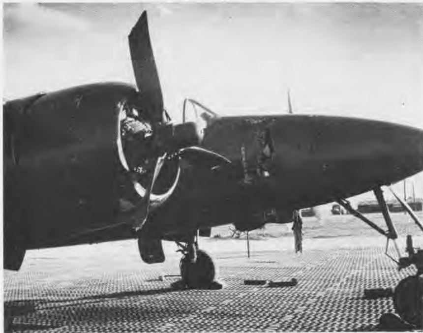
LOOK WHAT happened when someone didn't reconnect cockpit throttle and mixture controls after complying with F7F T. O. On taxiup, engine went to full power. Plane jumped chocks.
