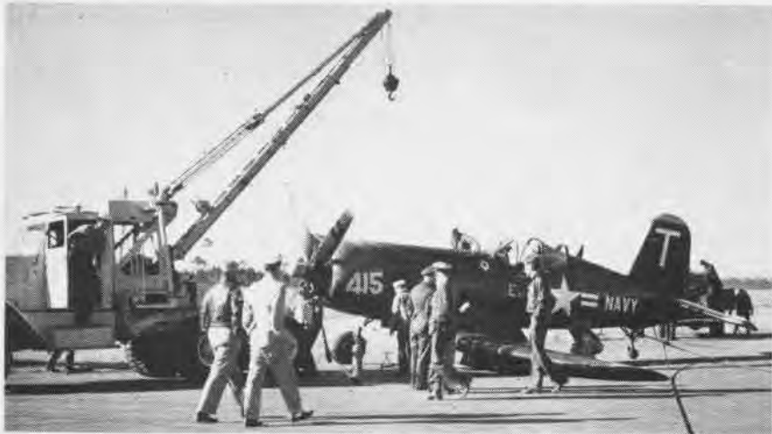
SPOILER AND his cousins in the maintenance crew reversed the up and down hydraulic lines on the port gear of Corsair. When port gear was down and locked, starboard was up and locked.
