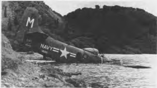
LACK OF a cotter pin caused throttle of this AD to disengage in flight. With no power available, pilot ditched, lost Skyraider.
