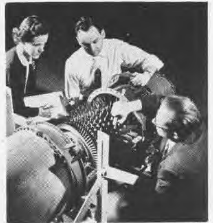
INSPECTING an experimental jet engine axial flow compressor prior to making speed run.
