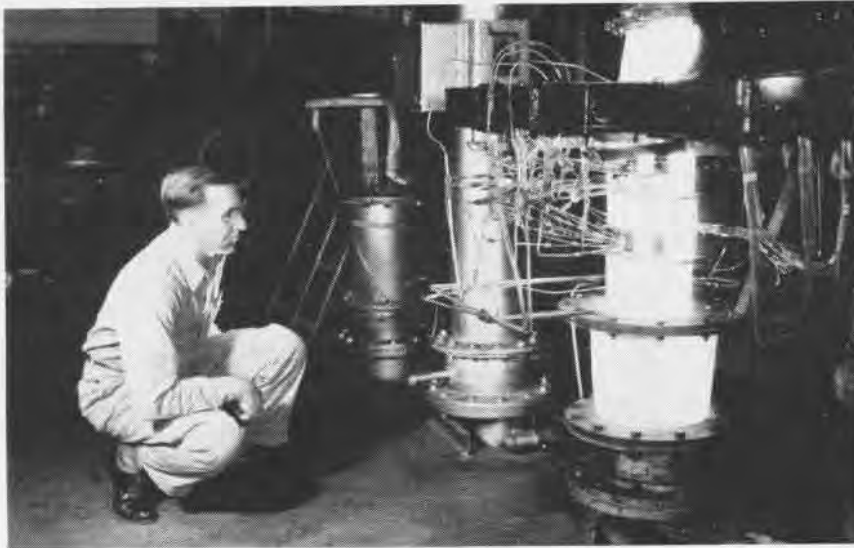
HIGH TEMPERATURE problems are studied by isolating a hot instrumented exhaust section. At temperatures between 1500 and 1600 degrees F, data is gathered on ignition and combustion.
