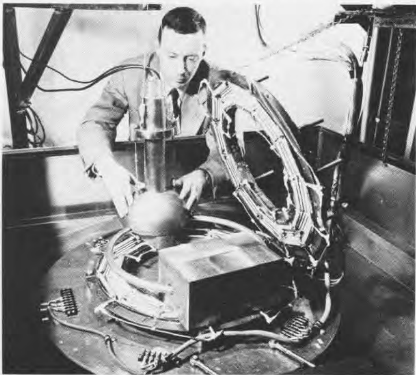
METAL DOUGHNUT is used to carry out corrosion research. Heating elements and thermocouples furnish high temperatures. Coolants and mass transfer of materials is an urgent nuclear problem.
