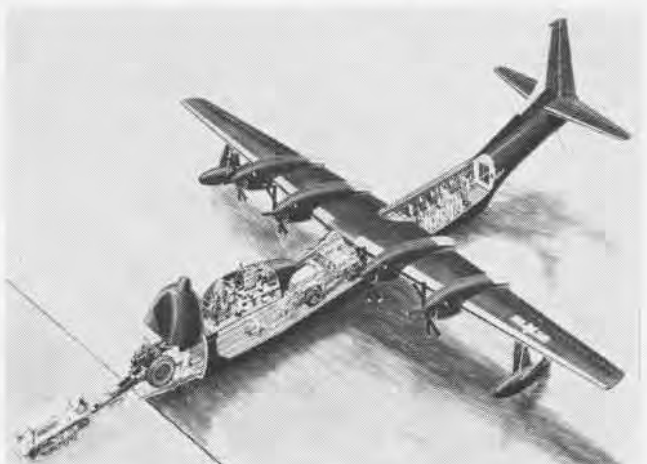
CUTAWAY drawing of the NAV-2 shows bow-loading ramp, full length cargo deck and elevated bridge. It will go into service at Alameda.
