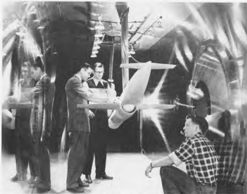
RAMJET missile model is seen mounted in 8x6 foot supersonic wind tunnel. It is used for tests simulating flight at 50,000 feet at speeds up to 1300 mph. Numerous configurations are tested.
