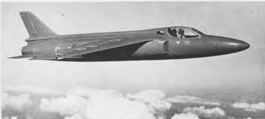
THOUGH essentially similar in design to the Gnat light fighter, the Midge is merely a prototype, intended to try out characteristics of that type pending availability of Orpheus turbojet
