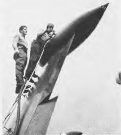
WING TANKS EXTEND JETS COMBAT RANGE
