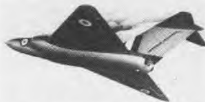
POWERED by two Sapphire turbojets, Gloster Javelin is built for high altitude flight.
