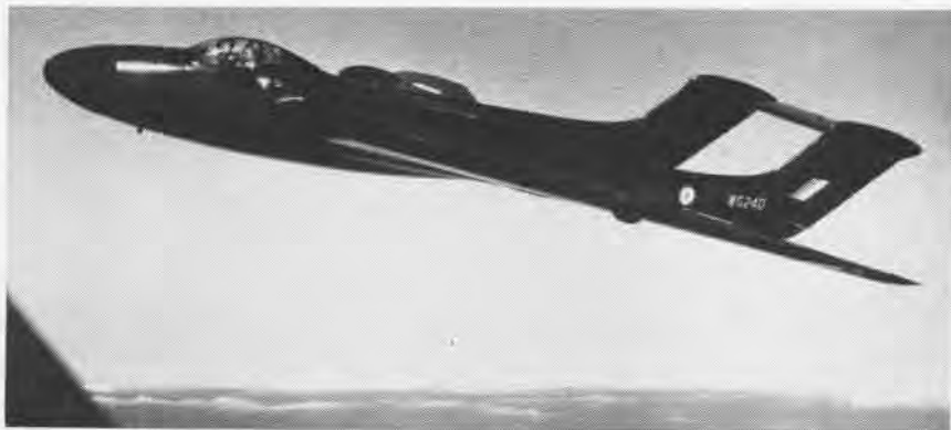
ORIGINALLY designed for shore-based service, this supersonic, twin-jet, all-weather day and night fighter, the D.H. 110, is being developed as a replacement for the carrier-borne Sea Venom .
