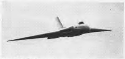
VULCAN is due to be powered by four Olympus turbojet engines. It flies at 50,000 feet.
