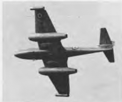
SILHOUETTE of Meteor in flight demonstrates wing tip installation of Soar jet engines.
