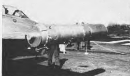
SOAR on Meteor wing tip is a small simple turbojet with big output of 1,810 lbs. thrust.
