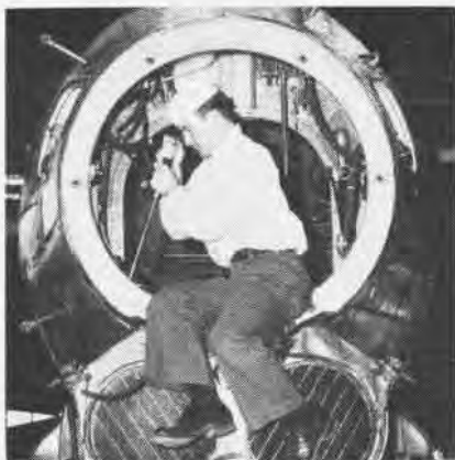
BOTH feet in his work, Norfolk airman Laurie prepares an engine mount for VP-861's P2V-3.
