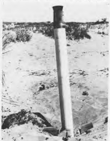
AFTERBODY of the rocket lies partially buried in the desert sand after the firing.
