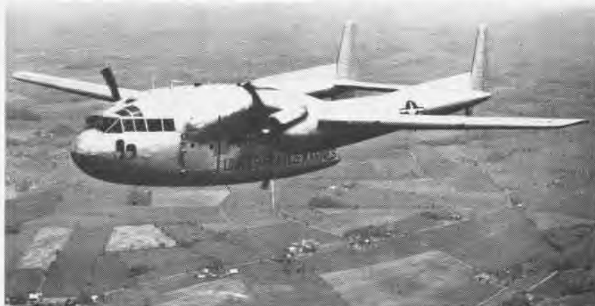
THE TWIN tail booms of the R4Q "Workhorse" make recognition relatively simple. This airplane is used by Marine aviation squadrons to provide air support to Marine Corps ground forces.
