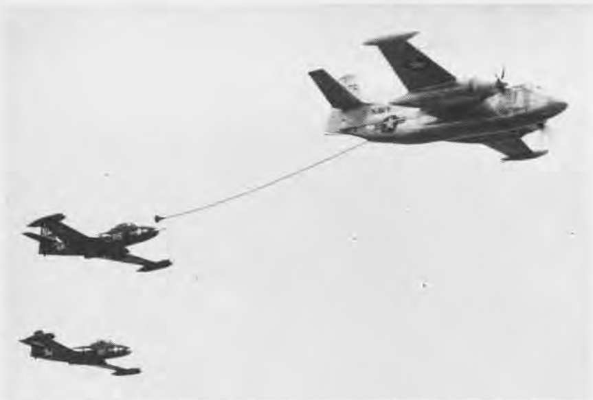
A NAVY AJ SAVAGE DEMONSTRATES PROBE AND DROGUE SYSTEM OF INFLIGHT FUELING
