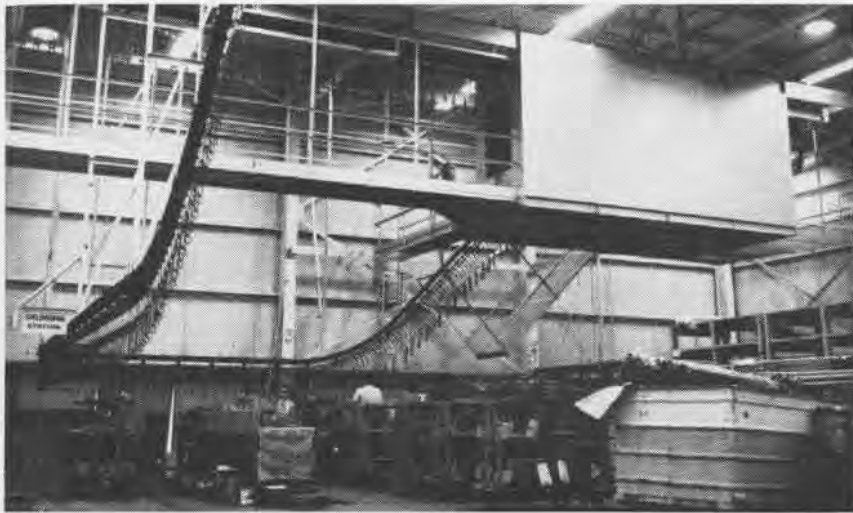
PAINTED PARTS FOR SKYRAY ENTER OVERHEAD DRYING OVEN, THEN GO TO INSPECTION
