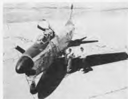
BOASTING a fuselage which is eight inches longer than her five predecessors, the Air Force's new F-86K is readied for flight. Packing four 20 mm cannons, sixth of the Sabrejet series is an all-weather fighter.
