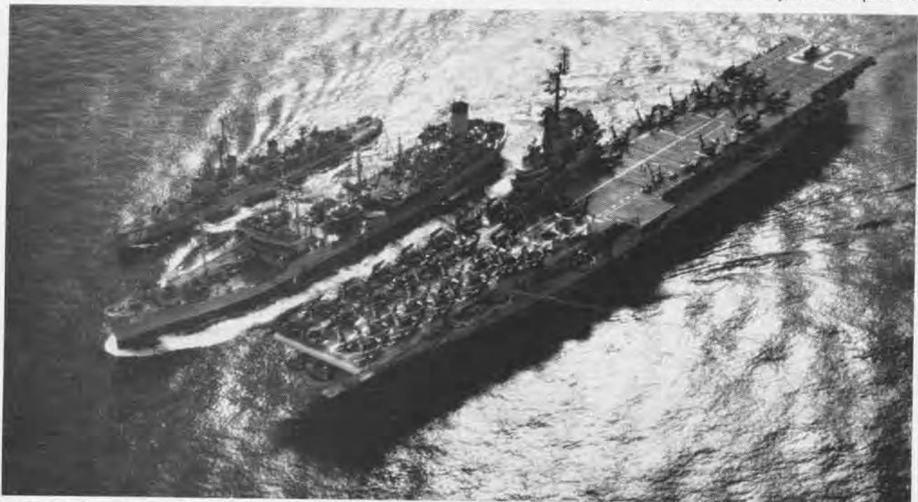
BECAUSE OF THE HIGH FUEL CONSUMPTION RATE OF JET AIRCRAFT, THE OPERATING CARRIER MEETS THE TANKER REGULARLY
