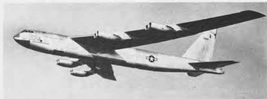
BOEING has unveiled the first production model of the Air Force's new B-52A Stratofortress. Powered by eight J-57 turbojet engines of 10,000 pounds thrust each, the huge bomber has a gross weight of 350,000 pounds. The B-52A differs from the two prototypes in that the cockpit arrangement has been changed to place the pilot and co-pilot in a side-by-side position.
