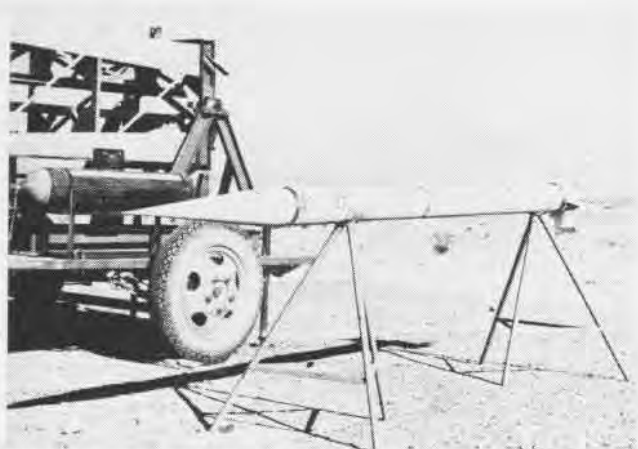
THE LONG cone-shaped nose of this 13½-foot rocket holds the new parachute, which is under test at White Sands Proving Grounds.
