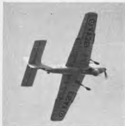
SEAMEW , a light, carrier-borne, ASW fighter, is powered by turboprop, has a crew of two.
