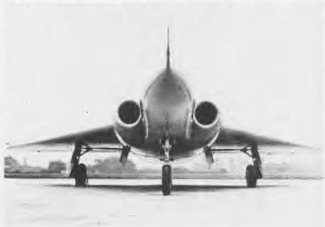
SUPERMARINE 525 , which passed through sonic barrier in a dive, represents interim development of supersonic fighter for Royal Navy.
