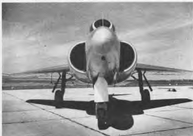
NOSE VIEW of Gloster Javelin delta-wing fighter looks like tail view because of nose spear used to gather data on test flights.
