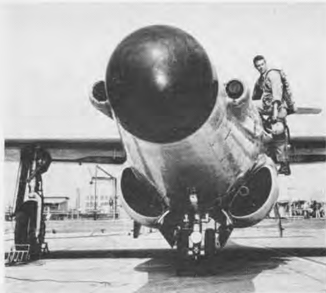
THE LATEST in automatic rocket launchers is modeled by this bulb-nosed F-89 Scorpion as it is readied for a test rocket firing run with Northrup test pilot Lew Nelson at the controls. Tabbled the
