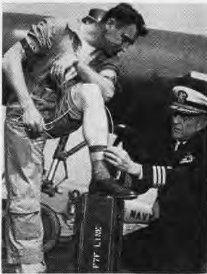
ELECTRODES are attached to Chief Kube's leg. Reactions are read on the ground.
