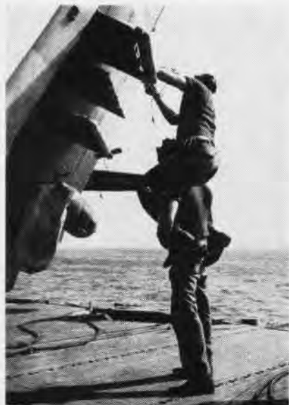
THE LAD on the bottom didn't lose a Rose Bowl bet. Two ordnancemen are using the "piggy-back" method to load small target rockets on the wing of a jet fighter aboard Yorktown on maneuvers with TF-77.
