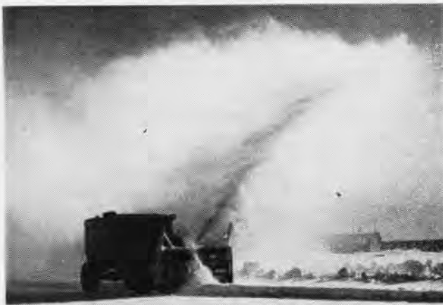
CONCRETE runways can be hastily cleared by busy snow plows. On ice-based fields, the snow is rolled flat and is left to cure.
