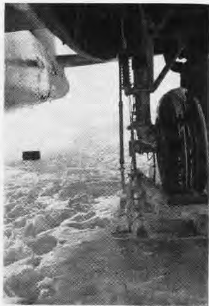
SKI EQUIPMENT , as shown here, makes aircraft maneuverable on Arctic snow fields.
