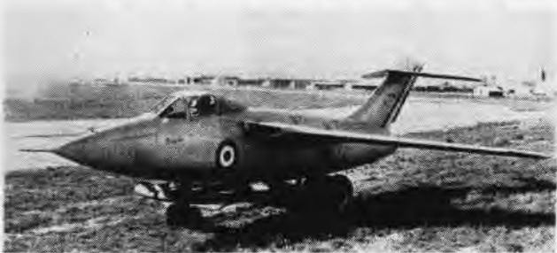
THIS VIEW OF 'BAROUEUR' SHOWS WAY IT IS MOUNTED ON TROLLEY
