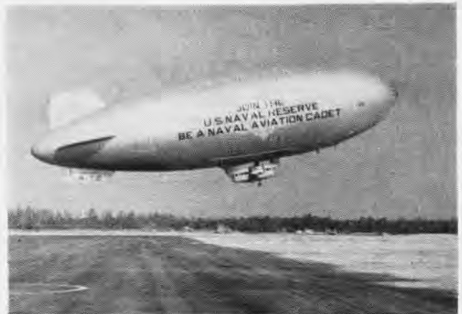
WITH AIRSHIP UNDOCKED, BUOYANCY OF LIFTING GAS TAKES IT ALOFT
