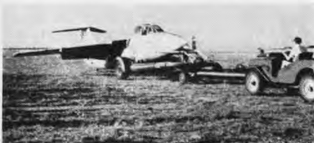
'BAROUEUR' IS PULLED ONTO TROLLEY BY MODIFIED JEEP IN FRANCE
