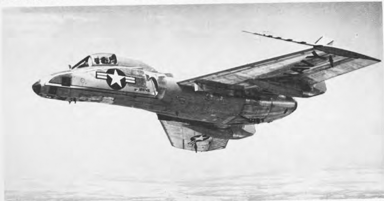
NEW CUTLASS, F7U-3P, PACKS FIVE CAMERAS IN NOSE, FLARES REPLACE THE GUNS.
