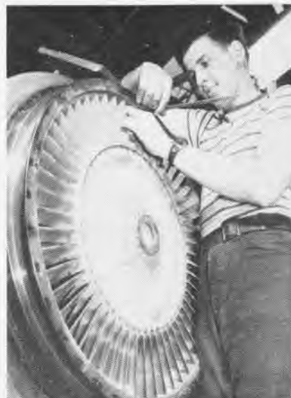
TURBINE WHEEL IS CHECKED WITH GAUGE
