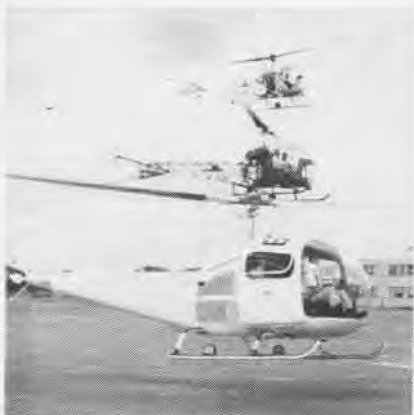
BELL experimental model 47G-1 (bottom) has the unique feature of being able to fly backward at 20 mph. Center is an Army H-13 and at top is standard demonstration 47 G-1.
