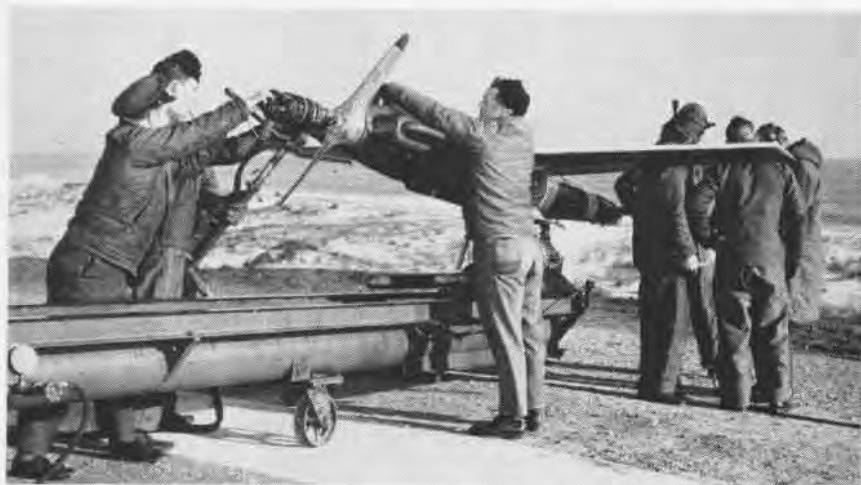
UTILIZING compressed air, crew members of VU-6 start the "bird" for its flight while other members check the radio control unit in the background. "Birds" fly for 90 minutes at 200 mph.
