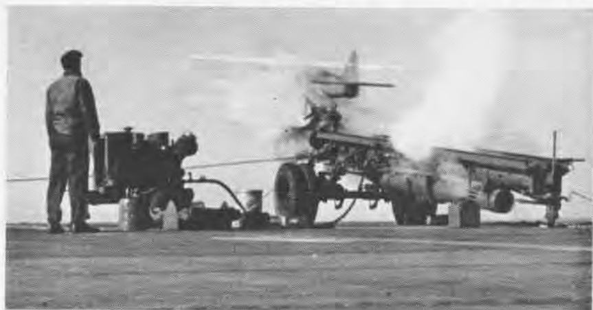
OFF goes the "bird" to be picked up and controlled by a remote unit aboard a carrier. The drone traverses the length of the mobile catapult in less than a second from the time of firing.
