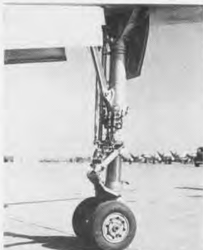
STEERABLE WHEEL CUTS HANDLING TIME
