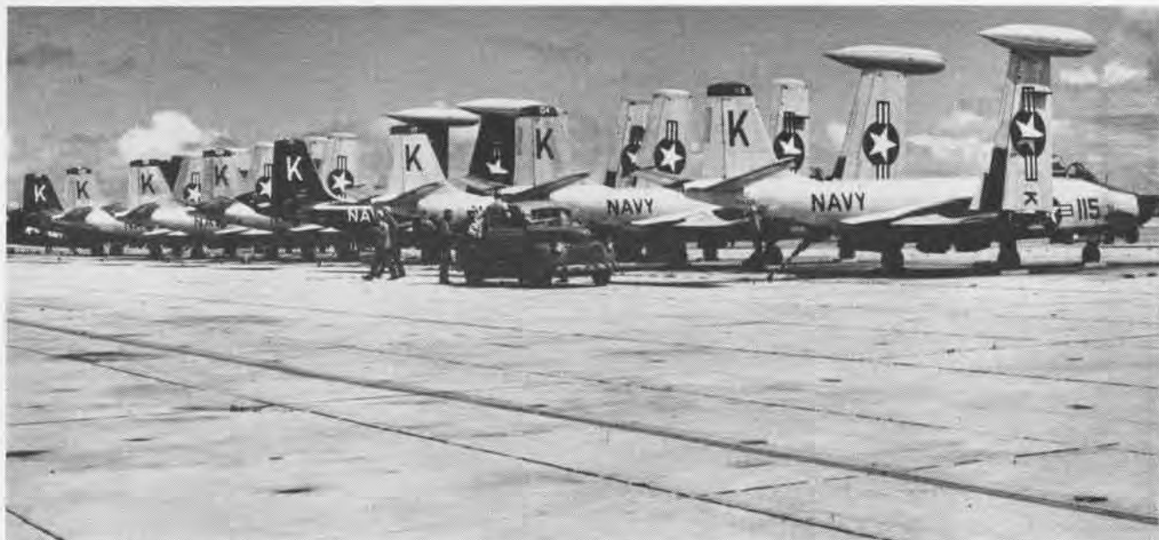
PARKING RAMPS MUST BE KEPT CLEAN, FREE OF DEBRIS WHICH MAY ENTER INTAKE OF ENGINES AND CAUSE EXTENSIVE DAMAGE
