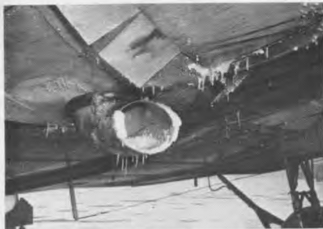
ICE ON AIRSCOOP INDICATES HEAVY ACCUMULATION ON WINGS PREPARING FOR EARLY MORNING TAKEOFF AT FALLON, NEVADA
