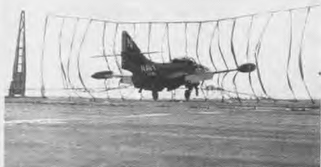
NEW 21 FOOT NYLON BARRICADE STOPS RUNAWAY JET ON HORNET
