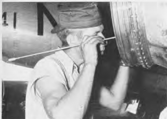
BURNER basket and turbine blades are given a 60 hour "B" check by J. R. Newbold, AD2. Engine is Westinghouse J34-WE34 from F9F.
