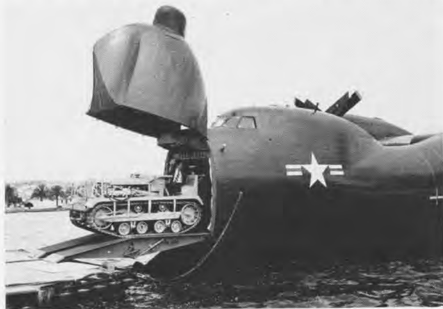
THE BOW of Convair's 80-ton RAY-2 "Flying LST" opens its huge jaws to receive a small tractor during a recent demonstration of its capabilities at San Diego. The turboprop TRADEWIND has been especially designed to put men and vehicles directly ashore during amphibious maneuvers.
