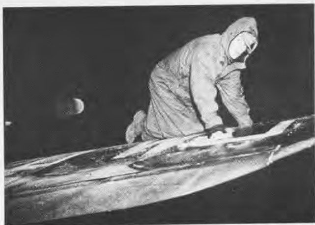
ICE ON AIRSCOOP INDICATES HEAVY ACCUMULATION ON WINGS PREPARING FOR EARLY MORNING TAKEOFF AT FALLON, NEVADA
