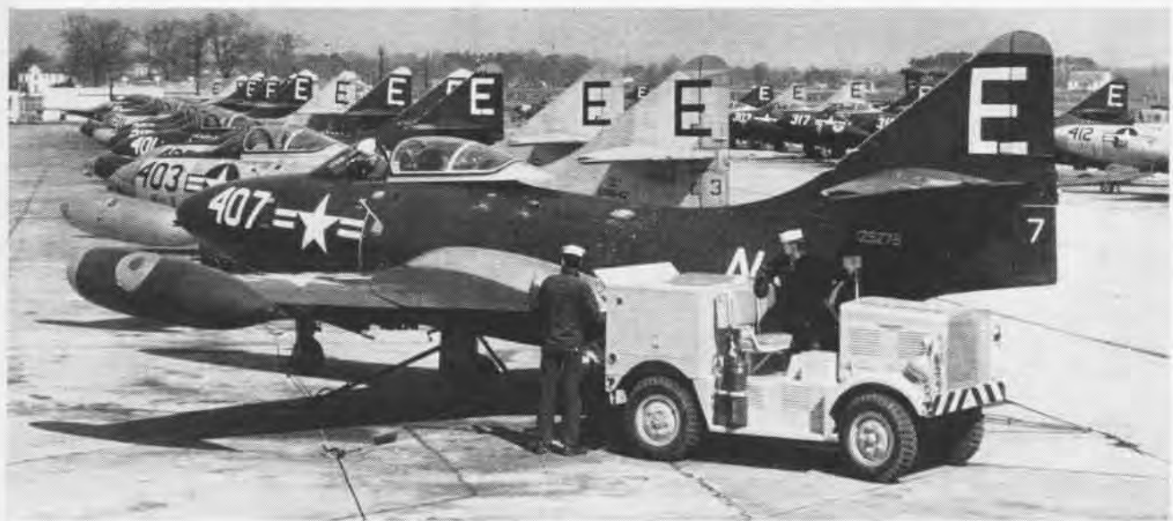
FASRON-5 personnel use new jet starter preparatory to turning up a Panther aircraft for engine test. Servicing, maintaining and making
