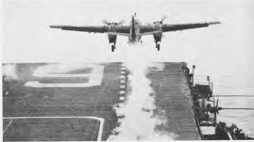
DOTS OUTLINE DECK LIGHTS ON CVA-59 STEAM CATAPULT IS MAJOR FEATURE OF CVA-59. USS HANCOCK LAUNCHES GRUMMAN 52F
