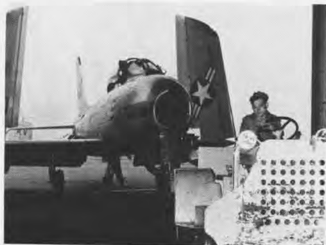
WINGS folded, Fury is towed to VMF-235 hangar for a periodic engine check. Maintenance personnel schooled at company plant for FJ-
