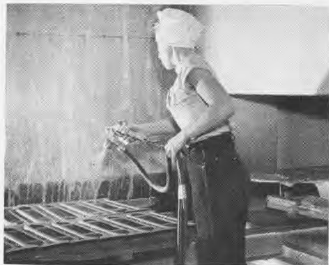
HERE a woman worker sprays on Metalbond. An efficient control of bonding cement can be obtained by carefully applying it to the strips prepared for the bonding process. This is crucial in making the alloy.
