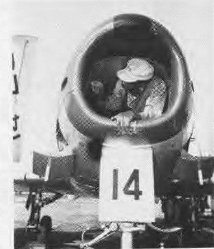
Sgt. Sharp crawls into air intake of a Fury to check air cooling vents of 20 mm cannons.
