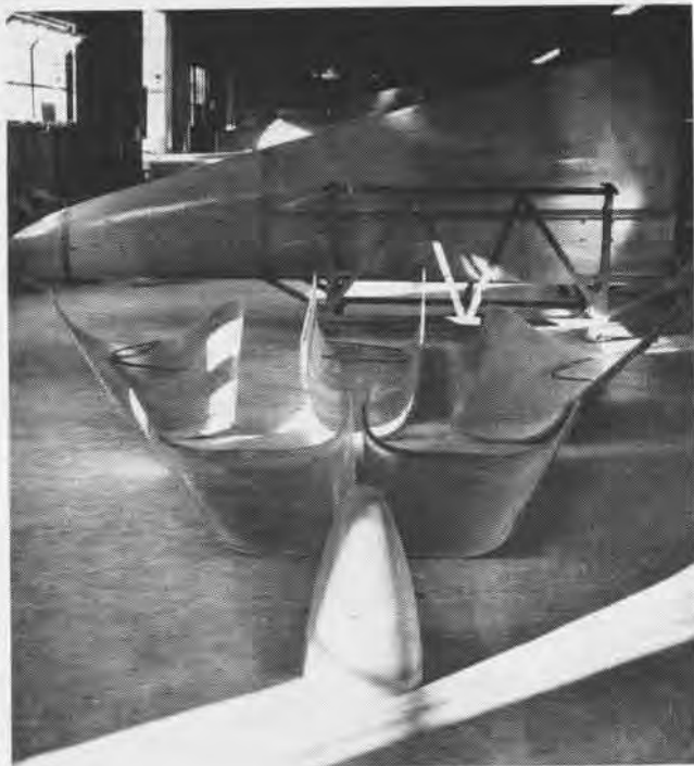
ECONOMY of engineering and manufacture is shown by major sections of honeycomb sandwich construction material for "Stinger Tail."
