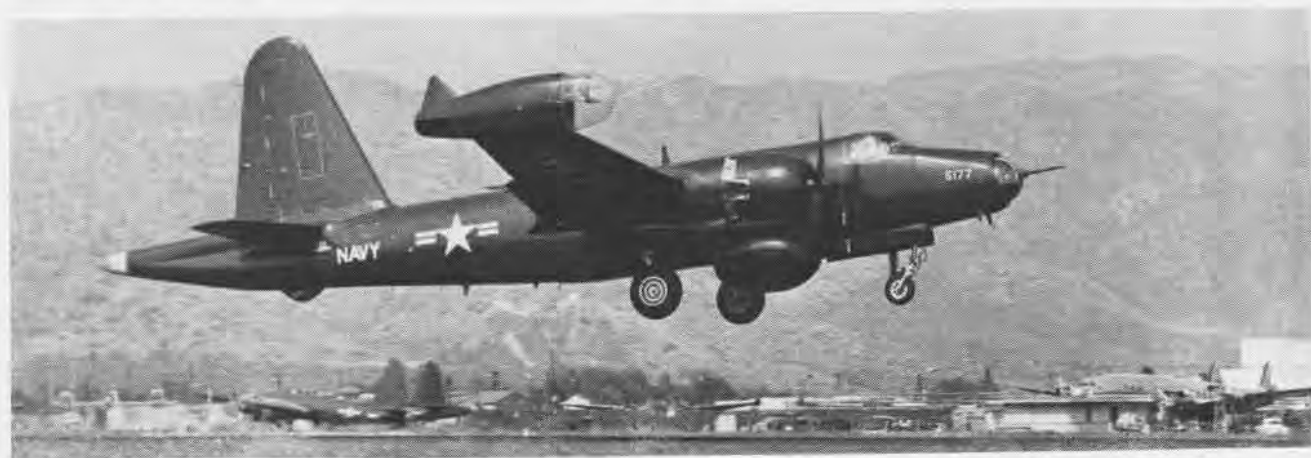
THE LOCKHEED P2V-5 Neptune bomber has a 17-foot reinforced plastic "Stinger Tail." The honeycomb sandwich construction consists of
