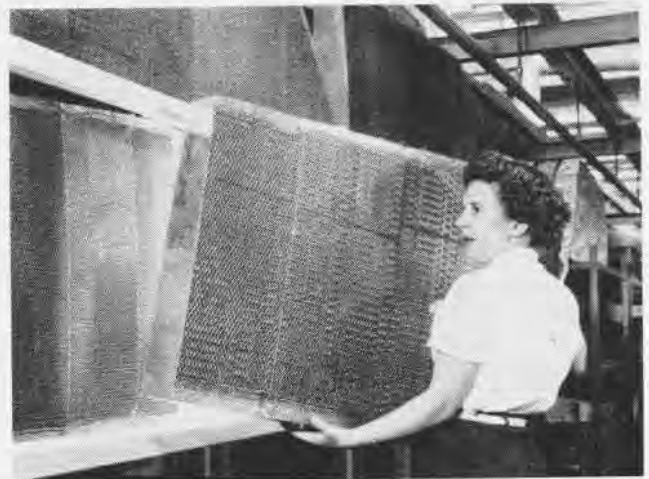
HONEYCOMB , used by Glenn L. Martin, has little stability in initial stage. With sheet metal faces bonded, it's rigid, withstands stress.
