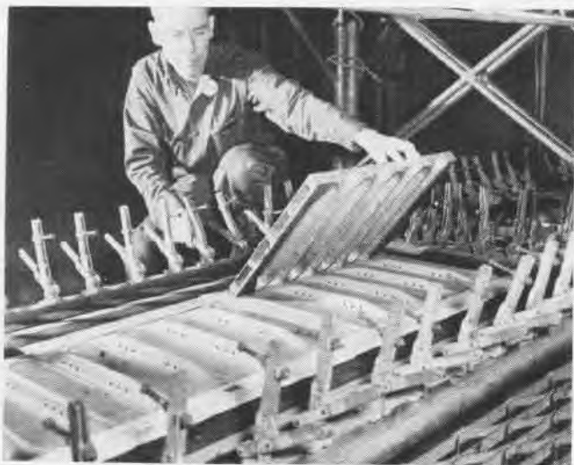
A CONVAIRE workman is shown here using an assembly tool which was especially designed to insure an even distribution of pressure prior to the oven-curing stage of process. Each step is carefully executed.
