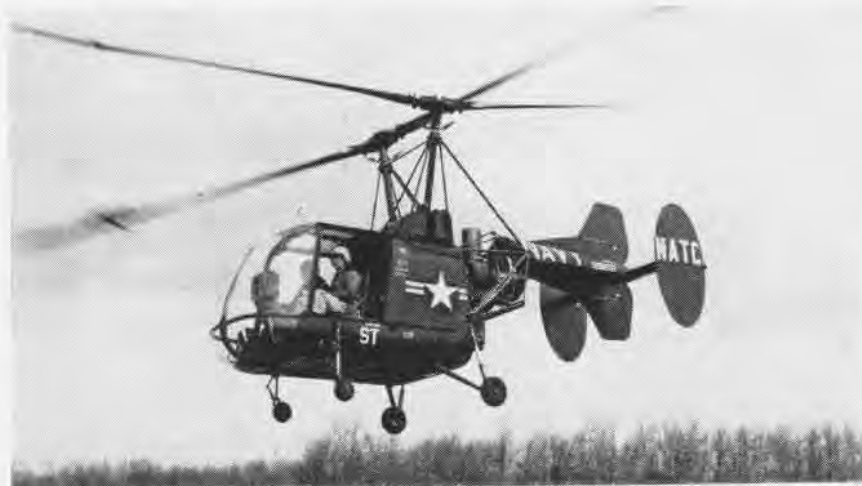
THE INITIAL flight of the Army-Navy sponsored twin-turbomotor helicopter recently took place at Kaman Aircraft. The twin turbines, which produce 380 hp., are mounted side-by-side. The HO4S-1 can be flown with turbines operating simultaneously or separately, providing twin-engine reliability through single engine performance. In actual operation, both turbines are used for vertical take-off and hovering with heavy loads, while in forward flight at cruising speed one turbine is off effecting considerable economy in fuel consumption. Two Boeing-502-2's power it.
