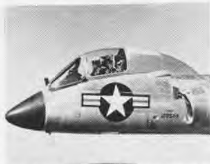
F9F-3 PILOT CAN'T EJECT THROUGH CANOPY
