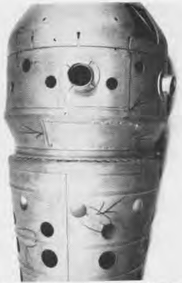
BLACK MARKS SHOW WELDED REPLACEMENTS
