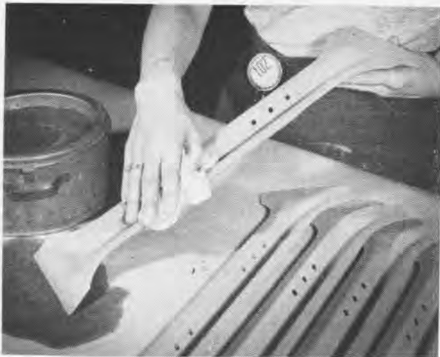
CLEANING process for magnesium alloy prior to bonding requires wiping with low-flash naphtha. This step is vitally important in preparing the magnesium alloy material for the Convaire bonding process.
