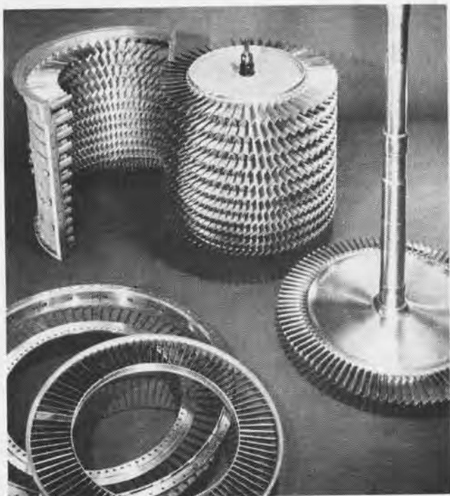
JET TURBINE blades which make a beautiful study in photographic design are made of stainless steel, titanium, S-816 and rimken alloy.
