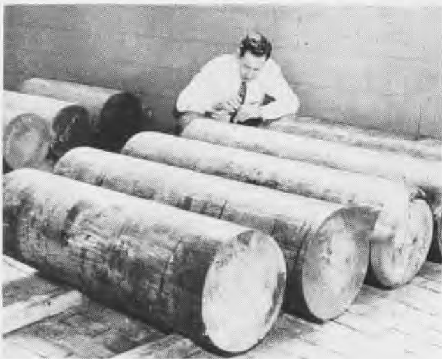
AN ENGINEER is checking the Brinell hardness of these titanium ingots. Formerly, engineers dealt in chunks of few pounds at a time.
