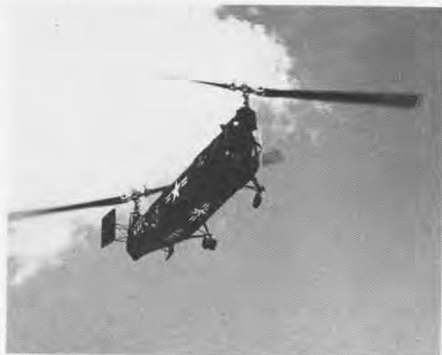
BELL'S ASW 'copter, HSL-1, flew 1,500 miles from Fort Worth to Patuxent River. Equipped with dipping sonar, it's undergoing tests.
