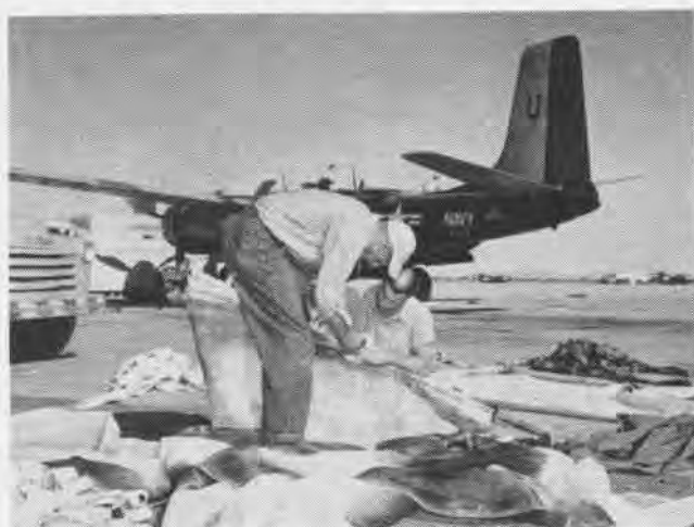
TWO MEN from F-4Skan-8 check towing bar on air-to-air gunnery target. The targets are towed by JD-1's like one in the background.
