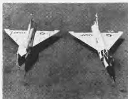
AIRPLANE on left is the first TF-102A produced by Convair for the USAF. This side-by-side trainer familiarizes jet pilots with the F-102A's performance as a weapon.
