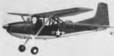
CESSNA'S OE-2 with a service ceiling in excess of 20,000 feet, joins the ranks of the Marine Corps air/ground team. Improvements include armored seats and self-sealing tanks.
