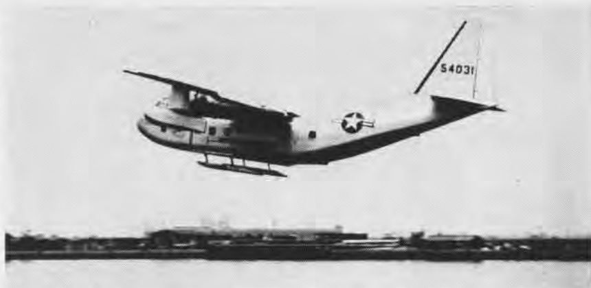
AN AIR FORCE YC-123E cargo aircraft takes off from waters near NAAS Philadelphia on a flight to demonstrate the new Pantobase landing gear. The landing gear, designed and developed by the Stroukoff Aircraft Co., is highly stressed land and water skis which can be used for water, ice or snow operations. The plane is also equipped with conventional landing gear for land operation.
