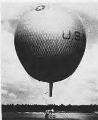
PILOT, at left, dumps sand ballast from basket to effect slow take-off at NAS Glynco.
