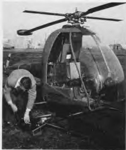
COMPRESSED air from this small portable hand gasoline engine furnishes power for starting.
