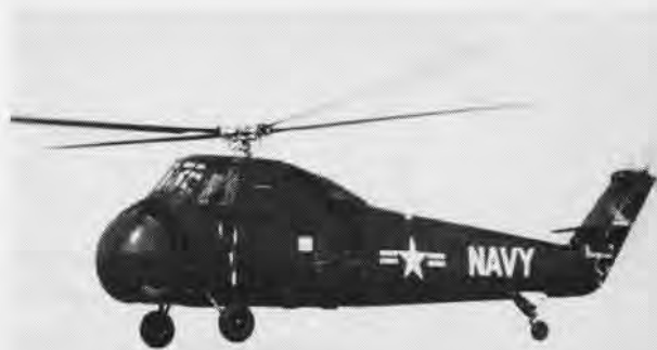
SINGLE ROTOR HSS-1, especially built as anti-submarine helicopter, carries its own lightweight homing weapons for sub destruction.
