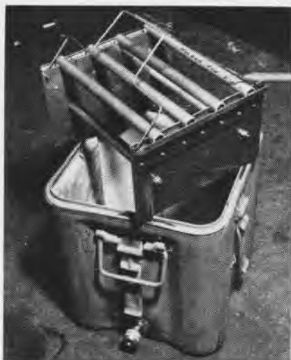
DISC HOLDER SHOWN ATOP CLEANING TANK
