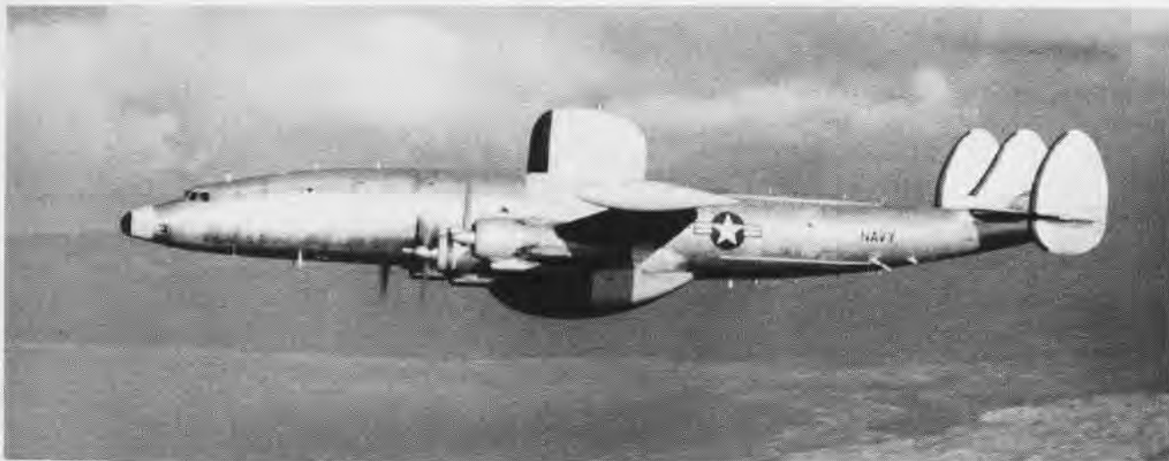
VIGILANCE is maintained by men and equipment of Airborne Early Warning Squadron One in this huge specially equipped Super-Constellation WV-2 aircraft. The flying radar station with its six tons of radar gear capitalizes on height for detection of intruders.
