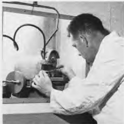
DIAMOND SAW CUTS CRYSTALS ACCURATELY
