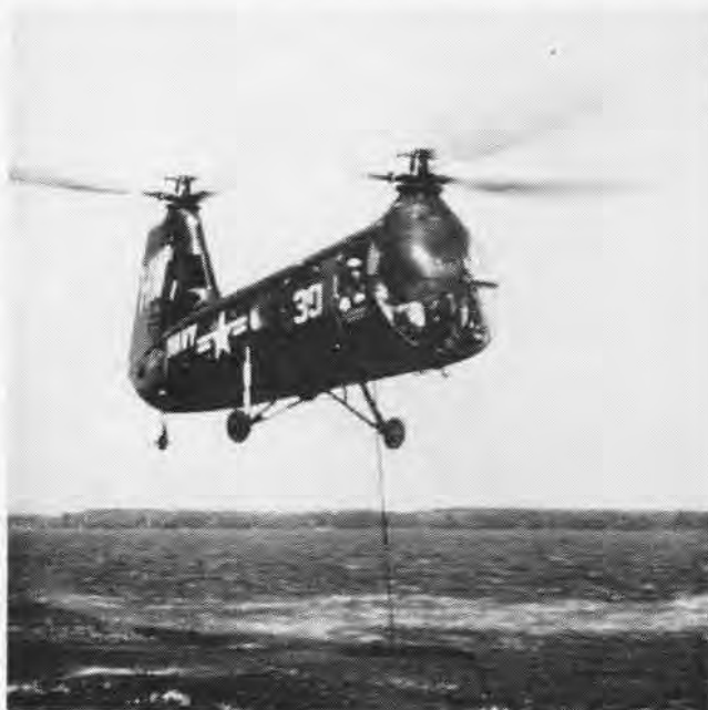
DIPPING sonar gear in play, this Piasecki HUP-2 hovers, just a few feet above surface of the water, pinging and listening.
