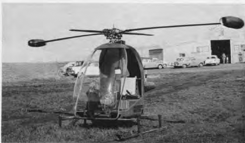
SMALL in structure but mighty in power, the Navy's HOE-1 ramjet powered helicopter sits on company's proving grounds at Palo Alto, Calif., awaiting demonstration trials for Navy officials.
