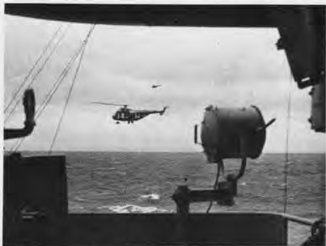
PLANE Number 14 of HS-4 performs task as guard—just one of its various roles—during launching of fixed wing aircraft from Rendova.
