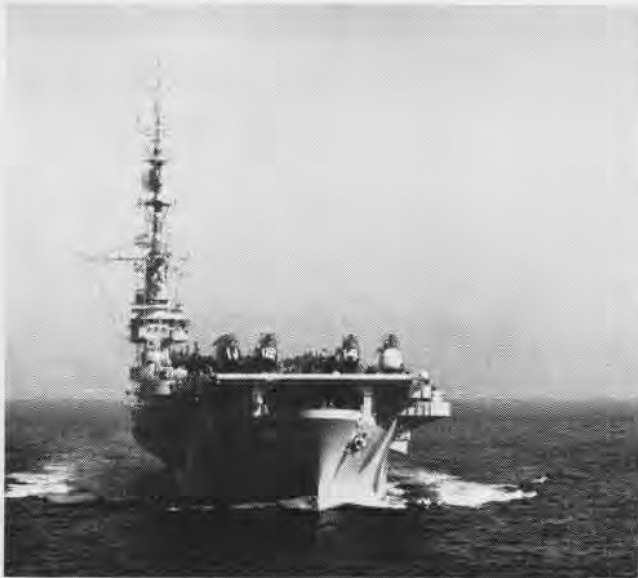
FOUR HS-4 helicopters sit with folded rotors on the bow of flight deck of the USS Rendova during Far East anti-submarine exercise.
