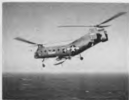
AN ARMY H-21C helicopter demonstrates its latest achievement, gas tanks that can be jettisoned. Designed to extend the range of the helicopter, the two tanks hold 165 gallons.
