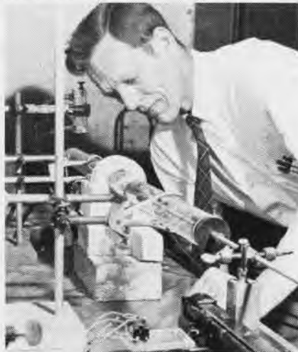
TRANSISTOR CRYSTALS ARE MADE BY ICING
