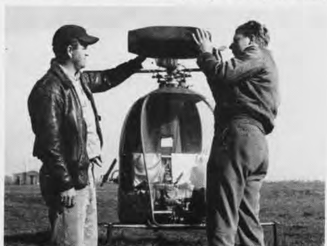
A HILLER mechanic and inspector check HOE-1's ramjet engine just before the takeoff for the flight demonstration of the new 'copter.
