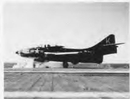
F9F-6 Cougar is 'stopped' by photographer as catapult slings full free. Steam spray is typical of steam 'cat' shots as demonstrated by VF-33 pilot on USS Intrepid at sea.
