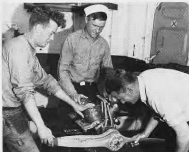
ENGINE tuning by Hulighan, Miller and Jones keeps the drones flying. After recovery, the engine must be cleaned of salt water immediately.
