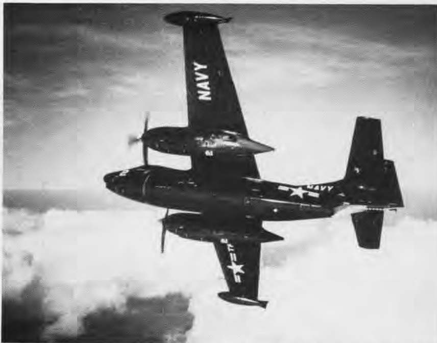
POWERED by two conventional piston engines and one jet, the AJ-2P Savage shows her underside and a few of the openings in her hull where 17 different types of cameras can be installed.
