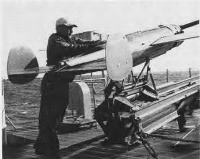
GROSS, AM2, readies the 'bird' for its 200 mph flight. Chute is packed, engine tuned and radio receiver tested before the target drone flies.
