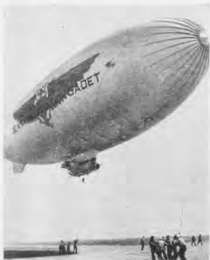
GROUND handlers of VP-871 grab bow lines of the ZSG-2 and "walk" it to its mooring mast.
