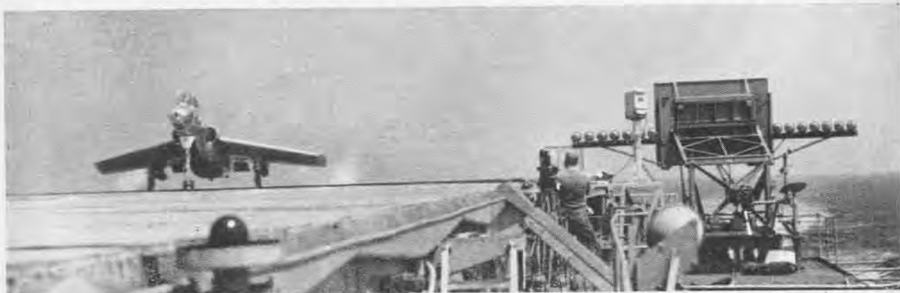
IN F7U-3 Cutlass, here making touch and go mirror landing, Lt. J. H. Cover, VX-3, shot pilot's-eye view of a landing aboard a carrier (on facing page) using British-developed mirror landing system. U.S. Navy pilots are enthusiastic in their approval of the mirror.
