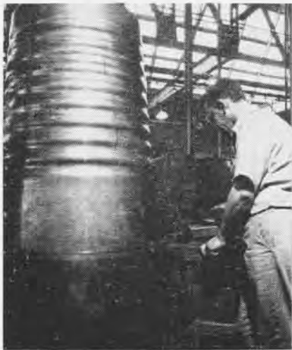
TIME-SAVING multiple electrode spot-welder joins two of the J-57 afterburner components.
