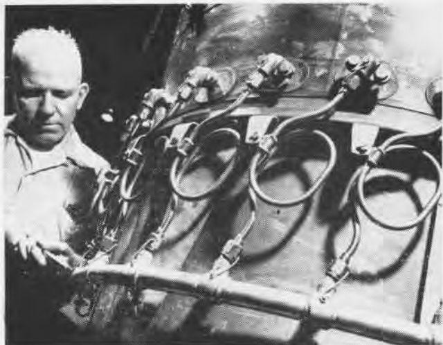
VITAL fuel manifold is then installed which will feed fuel into the air stream of the jet engine. Ignited fuel provides extra thrust.
