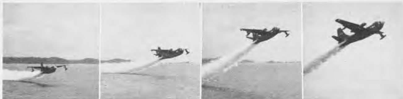
TAKING TIME out from the assigned task of patrolling the Far East defense periphery, a P5M-1 Martin Marlin attached to VP-40, puts on a JATO demonstration for military and civilian observers near Okinawa. The Marlin's R-3350-30WA powerplants are augmented by the 4,000 pounds thrust generated by the four JATO units. This set of sequence photographs was taken from the USS Philippine Sea.
