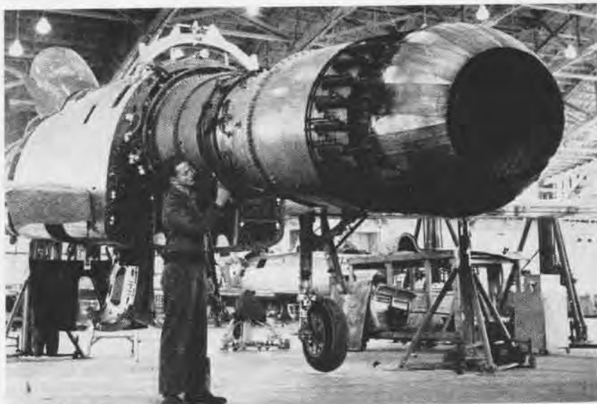
THE PRATT & Whitney J-42 afterburner is the forerunner of this one being installed on a jet fighter. One of the aircraft industry's first successful afterburners was the J-48's tailpiece.
