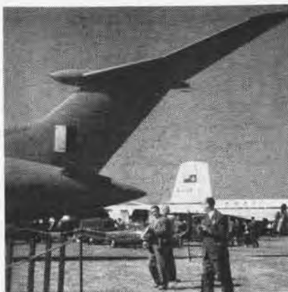
VICTOR HAS HIGH T-TAIL LIKE THE PGM-1
