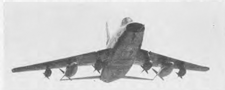
DESTINED for use by the USAF's Tactical Air Command, a North American F-100C, an attack version of the Super Sabre, is pictured in flight with external ordnance and wing tanks. The "C" is powered by a P5W J-57-P-7 turbojet engine with afterburner. Packing four 20 mm. cannon in the nose, the F-100C is equipped with inflight refueling gear and a new electronic bombing device.
