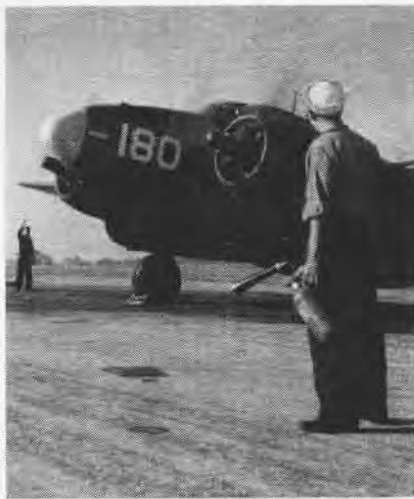
A PV-2 pilot gives this Harpoon a turn-up as starter (left) and firewatch (right) stand by.
