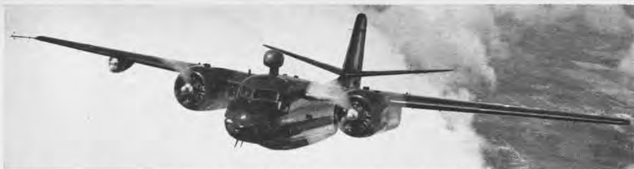
DESIGNED to carry new and larger antisubmarine weapons, the Navy's S2F-2, powered by twin R-1820-82 Wright engines, is shown in flight over Long Island. The new hunter/killer airplane is rapidly being integrated into Fleet use. The enlarged torpedo bay was built into the port side to accommodate the new weapon. To compensate for the S2F-2's increased weight, the tail surfaces have been increased.
