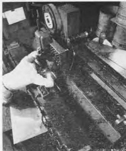
A WORKMAN fuses the three pieces together on a welder. This process is called butt-welding.
