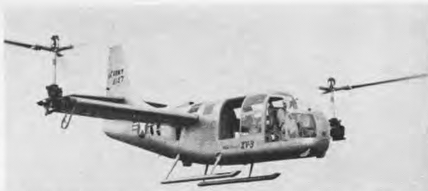
THE ARMY'S XV-3 convertiplane, developed by ARDC and Bell Aircraft, made its first successful flight recently with Bell's chief helicopter test pilot, Floyd Carlson, at the controls. The XV-3 is a tilting rotor type convertiplane, designed to combine the preferred performance features of the helicopter and airplane. The convertiplane was taken to an altitude of 20 feet.
