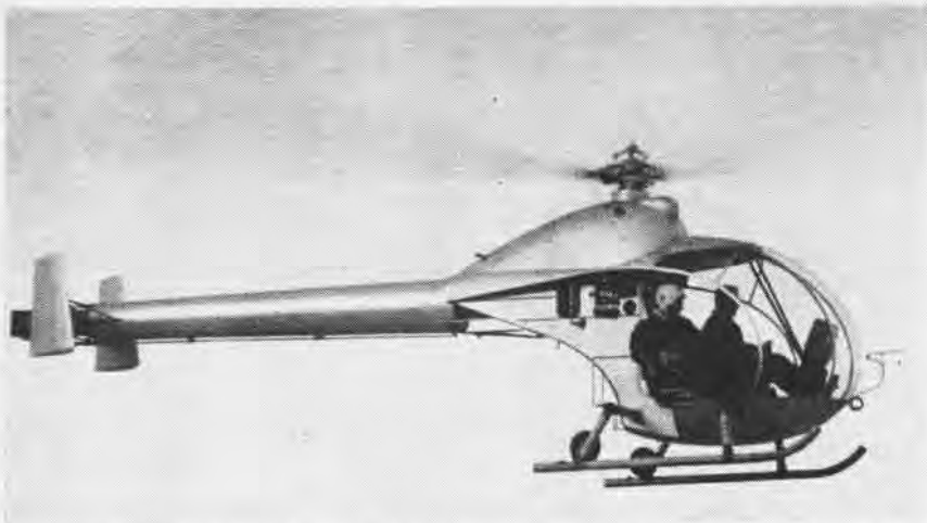
THE FORERUNNER of a new 5-place Spanish helicopter, the AC-13A is pictured in flight at Madrid, Spain. The new helicopter does not utilize the classic tail rotor but counteracts its torque action by orientable jets which are controlled by the pilot through two rudder pedals. Powered by a 260 hp Turbomeca engine, the helicopter was designed by French engineer M. Cantincau.
