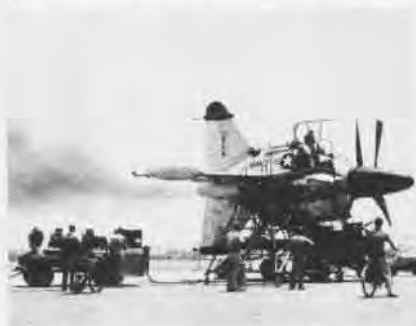
A PLUME of black smoke erupts from the tail pipe of the Navy's XFY-1 Pogo as crushed walnut shells are fed into the intake for cleaning the XT-40-A-14 turboprop engine turbine.
