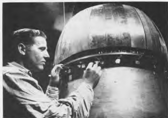
THE BOLTING and wiring into place of the rear section of the afterburner is directed at attaining the maximum structural strength.
