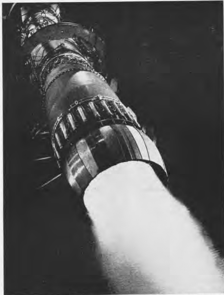
ROARING its defiance to the sound barrier, this powerful J-57 afterburner spurts flames from its exhaust as raw jet fuel is fed into it during tests.
