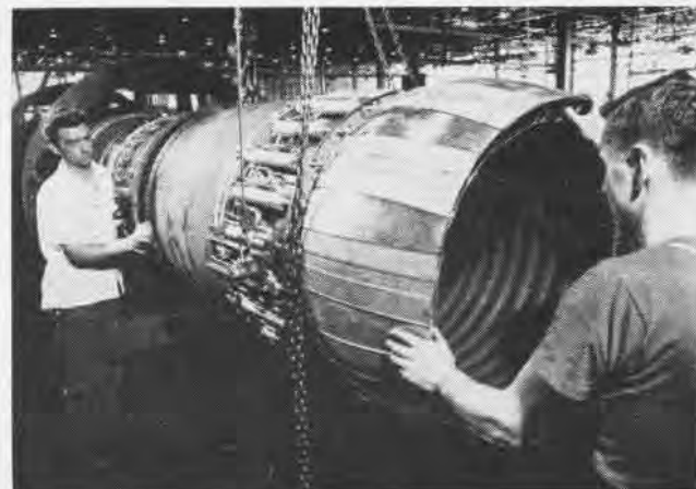
THE COMPLETED afterburner is installed on the J-57 axial-flow jet turbine. This addition will greatly augment the engine's thrust.
