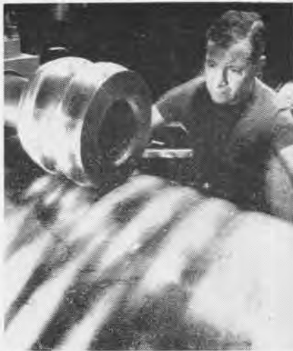
ADDITIONAL strength for the afterburner is obtained by corrugating the stainless steel alloy.
