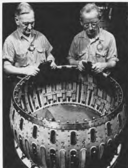
THE IRIS support assembly is one of the most intricate pieces of the J-57's afterburner.
