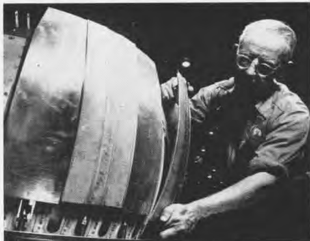
OTHER essential parts of the J-57 afterburner are components of the iris. These stave-like parts control the tail pipe diameter.
