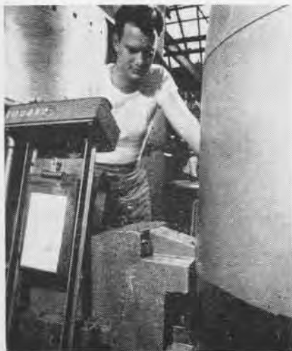
HOLES to fasten rear section to the front are punched by this powerful punch press at P&W.
