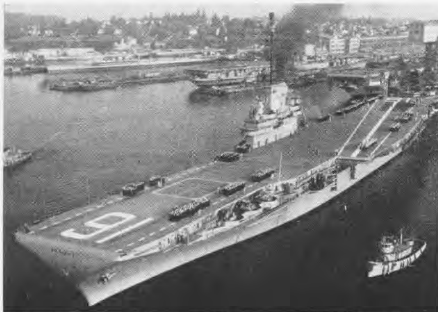
AFTER BEING out of service eight years, the USS Lexington (CVA-16) sails out of the Puget Sound Naval Shipyard, Bremerton, Washington, where she recently completed 22 months of modernization. She heads for her initial sea trials after a conversion which included the hurricane bow, angled deck and steam catapults. Home port for the big carrier will be San Diego.
