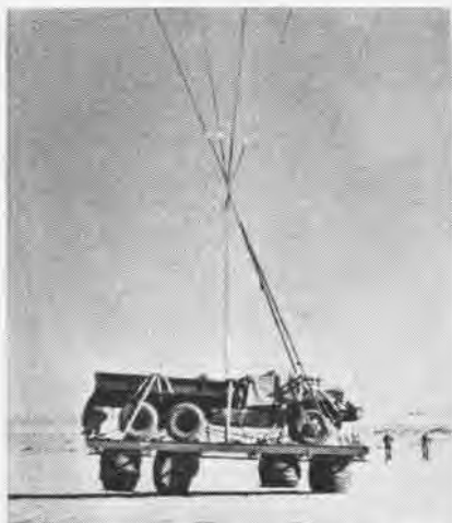
AIR-FILLED shock absorbers—shaped like barrels—cushion the impact of 2½-ton truck.
