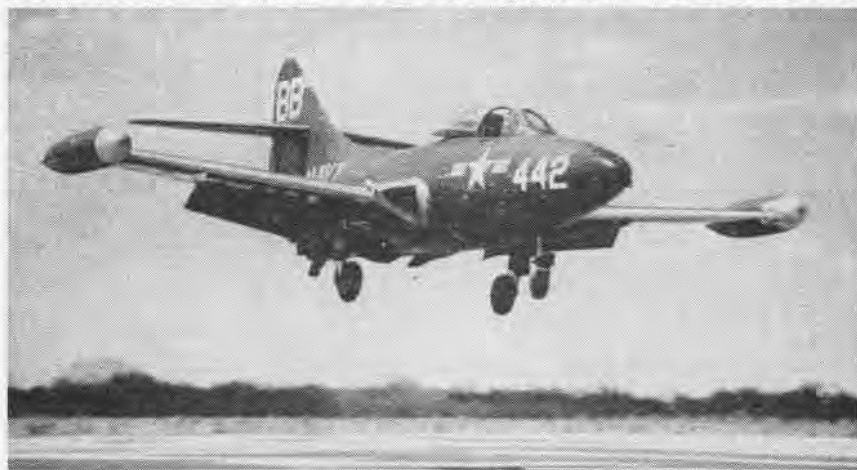
WITH GEAR down and locked and flaps extended, this F9F-2 Pantherjet glides into the groove on the final approach. The student pilot at the controls is enrolled in the 100-hour syllabus.
