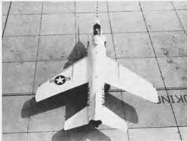
GRUMMAN F11F TIGER'S "COKE BOTTLE" SHAPE IS APPARENT
