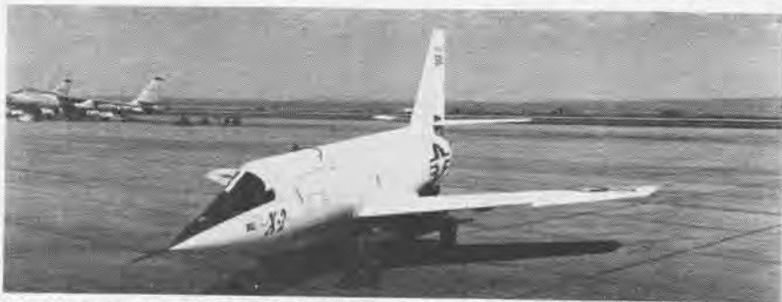
X-2 DESIGNED TO FLY FASTER THAN THE X-1A UTILIZES SKIDS INSTEAD OF WHEELS
