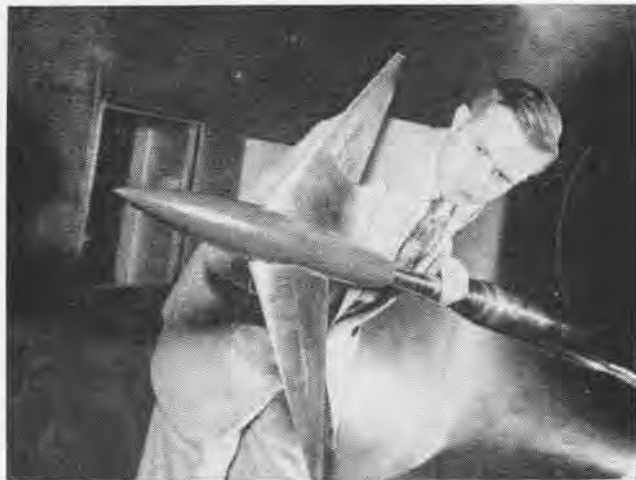
R. T. WHITCOMB IN WIND TUNNEL WITH AN AREA RULE MODEL
