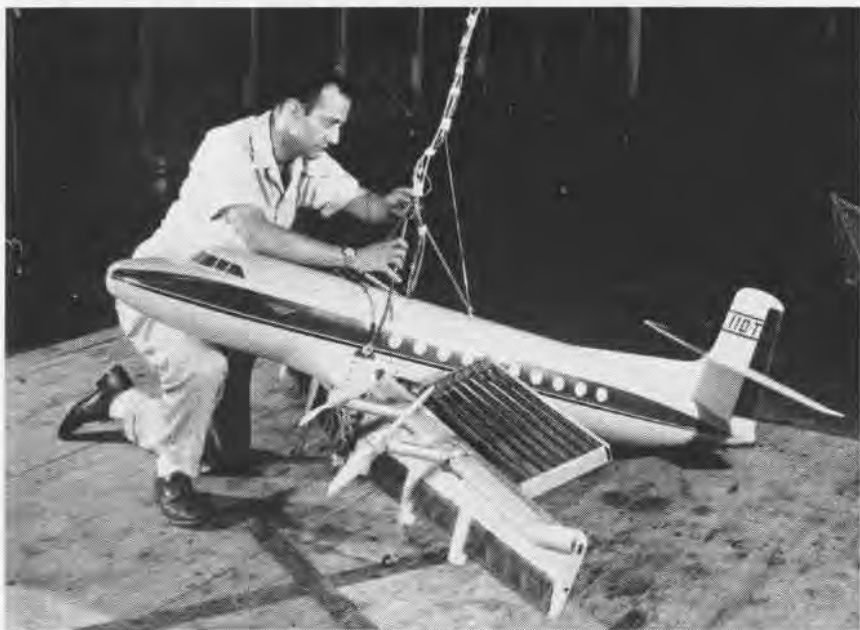
NACA SCIENTISTS are studying vertical flight problems with airplane models, such as this four-engine transport, which derive lift through a system of large vanes and flaps capable of directing the propeller slipstream downward for low-speed or hovering flight. NACA's Langley Aeronautical Laboratory is studying questions of dynamic stability and control in hovering, vertical take-off and landing, and transition to forward flight. Here a technician checks the cables which supply power to the model and provide safety control for the free-flight tests.
