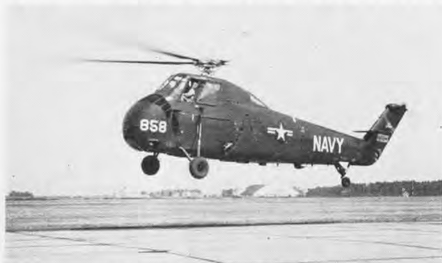
HIGHLY maneuverable and versatile, the anti-submarine HSS-1 comes in for an easy landing on the ramp at Service Test. Pilot Lt. J. L. Blades is just returning from three hour test hop.
