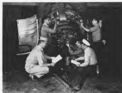
TAD CREW from three helicopter squadrons make a check on R-1820 engine of an HSS-1.
