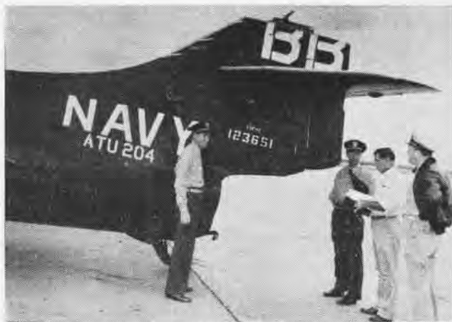
DISASSEMBLE AND TRUCK TO CORPUS WAS VERDICT ON THIS F9F P AND E MAN GIVES HIS DIAGNOSIS ON REPAIRING TAIL DAMAGE
