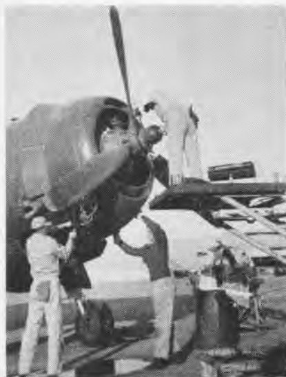
CORPUS MECHS CHANGE ENGINE AT EL PASO
