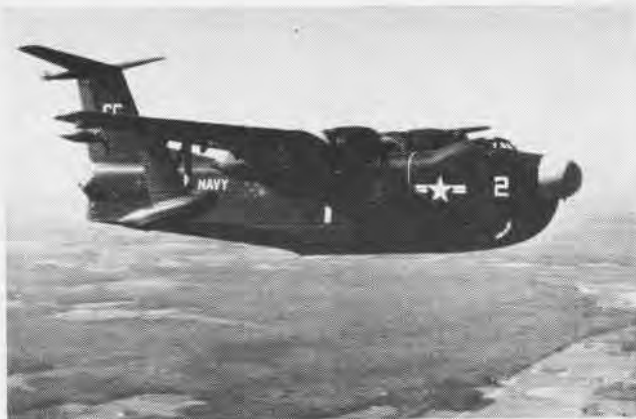
THE NEW P5M-2 is easily distinguished from its predecessor, the P5M-1, by the high "T" shaped tail. The plane weighs 56-tons fully loaded.
