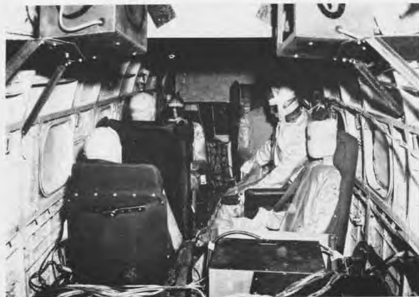
SIX DUMMIES rode a worn-out transport plane through a severe crash landing staged by research scientists. Instruments measured forces exerted on passengers seated in various positions.
