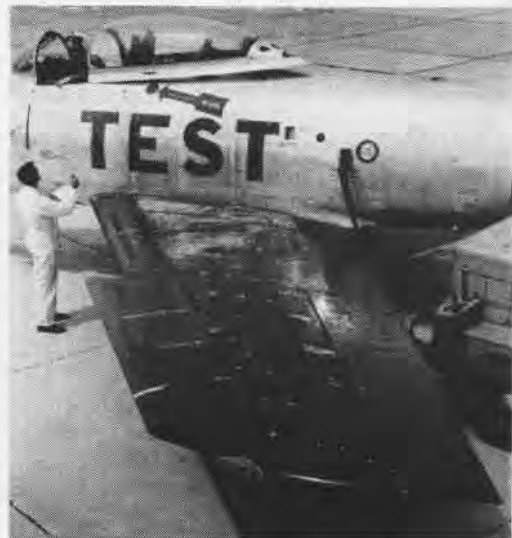
EXTENSION of wing leading edge to improve lift of sweptback wing is flight-checked by wooden contour.
