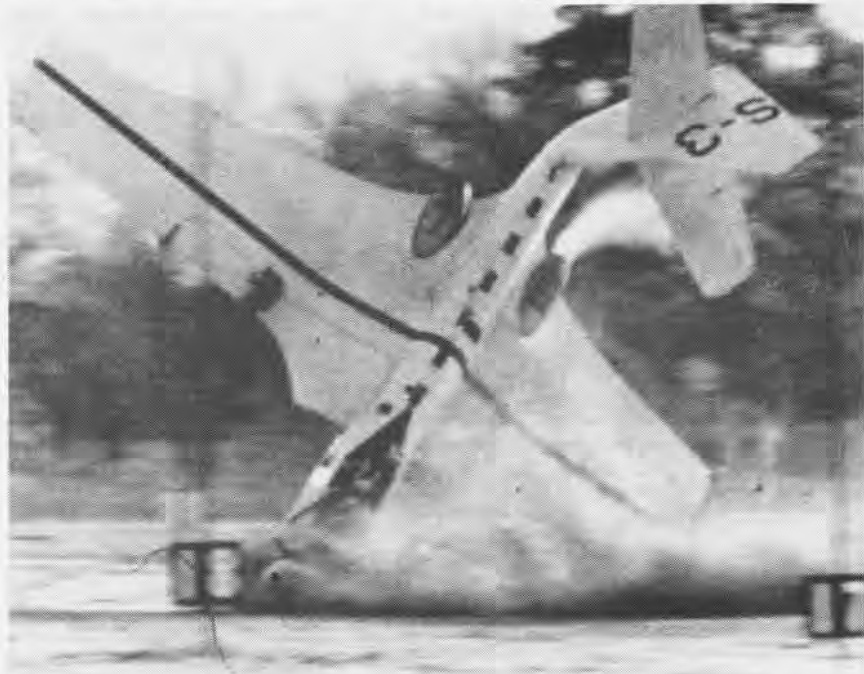
CRASH and fire research are leading to design principles which will increase safety. Piston and jet planes, such as this cartwheeling Phantom, were used in the Lewis Laboratory program.
