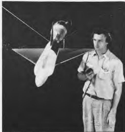
DYNAMIC stability testing is accomplished by using oscillating models like the F-102 fighter shown here.
