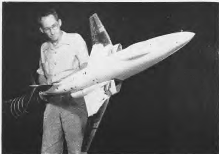
VALUABLE indications to the designer of flight performance to be expected of a new airplane are obtained in wind tunnel tests. Here an F-101 model is mounted for tests.
