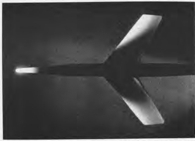
SIMULATED aerodynamic heating on a model placed in a jet of hot gas shows how sharp nose and thin wing edge heat more rapidly.
