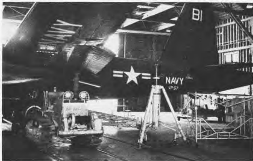
HERE'S THE 'LOCOMOTIVE' WHICH PULLS AIRPLANES INTO THE HANGARS AT NAS WHIDBEY
