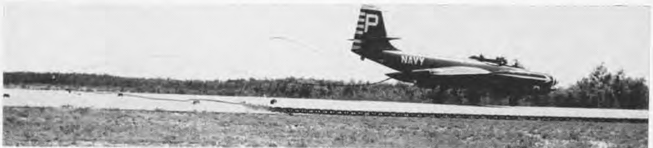
DURING a demonstration of emergency arresting gear at NAS Cecil Field, the tailhook of an F2H Banshee from VF-62 whips the wire rope into snake-like design as the wire is engaged. The gear has been in use
