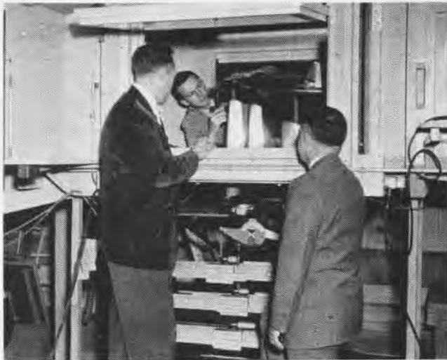
EVEN in these times of supersonic flight, much basic knowledge must still come from subsonic windtunnels. Here students install a model.
