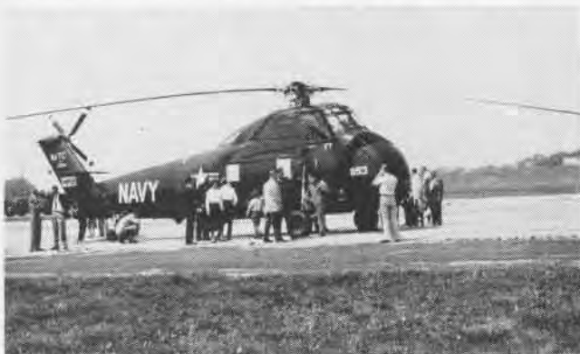
LATEST NAVY model, Sikorsky HSS-1, cuts 56-foot swath as it executes anti-submarine missions. It is expected to replace HO4S-3's as H/K.
