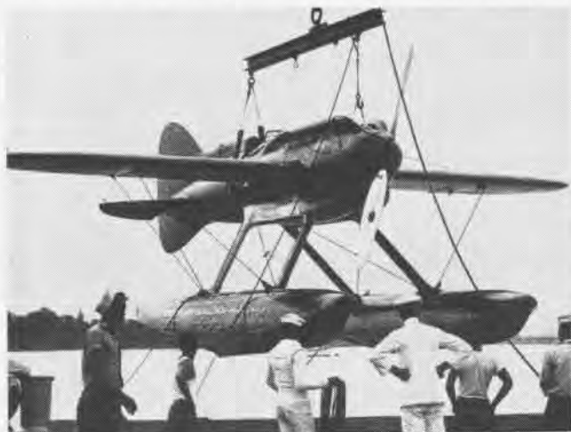
MONOPLANE version of "Mercury" seaplane racer didn't make 1929 Schneider because of baffling problems in ignition, cooling, weight.
