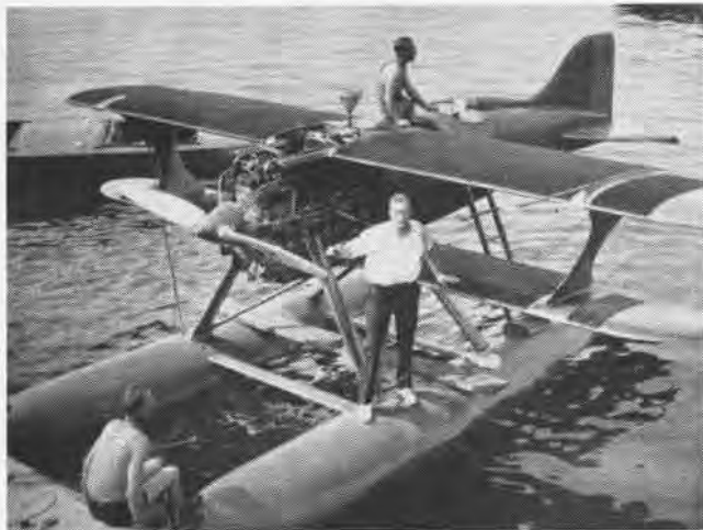
LT. AL Williams stands on float of his Navy-built "Mercury" racer. High speed pontoon flutter prevented entry in 1927 Schneider Race.
