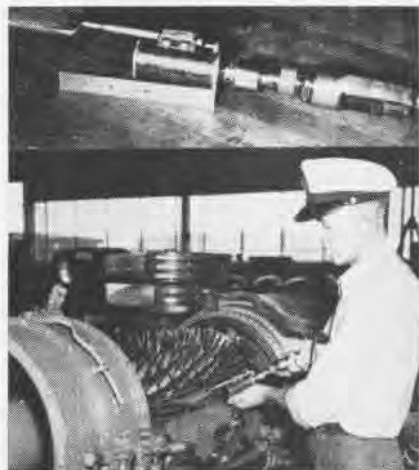
BLADE CLEANER IS USED ON J-34 ENGINE
