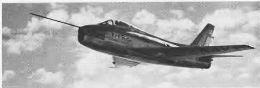
POWERED by a J-65-W-4 gas turbine, the FJ-4 Fury is the latest of this noted series to come off production lines at North American. Its Sapphure power plant generates 7,800 pounds thrust.
