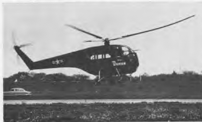
DOMAN'S YH-31, four litter utility-ambulance type craft, built for the Army, is designed for rugged country or combat area operations.
