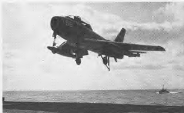
WITH THE power-on approach and speed brakes extended, less time is consumed by the engine to accelerate to full power on a wave-off.
