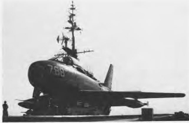
FLAPS may be retracted soon after take-off with no settling and very little trim change. The Fury has excellent stall characteristics.
