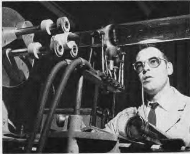
LAB TECHNICIAN blows the glass envelope that will house and protect the mass spectrometer tube as it probes mysteries of outer space.
