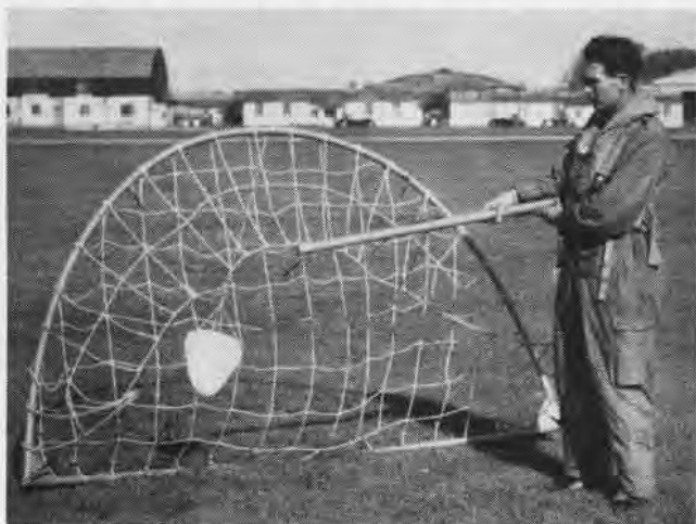
NET IS SIMPLY MADE WITH ALUMINUM FRAME AND SPREADER BAR
