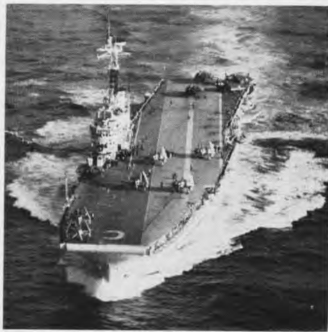
THESE TWO striking photographs of HMS Centaur (left) and the USS Annetam graphically demonstrate the big differences in the two nations' angled deck carriers. HMS Centaur's deck angles at 5\frac{1}{2}^{\circ} from
