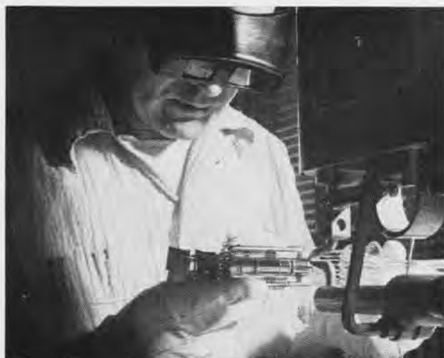
SCIENTIST spot-welds cathode-ray tube. This picture tube, flown on rockets, will gather data on vertical aspects of rockets in flight.
