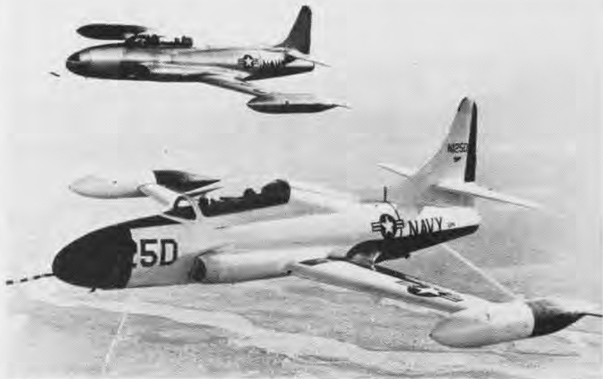
THE NEW Lockheed T2V-1 (foreground), jet trainer designed to operate with aircraft carriers, is paced by a TV-2 two-place jet land-based trainer. The T2V-1 introduces numerous safety and performance features, one of which is a boundary layer control system. Air is ducted into the wing and squirted through tiny holes directed at the flaps and ailerons. This causes the normal airflow to hug the control surfaces giving improved performance and increased lift.
