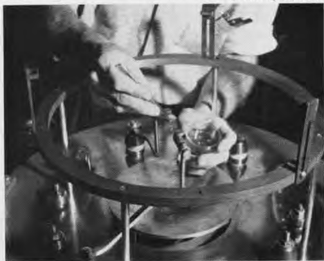
CHARGING a bell jar with metal shavings on electrical filament is one step in coating tubes with metal film a few millionths of an inch thick.
