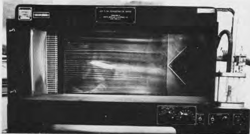
THE LATEST additions to the training of neophyte pilots at the Navy's Pre-Flight School, Pensacola, are two theory of lift simulators that were designed and constructed by the Special Devices Center. The demonstrators utilize kerosene smoke that is drawn through a series of nozzles over the air foil of a scale model aircraft to demonstrate air flow over an airplane wing.
