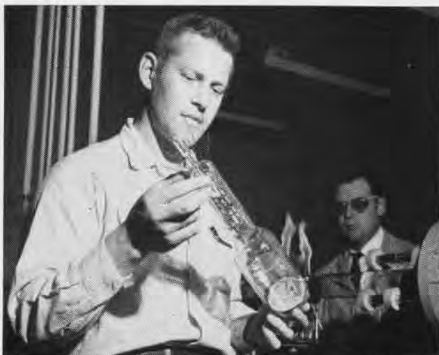
CUSTOM made, these glass envelopes are hand-tailored to fit the special type cathode-ray tube. They must pass many close inspections.
