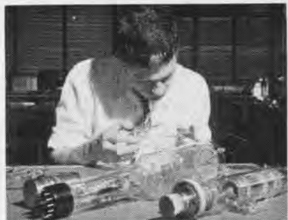
LAST inspection of electron tubes before use. Coked spectrometer is destined to fly high.
