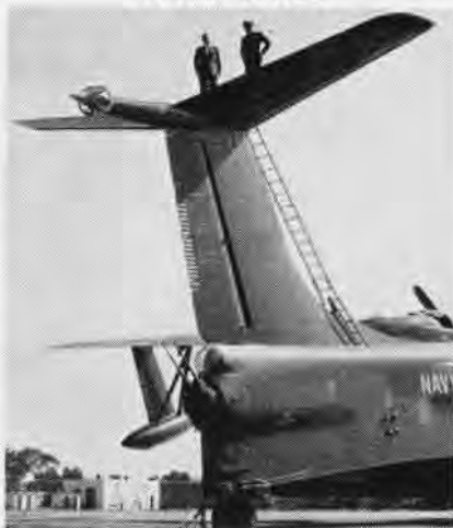
MAMMOTH size of the high T-tail of the P5M-2 Martin Marlin is shown as two men stand on it. This is one of the first of the new planes to be assigned to San Diego patrol units.
