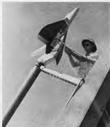
RESEARCH model of transonic airplane is being readied for flight from launcher by technician.
