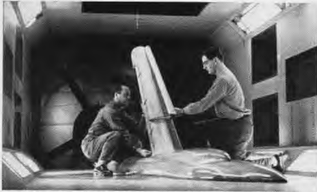
WIND TUNNEL MODELS ARE MADE TO SCALE FROM DESIGN PLANS
