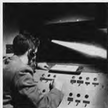
ENGINEER operating rig used for studying film-cooling of combustors at the Lewis Lab.
