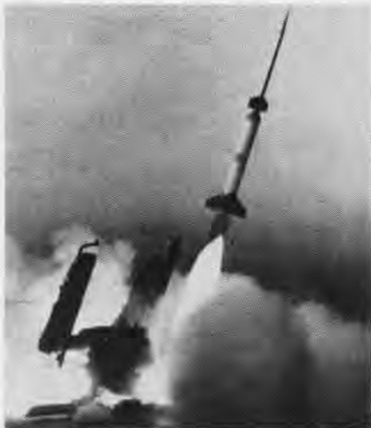
THIS research model was used to study aerodynamic heating in flight recorded at Mach 5.6.
