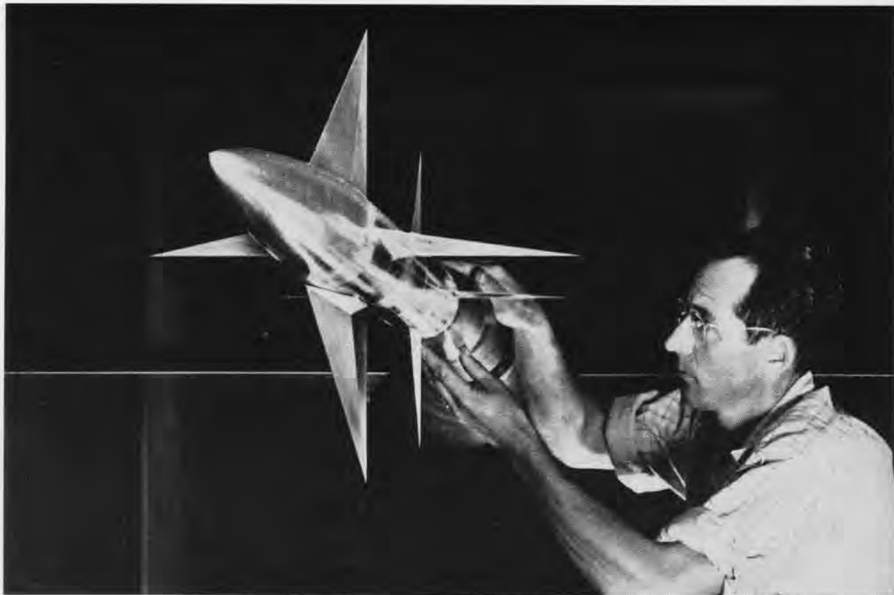
TECHNICIAN readies a missile model for wind tunnel test. Problems in missile design are under constant study in the supersonic wind tunnels of NACA's Ames Aeronautical Laboratory. Missile above has cruciform wings and tail, is one of numerous types being studied.
