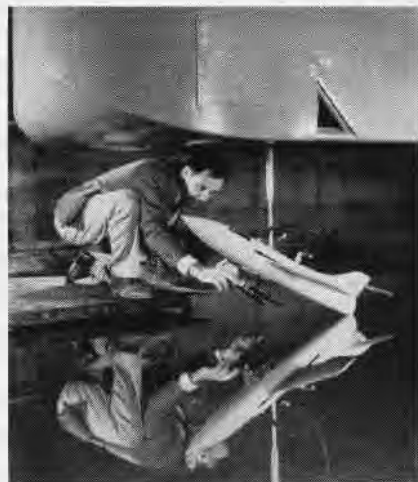
ENGINEER at NACA towing tank prepares model with hydro-skis for a speed test run.
