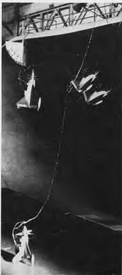
MULTIPLE exposure flight photo of scale-model Convair XFY-1 in Langley full-scale tunnel.
