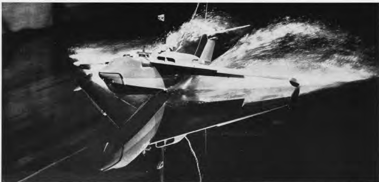
SMALL SCALE model of the XP6M-1 Martin Seamaster is shown undergoing evaluation tests of hydrodynamic characteristics at a towing tank of the Langley Aeronautical Laboratory of NACA. Take-off and landing evaluation tests were made in both rough and smooth water.
