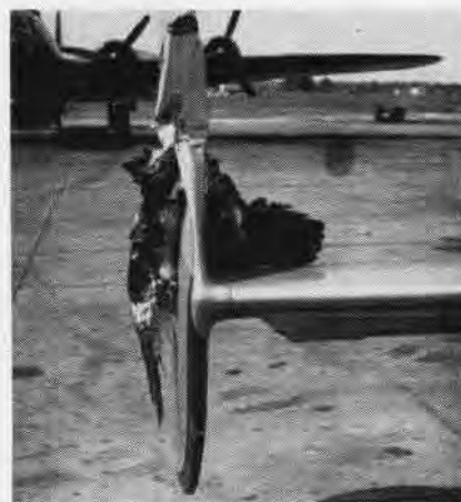
SNB STABILIZER SHOWS GULL'S SAD TAIL
