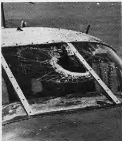
A 40-OUNCE HAWK CAUSED THIS DAMAGE
