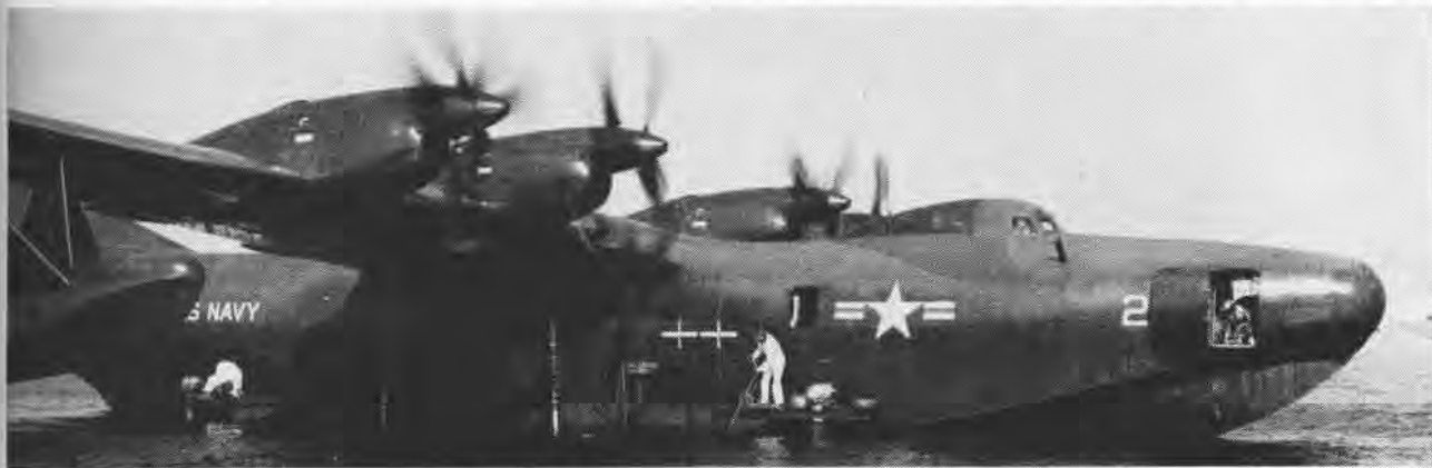
GAS TURBINE ENGINES drive contra-rotating props which pull the R3Y. The turboprop gives good take-off, low speed and low-altitude per-
