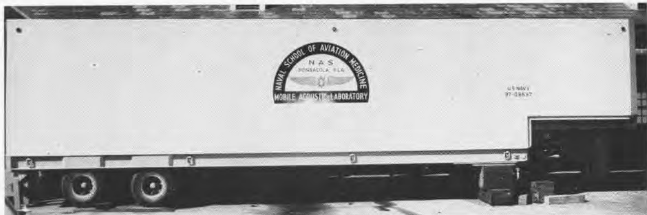
SOUNDPROOFED WITH TWO WALLS, 16-TON TRAILER IS FILLED WITH SENSITIVE ELECTRONIC GEAR FOR TESTING NOISE LEVELS
