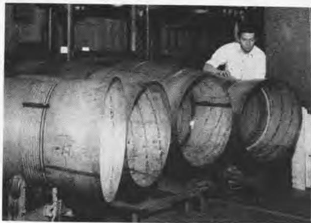
THESE RAMJET combustion chambers are being given a final check. Resembling mammoth bazookas, they were built for Marquardt by Ryan.
