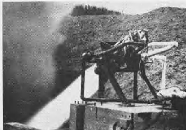
IN 1947, a 6,000-pound thrust Reaction Motors rocket engine like this one powered the X-1 through the sonic barrier in level flight.
