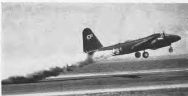
AN EXAMPLE of solid propellant rocket engine is the JATO bottle. This P2V Neptune of VP-8 carried eight bottles to assist take-off.
