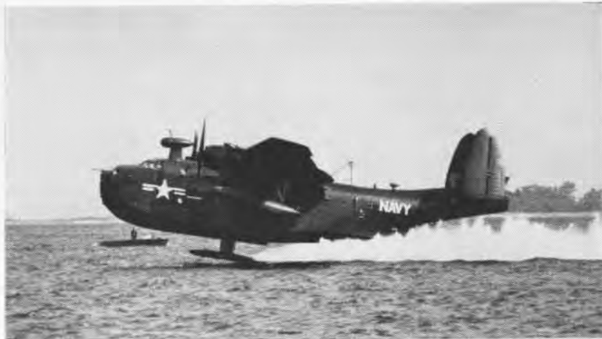
A MODIFIED version of an old PBM Martin flying boat begins a landing on Chesapeake Bay using a hydro-ski that is being tested by the Navy and Martin Aircraft. The hydro-ski acts as a better shock absorber than the conventional ice-bottom hull. Tests are under the auspices of BUAER to determine the practicability of using them on future production seaplane aircraft.
