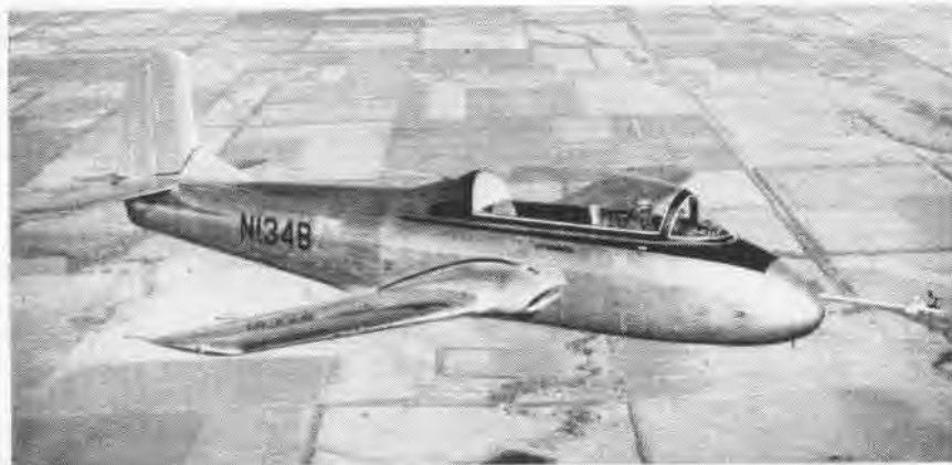
BEECH AIRCRAFT'S experimental Model 73, a two-place trainer, made its initial flight on 18 December near Wichita. Powered by a Continental J69-T-9 turbojet engine and weighing only 4,521 lbs., the new trainer has a speed of 293 knots at 15,000 feet. Its stalling speed is 60 knots.
