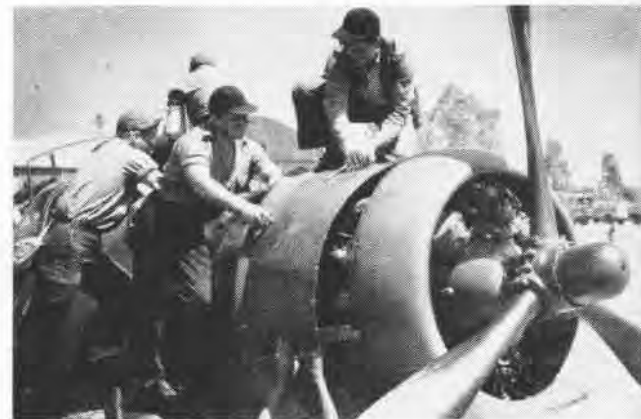
OF 10,000-LBS. of fuel used in WW II reciprocating engine, 3,000 carried load, 2,000 cooled engine, and 5,000 was lost in exhaust heat.
