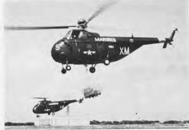
ROCKETS ON ROTORS powered these HRS-2 helicopters. Reaction Motors manufactured these liquid propellant engines for the Marine Corps.
