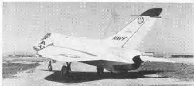
THE DOUGLAS-BUILT F4D is also equipped with the P&W J-57 turbojet, with afterburner. This plane holds three km. world speed record
