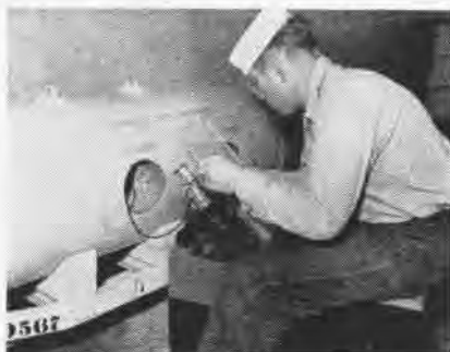
EXTENDER WITH DETONATOR IS INSTALLED
