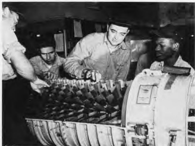
JIM ROARK has checked his own plane. Now he lends a hand at cleaning corrosion from compressor blades of jet engine on another plane.
