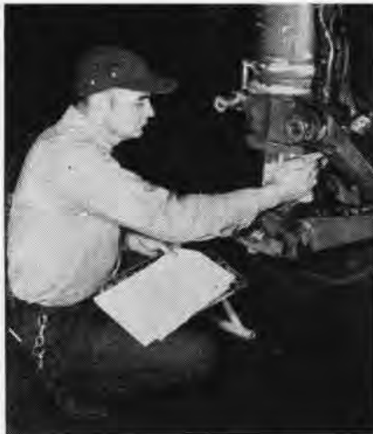
AS PART of detailed pre-flight examination, polished strut on landing gear is inspected.
