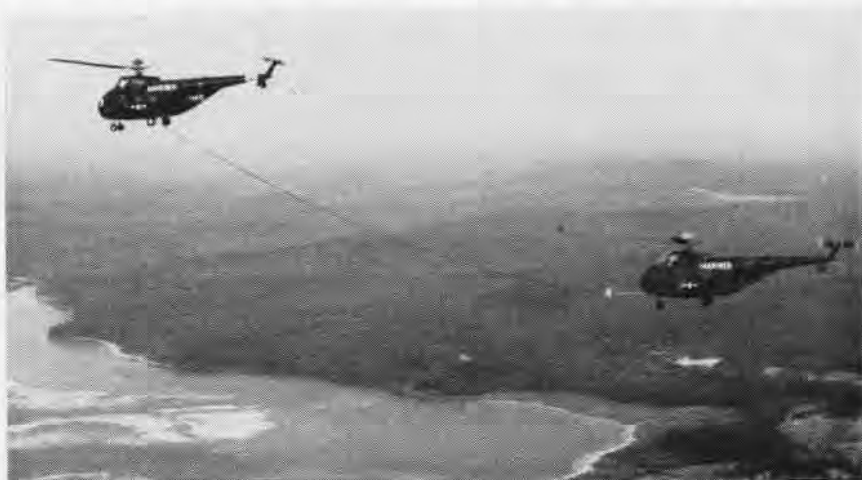
HELICOPTERS of Marine Experimental Squadron One demonstrate the feasibility of in-flight refueling before contractors and representatives of BuAer at MCAS Quantico, Va. The system uses the probe-drogue technique developed for the refueling of carrier-based jet aircraft.
