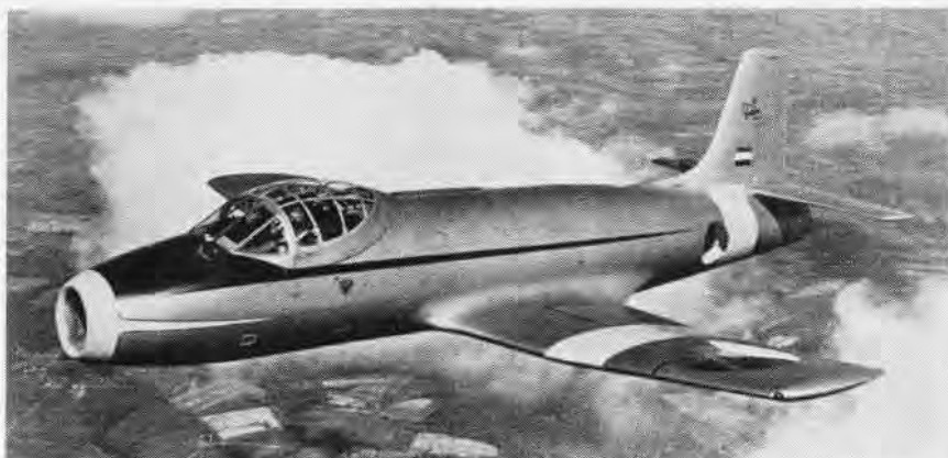
THIS DUTCH-MADE Fokker S-14 jet trainer is being demonstrated to U.S. Navy and Air Force pilots by the Fairchild Engine and Airplane Mfg. Co. Powered by a Rolls Royce Derwent Mk. 8 engine, with 3470 lb. thrust at 14,550 rpm, it has take-off weight of 11,800 lb. S-14 has range of 520 nautical miles at 508 kt. Pilots who have flown it describe it as very stable, easy to fly and land. A large canopy gives all around visibility both during flight and while taxiing.
