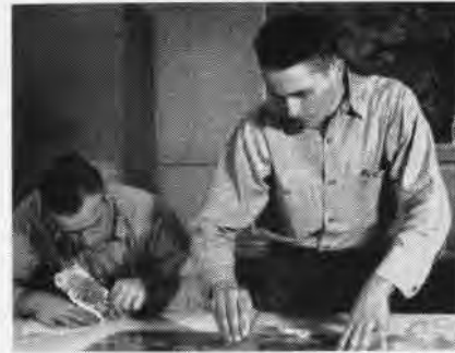
WHILE MAKING a controlled mosaic, accurate sections of photos are squeezed down on board.
