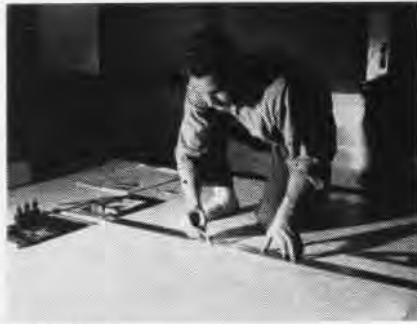
GEOGRAPHIC coordinate lines are carefully plotted on the basic grid for a scale map.
