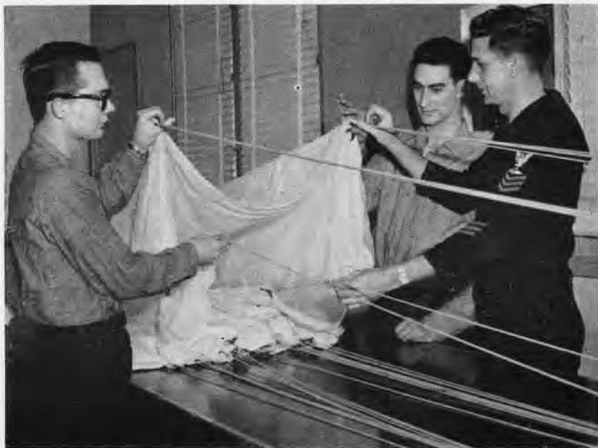
INSTRUCTOR O. H. Deitchler, PR1, in the parachute rigging shop shows James Sprint, AA, and D. D. Humphrey, AA, the right way to pack a parachute. Later their special skill may save lives.
