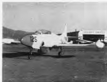
LOCKHEED'S new Navy jet trainer, the T2V-1 Seastar, is scheduled for delivery next fall. The trainer will be powered by either a J-33-P-22 or a J-48-P-8 turbojet engine. Landing speed for the new plane is about 97 knots.
