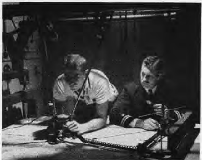
THE PLOTTER used for making maps utilizes red and green lights and glasses with red and green lenses to give photostereoptic detail.
