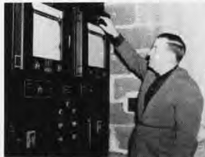
MR. FULTON uses one knob to adjust pressure to simulate altitude up to 70,000 feet.
