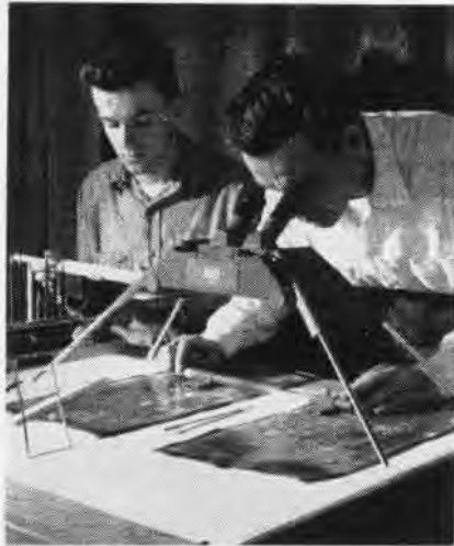
WITH STEREO METER you measure height of hills almost as accurately as with rod and chain.
