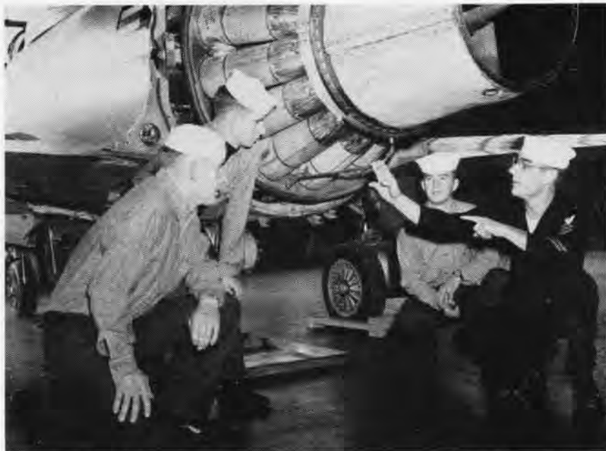
IN THE AIRCRAFT familiarization phase of the school, students are shown how to remove the tail section of an airplane. Instructor Seib uses a jet-powered TV-2 trainer to demonstrate his talk.
