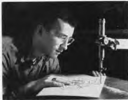
CUTTING OUT a contour is one of the opening steps in the preparation of a terrain model.
