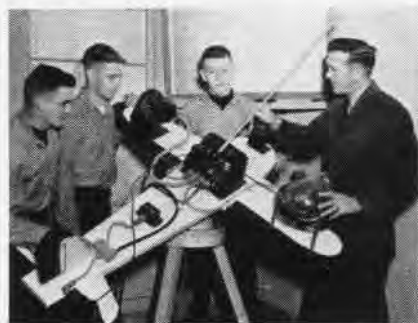
IN ELECTRICIAN rate shop, students get check-out on the gyro stabilized fluxgate compass.
