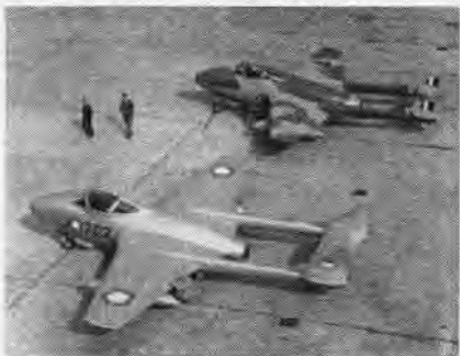
BRITAIN'S new version of the Vampire trainer has dorsal fins and improved cockpit vision. It incorporates a blind flying panel and full provision for twin ejector seats.
