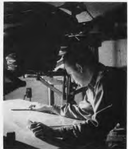
USING RECTIFIER , technician can correct errors in photo which is not exactly vertical.
