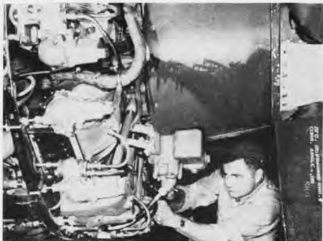
AFTER EACH flight, the plane captain must make a post-flight safety check. Here he traces an oil leak near the rocker box drain sump.
