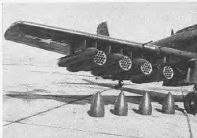
SEVEN AND NINETEEN-ROUND LAUNCHERS HAVE FRANGIBLE CONES
