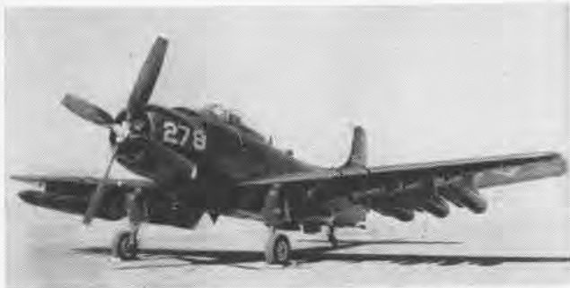
IN OLD SYSTEM, AD-6 CARRIED ONLY 12 FIVE-INCH ROCKETS WITH NEW SYSTEM, AD-6 CAN LOAD 156 OF THE 2.75 ROCKETS
