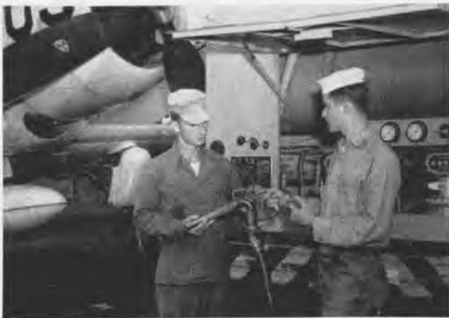
SPARKS ARE ELIMINATED BY ATTACHING CLIPS TO PLANE WING
