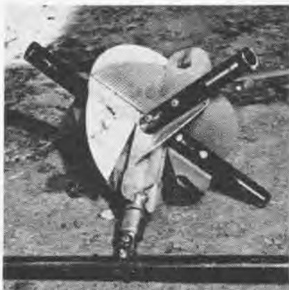
PIPES PROTECT REFLECTOR ON TAKE-OFF
