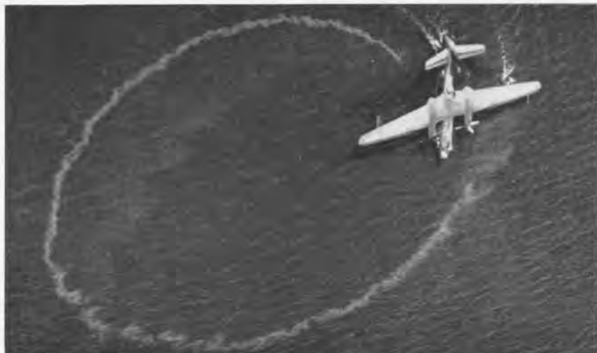
HYDROFLAPS INCREASE MANEUVERABILITY OF P5M-1 MARLIN, SUCCESSOR OF MARINER
