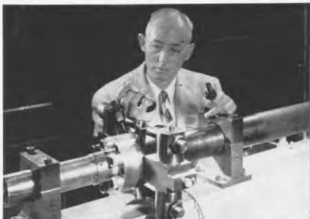
AMOUNT OF FLATTENING OF SPHERE REVEALS FLIGHT PRESSURE
