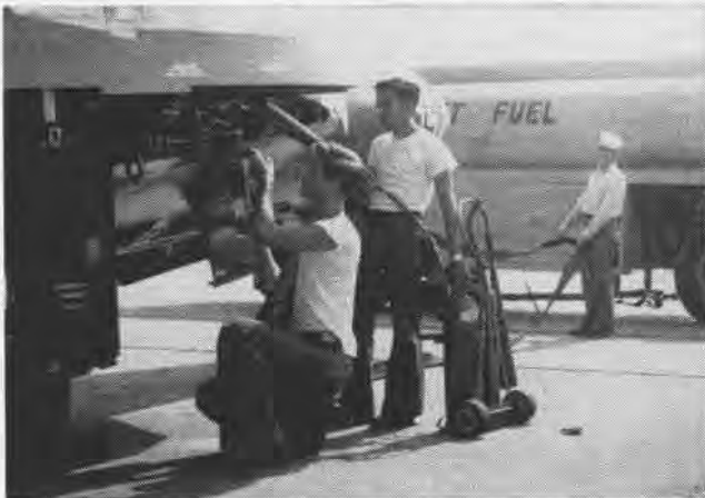
PRESSURE REFUELER NOZZLE IS FITTED TO TANK OF COUGAR
