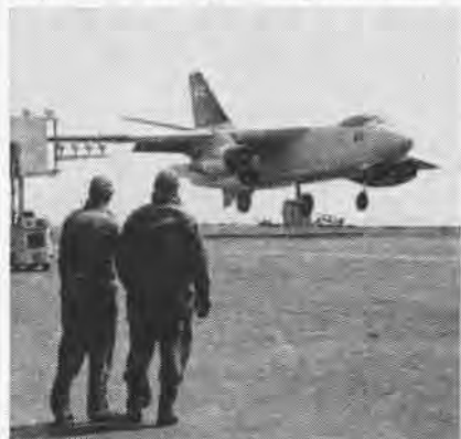
AN A3D SKYWARRIOR from Patuxent River shoots touch-and-go landings aboard the USS Forrestal using the mirror landing system.
