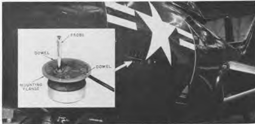
ANGLE-OF-ATTACK TRANSMITTER WILL BE INSTALLED IN MANY AIRCRAFT IN THE FLEET
