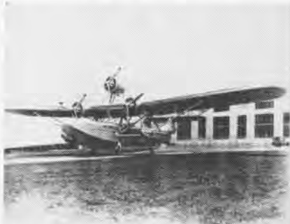
EXPERIMENTAL P2M-1 HAD THREE ENGINES
