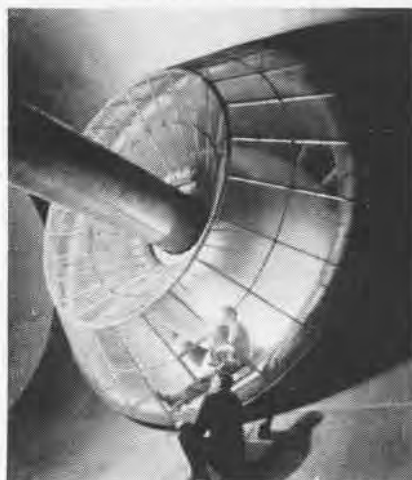
SCREENED INLET OF COMPRESSOR NO. 2
