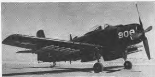
IN OLD SYSTEM, AD-6 CARRIED ONLY 12 FIVE-INCH ROCKETS WITH NEW SYSTEM, AD-6 CAN LOAD 156 OF THE 2.75 ROCKETS
