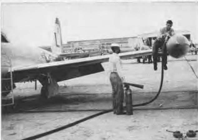
MINIMUM DISTANCE BETWEEN REFUELING OPERATIONS IS 100'
