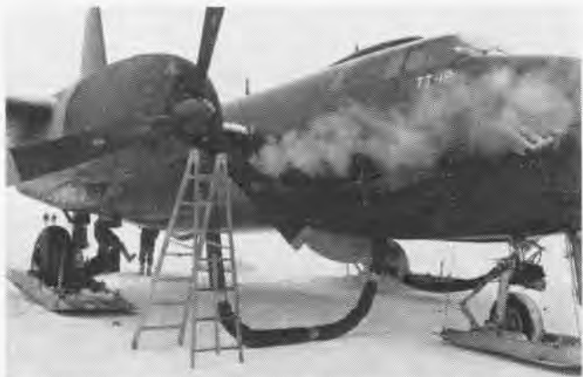
P5V ENGINE GETS ITS PREHEAT, NECESSARY BEFORE STARTING
