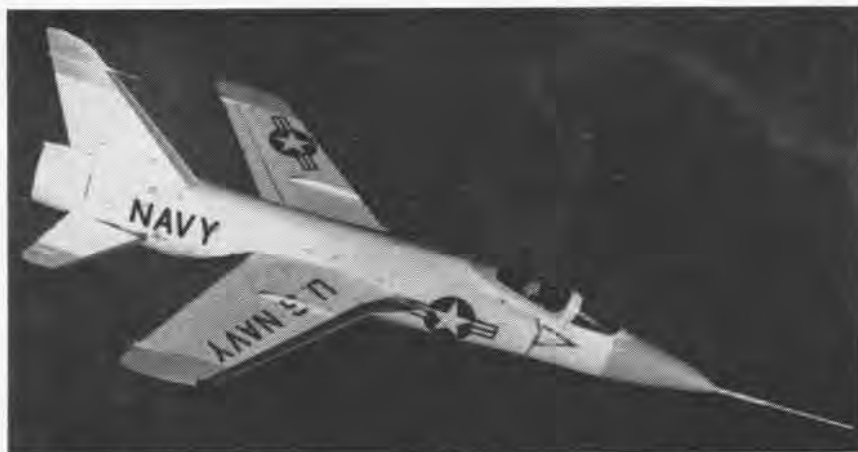
THE GRUMMAN F11F-1P Tiger, a faster version of the Navy's supersonic F11F-1, is powered by the General Electric J-79 turbojet with afterburner. Its indented or pinch waist fuselage is clearly shown. There were minor revisions to the basic Tiger airframe to permit installation of a larger power plant. Capacity of the inlet ducts was increased to allow for a greater airflow requirement, and the aft fuselage was rebuilt to house the larger diameter of the afterburner.
