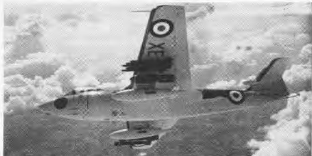
THE SEAHAWK CARRIES BOMBS, WING TANKS, ROCKETS AND GUNS
