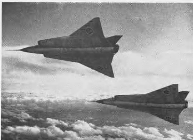
DOUBLE DELTA CONFIGURATION OF THE WINGS IS OUTSTANDING CHARACTERISTIC
