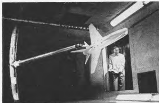
TO STUDY the effects of aerodynamic characteristics at altitudes simulating spinning conditions, this scale model XF8U-1 is used.
