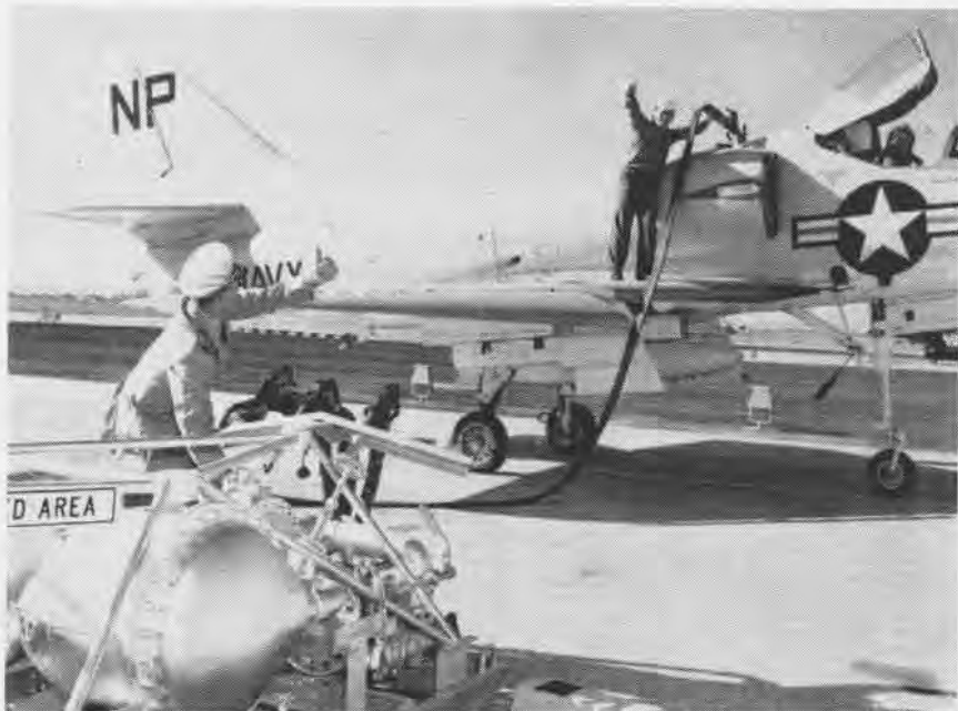
'THUMBS UP!' The new High Speed Refueling System at NAS Moffett Field is ready to go with Capt. Arthur S. Hill, Commanding Officer, opening the first valve. Pilot of the Navy's A4D Skyhawk about to be refueled is Cdr. G. C. Anderson of VF(AW)-3. Facilities of the system include eight stations that accommodate eight aircraft simultaneously. The JP-4 fuel is pumped from a 105,000-gallon tank. Each station fuels an airplane at a rate of 400 gallons per minute.
