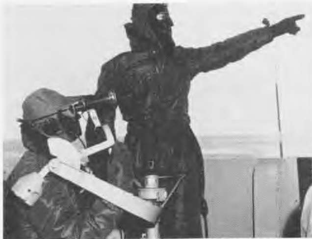
CREWMEN TESTED FACE MASKS AND ELECTRICALLY HEATED SUITS
