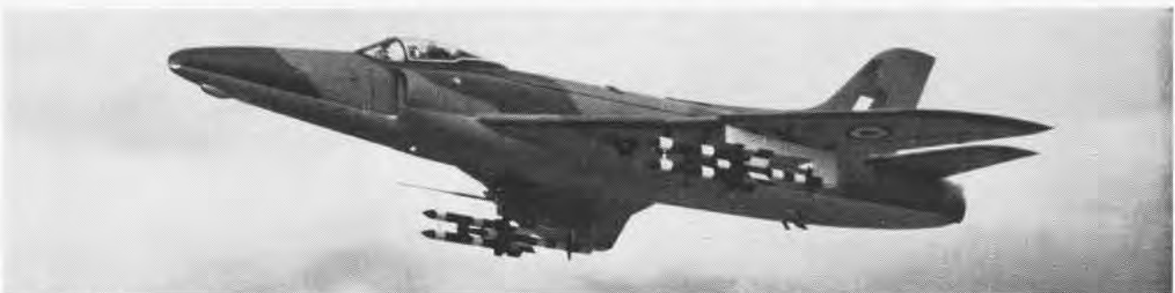
THE PROTOTYPE SUPERMARINE MARK 7 SWIFT IS FITTED WITH TWO FAIREY FIREFLASH MISSILES, BUT IT CAN CARRY FOUR
