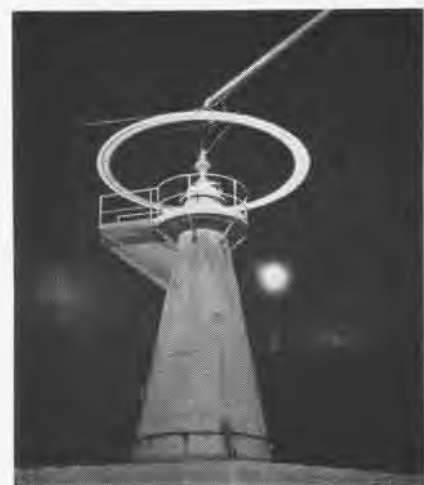
SMALL RAM jets at rotor blade tips form halo effect above Helicopter Test Tower at night.
