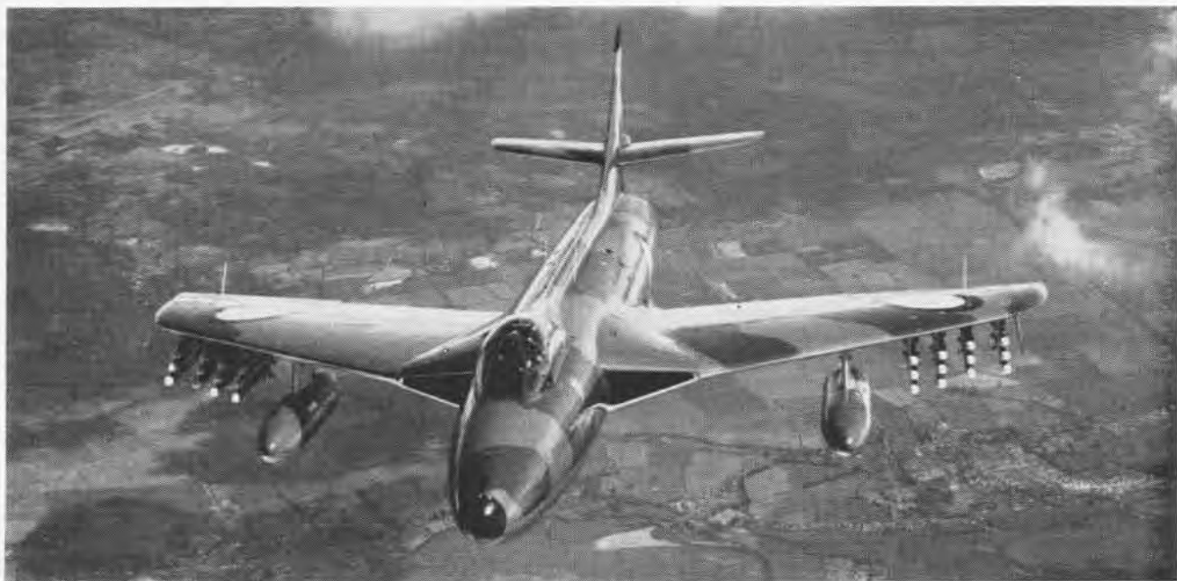
IN THIS FLIGHT, THE HAWKER HUNTER MARK 6 IS CARRYING TWO 100-GAL. EXTERNAL GASOLINE TANKS AND 24 THREE-INCH ROCKETS
