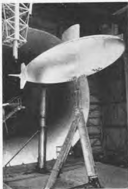
SCALE MODEL IN AN NACA WIND TUNNEL
