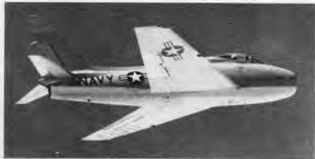
FJ-4, LATEST of the Fury series in production at North American has a high rate of climb and may also deliver externally stored weapons.
