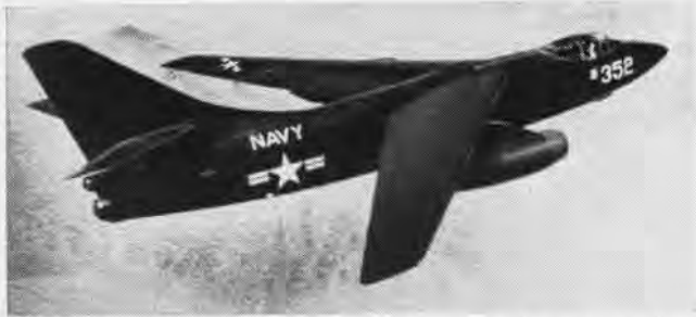
A3D-1 SKYWARRIOR heavy attack aircraft groomed to operate from steam cat carriers, will increase striking radius of the fleet.
