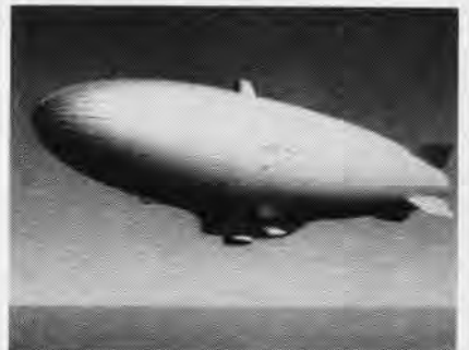
ZPG-2W , sporting radome on top of envelope will be assigned to early warning units.
