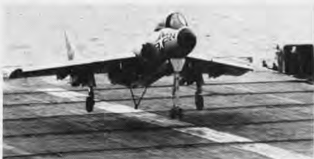
F7U-3M CUTLASS , a twin turbojet carrier fighter equipped to launch air-to-air guided missiles, lands on the angled deck of Sbangi-La .
