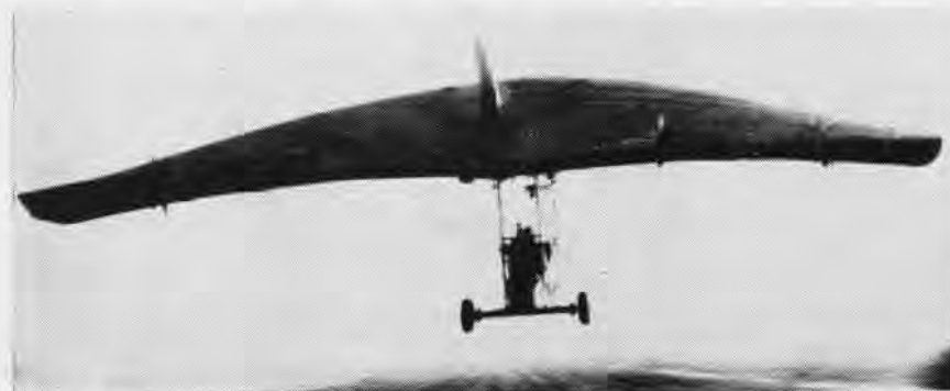
FLYING MATTRESS has a take-off speed of 18 mph and top speed of 45 mph. This is the first prototype with a wingspread comparable to other light planes, but with a delta-shaped wing.
