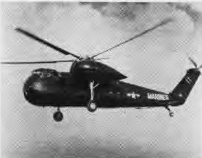
NAVY'S HR2S-1 built for Marines can carry 26 men, their assault equipment, three jeeps.
