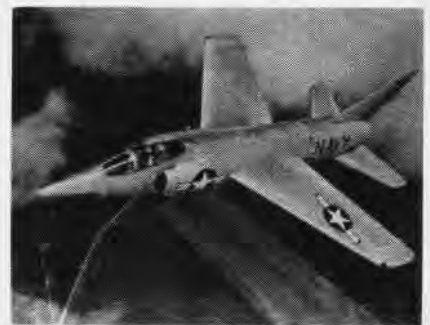
F11F-1 TIGER is first aircraft to incorporate area rule or "coke-bottle" fuselage.
