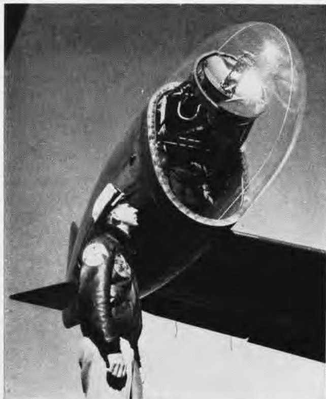
This searchlight on the wingtip of a P2V Neptune uses a lot of current, but it produces 75 million candlepower.
