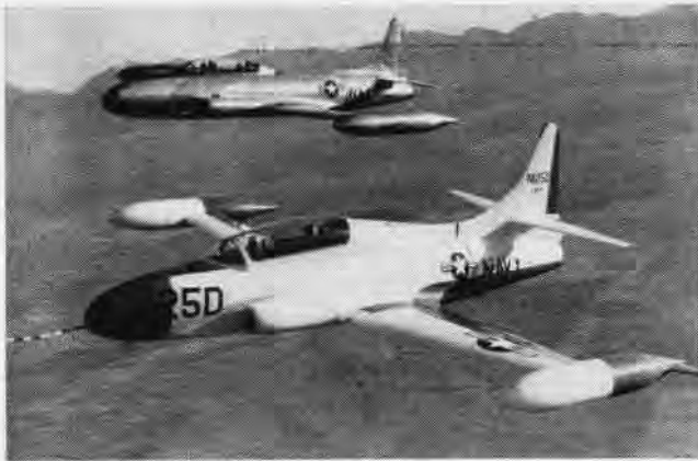
T2V-1 JET trainer, an improved version of the TV-2 which it leads, has the equipment required for training operations aboard carriers.
