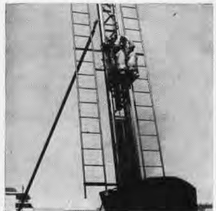
HOW TO BLOW your top is taught with this ejection seat trainer. It is also used for demonstration purposes for families of pilots and crew members at NAS Corpus Christi, Tex.
