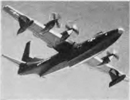
THE BIG R3Y-1 Tradewind transport can fly at speeds above 350 mph and carry 24 tons.
