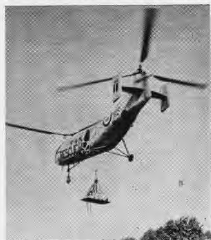
EQUIPMENT WAS CARRIED UNDER FUSELAGE
