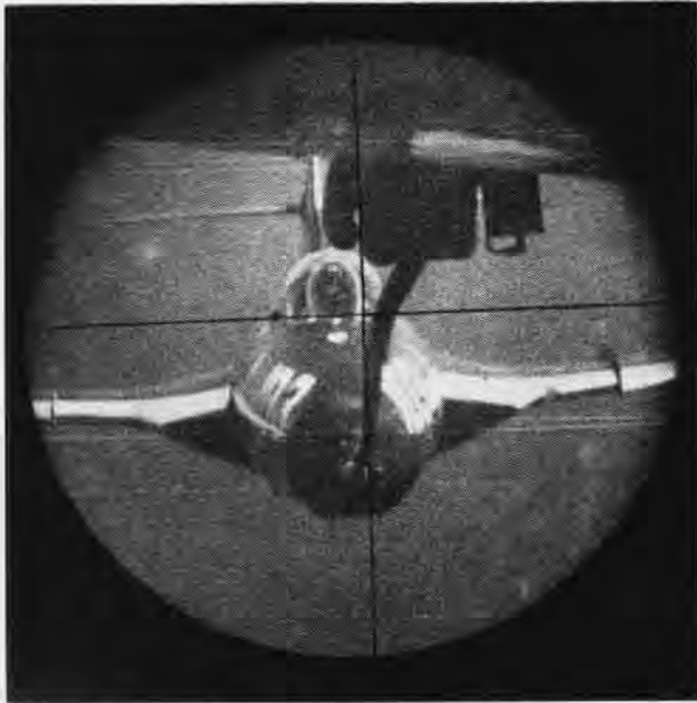
'FILL 'ER UP'—Inflight refueling of an F9F-8 Cougar fighter as seen through the Bomb Director Periscope of the AJ Savage tanker.
