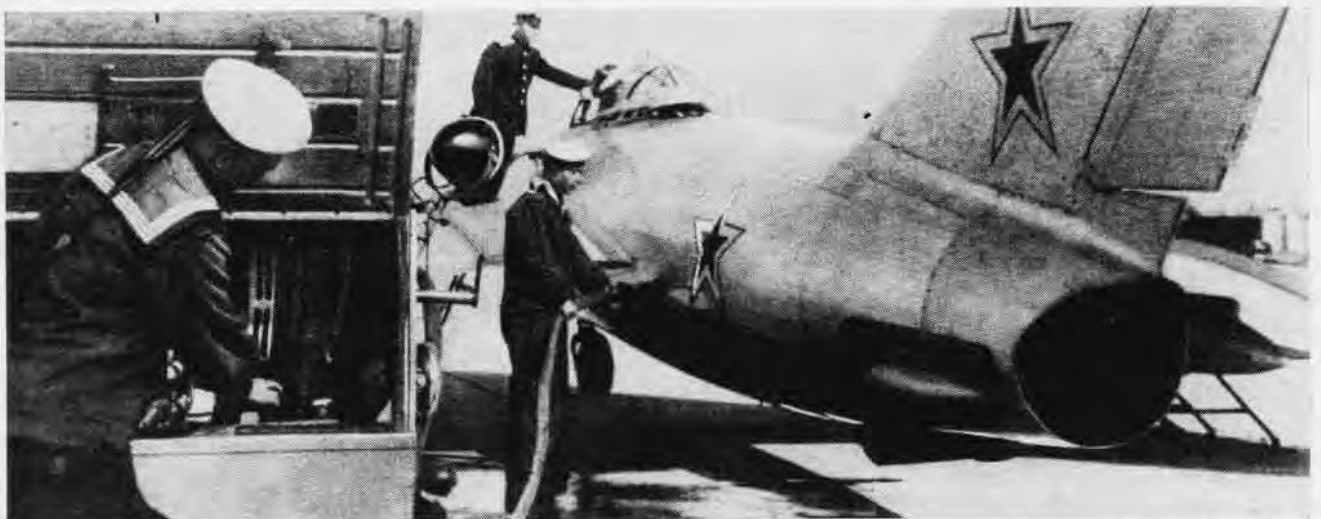
IT IS INTERESTING to see enlisted men wearing formal dress blues as they service a fighter aircraft. While they fuel the Fresco, a Soviet naval officer is checking out the pilot in the cockpit. Note especially the dive brakes located on either side of the tail pipe.
