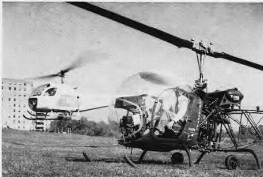
BELL AIRCRAFT'S helicopter division recently demonstrated a new approach to the design of rotor hubs for choppers. Snow White (1), a commercial 47-G series, utilizes stabilizer bars on the rotor hub while the new design in the foreground does not. Removal of the stabilizer bars reduces cost and eases maintenance. Bart Kelly, chief helicopter engineer, pilots test version.
