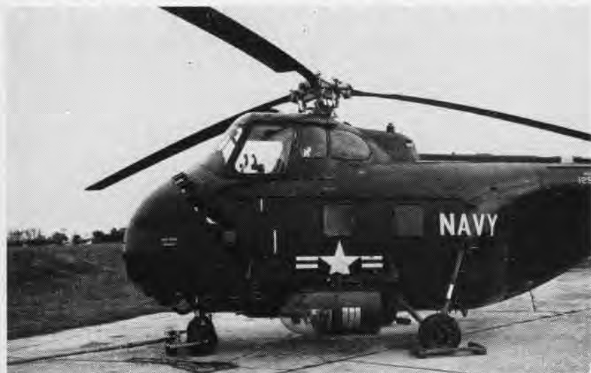
SEARCHLIGHT MOUNTED ON HELICOPTER IS DESIGNED TO EXPEDITE NIGHT RESCUES
