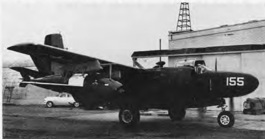
NAVY JD-1 WITH FIREBEE SLUNG UNDER WING, REVS UP FOR TAKE-OFF AND LAUNCHING
