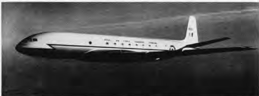
THE FIRST de Havilland Comet II for service with the RAF Transport Command is flight-tested before delivery. Squadron No. 216 will be fully equipped with the jet-powered transport by mid-1957. Power plants for the Comet II are four Rolls-Royce Avon 117 engines of 7,300 lbs. thrust each.
