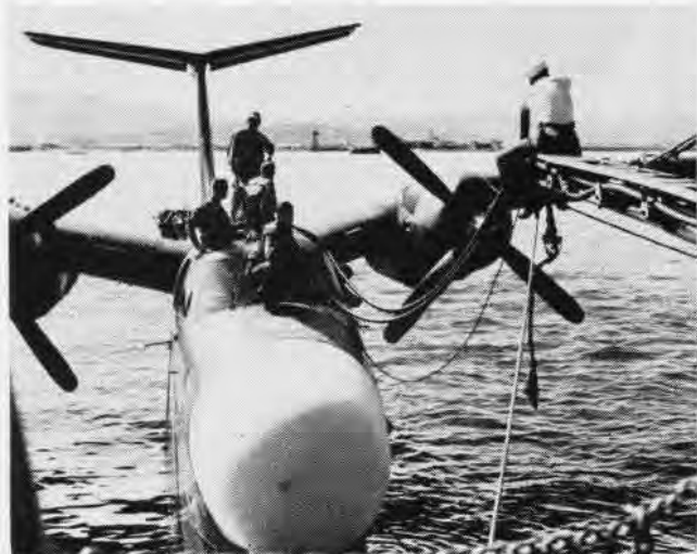
PRESSURE FUELING PUTS IN 3000 GALLONS OF GAS IN SIX MINUTES
