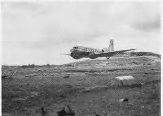
LOW-FLYING R4D makes first of four passes over the 4,000-foot strip to discharge cargo. Old tires mark centerline of target drop area.
