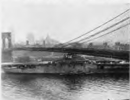
WITH MAST and radar removed, the USS Leyte manages to "squeeze" under Brooklyn Bridge on her trip to the Navy Yard for a routine overhaul. Three tugs assisted in the move.
