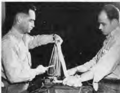
NOT SPAGHETTI but shroud lines being stowed into the parachute pack by the riggers.
