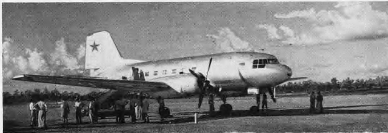
CRATE, THE IL-14 TRANSPORT, IS POWERED BY TWO RADIAL ENGINES, APPROXIMATE LENGTH 70', SPAN 101', CRUISES 250 MPH.
