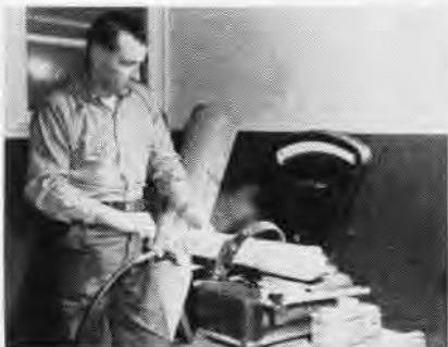
L. FARRIS, PR1, replenishes life raft inflation bottle with a supply of carbon dioxide.
