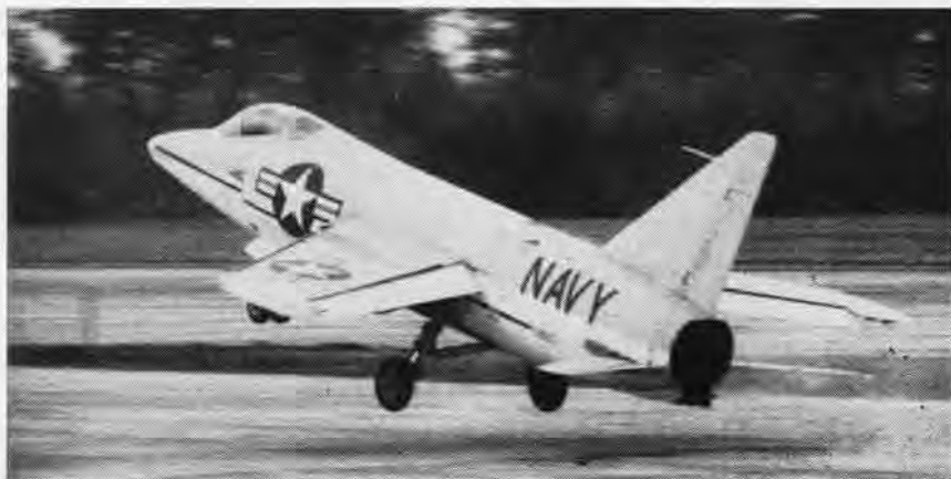
THE XC-7 STEAM catapult at Naval Air Test Center, Patuxent River, gets a work-out as the Navy's F11F-1 is launched for tests. The Tigerjet in all its production models is powered with a J-65 Sapphire turbojet with afterburner. It will be the latest Grumman plane to join the Fleet.
