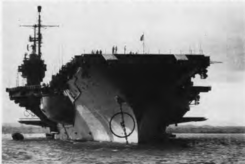
WHILE THE GIANT USS Forrestal lay at anchor in Guantanamo Bay, Cuba, a seaman was lowered away to paint the anchor chain (see circle). This unusual photograph shows a good comparison between the size of the seaman and a massive 360-lb. link in the ship's anchor chain.
