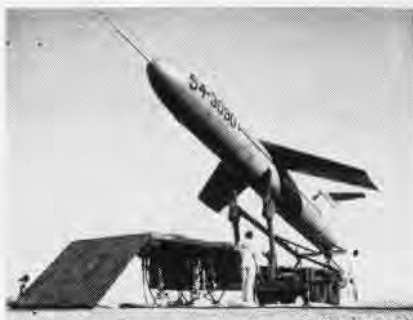
A TEST VEHICLE of a new version of Martin's Matador is ready for test firing at Air Research Development Center, Holloman AFB, New Mexico. For tactical missions, TM-61B will have a new electronic guidance system.
