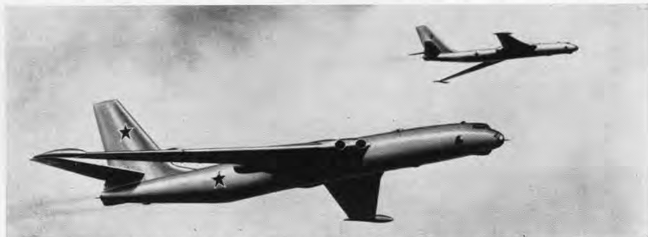
THE BISON BOMBER IS POWERED BY FOUR TURBOJET ENGINES, HAS AN APPROXIMATE SPEED OF 550 MPH; LENGTH 158', SPAN 175'
