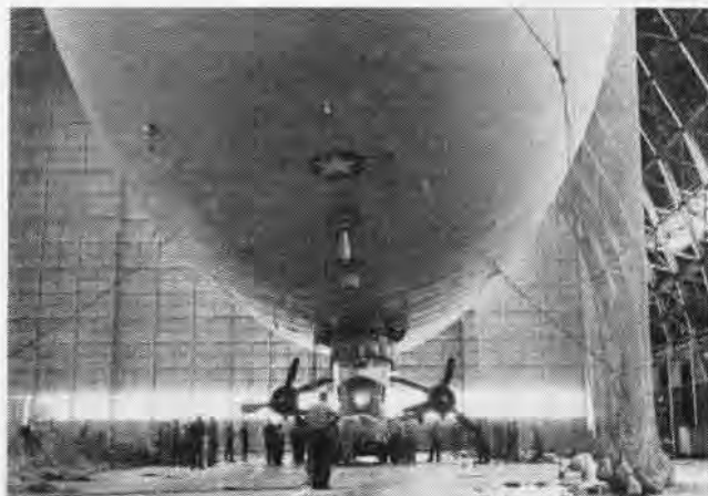
FINAL STEP in preparing the airfoil for flight is the attachment of the gondola. The envelope is held in place by a weighed net.
