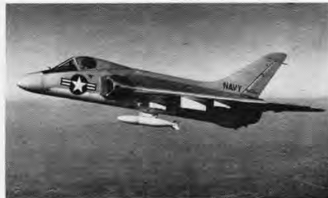
F4D SKYRAY IS POWERED BY A P&W J-57 WITH AFTERBURNER
