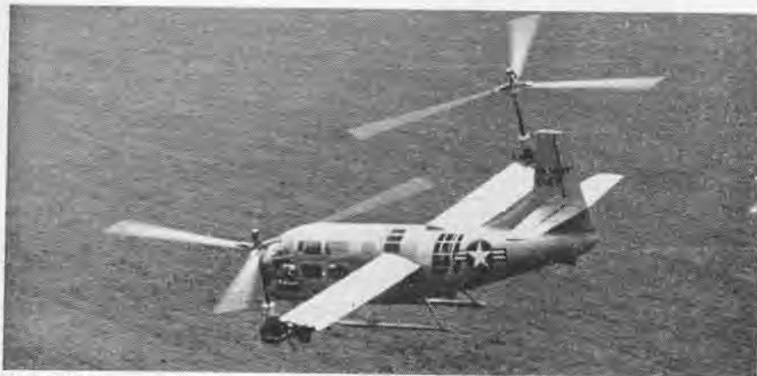
BELL XV-3 Convertiplane has made up to 15 degrees forward rotor mast angle conversions in flight during phase 1 flight tests at Bell's Texas plant. Evaluation flights in helicopter configuration indicate that low power settings will be required in forward flight up to 80 knots. The Convertiplane's vibration level is very low because of flexible rotor mountings.
