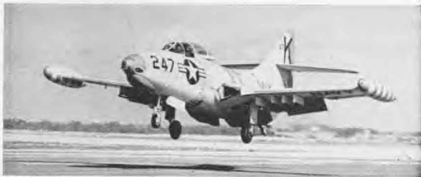
THIS PANTHER was the first aircraft to make a landing on the new NAAS Kingsville, Texas, runway. The 8,000-foot runway is constructed of caliche and asphalt and is 25 inches deep. The strip was completed in June, but the actual opening and first landing was on 18 July. Cdr. C. A. Crow, Jr., Officer-in-Charge of ATU-202, was at the controls of the Grumman F9F-6.
