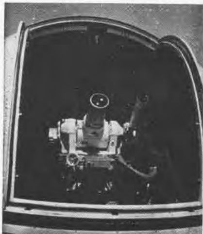
THIS IS AN ASKANIA CAMERA THAT FILMED THE SPEEDING CRUSADER, ABOVE, AS IT FLASHED OVER THE 15.1 KILOMETER RUN
