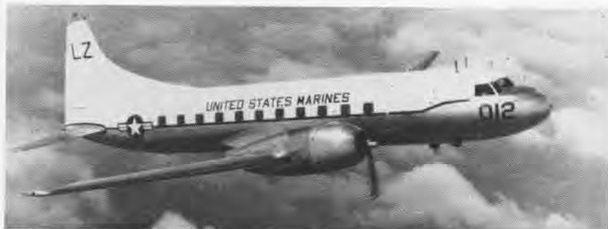
LATEST ADDITION to Marine Corps flying team is the Convair R4Y-1, a twin-engine, cargo-type plane. A rapid rate of climb, and the plane's ability to fly higher and carry more weight in proportion to its size are some of the chief advantages the aircraft has over similar types in use by the Marine Corps. The R4Y can carry 44 passengers with top speed of about 260 mph.
