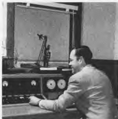
A TEST OF ANTENNA ON A MODEL REGULUS
