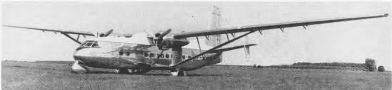
● HUREL-DUBOIS MODEL 32 WITH TWO P&W ENGINES AND HIGH ASPECT RATIO WING IS ON ORDER FOR THE FRENCH NAVY ●
