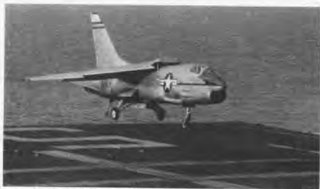
CHANCE VOUGHT F8U-1 Crusader exhibits its two-incidence wing during landing on USS Forrester. It exceeds sonic speed flying level.
