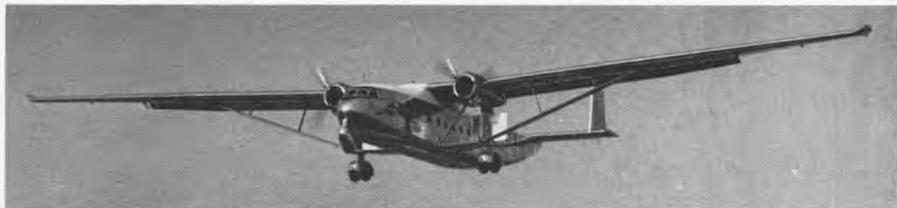
● THIS IS A PROTOTYPE DESIGN WHICH IS DESIGNED FOR NAVAL RECONNAISSANCE; IT CAN LAND ON SHORT FIELDS ●
