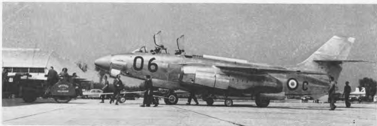
● S.O. VAUTOUR, A BOMBING, ALL-WEATHER FIGHTER FOR TACTICAL SUPPORT, EXCEEDED MACH 1 IN PROTOTYPE MODEL ●
