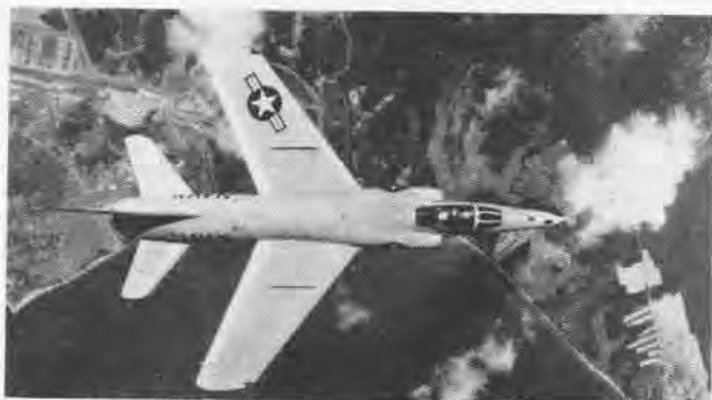
GRUMMAN F11F-1 Tiger was the first plane to have area rule used in its design from the first planning. Note the wasplike fuselage.
