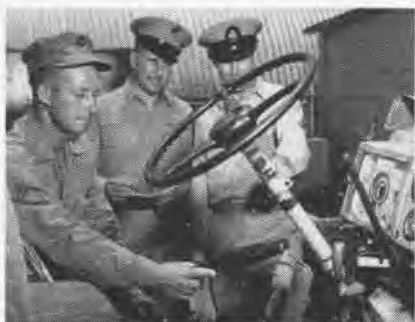
TSGT. C. J. PERRY (L), MSGt. P. J. Hillock , and Cbief H. A. Simmons (R) examine safety features on VMP-533 starting mule. Extension cord extends distance between plane and vehicle. Clutch is of non-slip variety.
