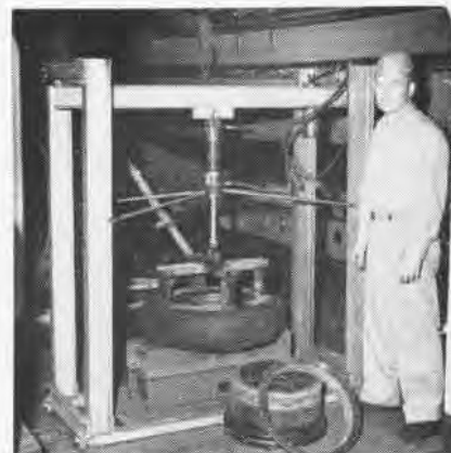
CHIEF AVIATION Metalsmith L. E. Summers, aboard USS Intrepid, built this machine to break the tire from its rim in two minutes. This task formerly took 30 minutes.
