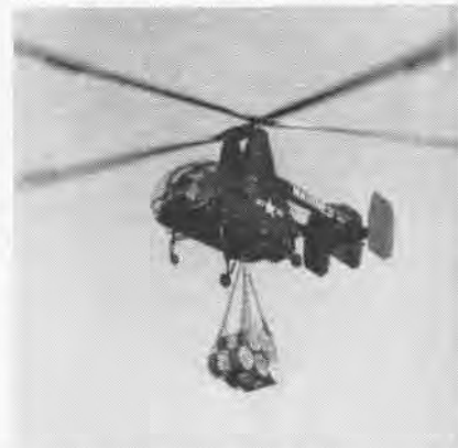
THE MARINE CORPS' HOK-1 plays the part of a "skybook" in this demonstration of lifting ability. The sling releases automatically.
