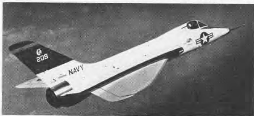
THIS IS the Douglas XF5D Skylancer. It is an all-weather, carrier-based, high altitude performer, with a wafer thin, modified delta wing which takes back from a long, slim fuselage. Complete performance data on the Skylancer has not been revealed, but general flight characteristics were described as excellent. It is powered by an improved model of P&W's J-57.
