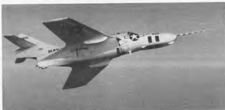
GRUMMAN F9F-8P photographic Cougar sports the so-called fences, or metal strips to interrupt the boundary layer flow toward the wing tips. It is a device to prevent pitchup and tip-stall.
