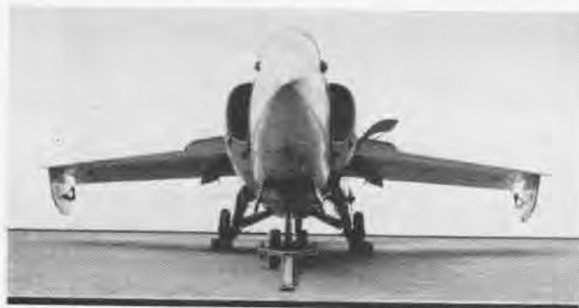
HEAD-ON VIEW of F11F-1 Tiger on deck edge elevator of the Forrester appears like face of monstrous bug. Note the leading edge slats.
