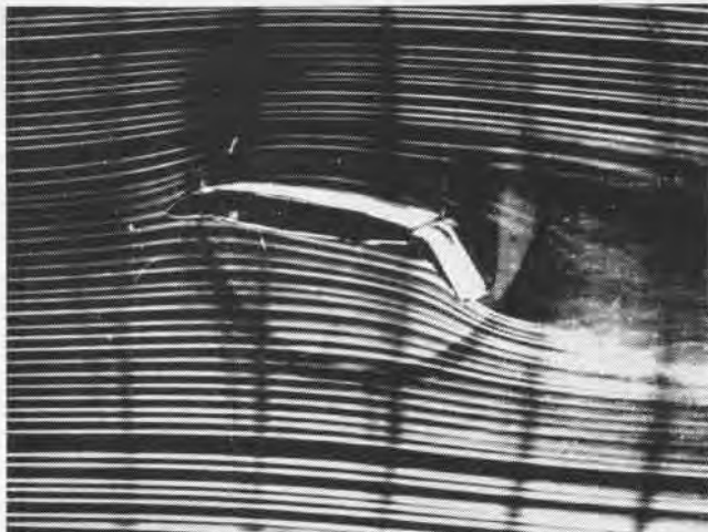
COMPARE FLOW field about airfoil above with that on right, to which Boundary Layer Control has been added. Note turbulence above
