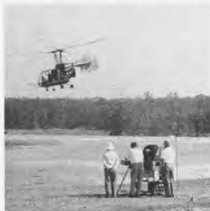
KAMAN ROBOT helicopter is put through paces during a demonstration for DOD officials. Ground control is simple. Safety pilot is in the robot, but he does not fly aircraft.
