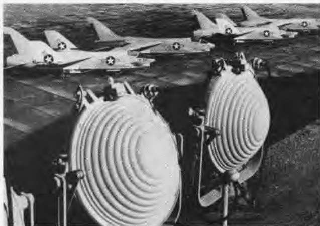
F8U'S FROM FIP program line up on Service Test hangar apron. The two round objects in foreground are searchlights for night flying.
