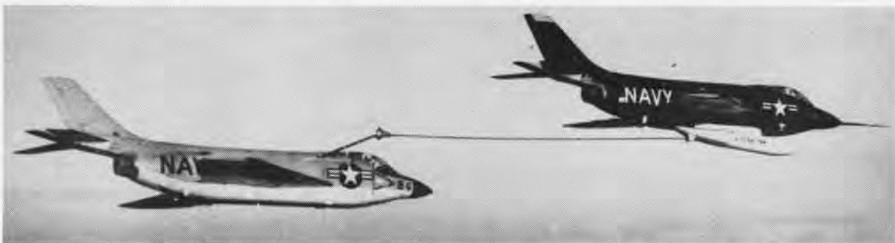
TWO F3H-2N Demons make in-flight refueling contact during experiments near St. Louis. Developed by Beech Aircraft for McDonnell, the system enables a fast jet fighter to draw fuel from a plane of
