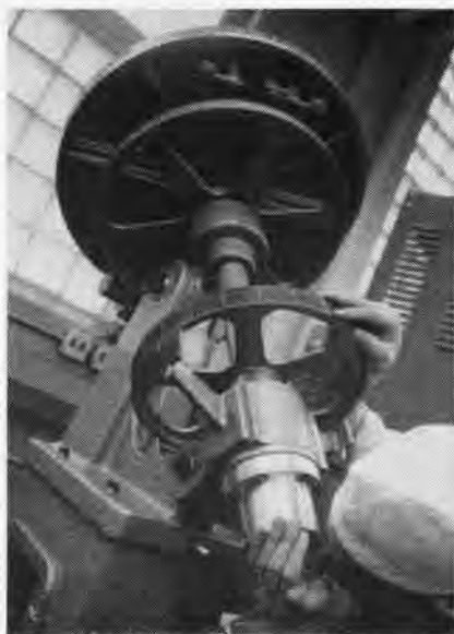
SIDEREAL equatorial mount, developed by Minneapolis-Honeywell, reportedly will use the stationary North Star as a reference point in guiding missiles and rockets to targets.
