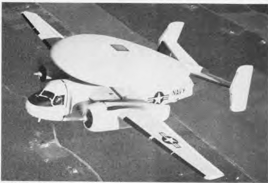
AT FIRST GLANCE, this looks like it should be smothering a steak, but it is a WF-2, named Tracer , Grumman Aircraft's entry in the field of Early Warning. The contrivance looking somewhat like a mushroom houses the antennae and other electronic gear for aircraft's mission.
