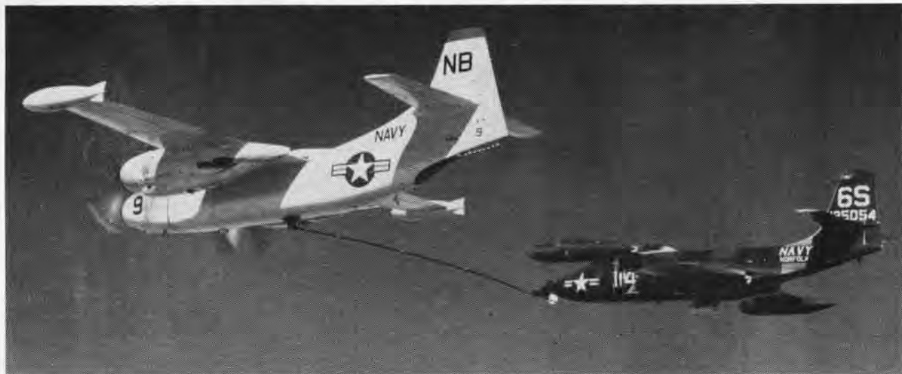
A NORFOLK F2H Banshee gets its "trimony" filled from an AJ Savage during Operation Gashose. Deployed to NAS Sanford for a weekend, VF-861 qualified its members in the "probe and drogue" method of in-flight refueling. The training exercise was flown with VAH-5.
