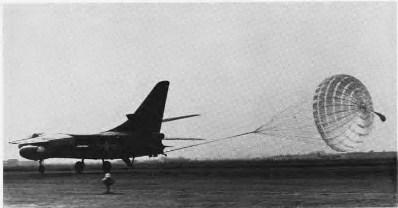
TO HALT THE POWERFUL A3D SKYWARRIOR AS IT COMES IN TO LAND, A STURDY DROGUE PARACHUTE IS FOUND TO BE HELPFUL
