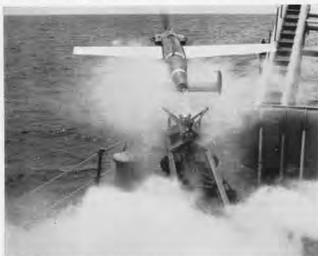
DOWN THE 30-FOOT RUNWAY GOES TARGET DRONE AT 200 MPH
