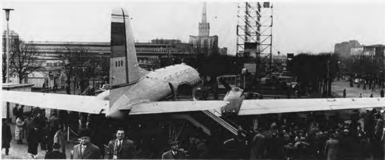
THE RUSSIAN CRATE was shown at the Leipzig Fair with its East German markings. The Crate is a twin-engine development of the Coach
