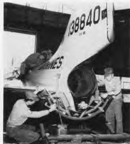
ENTIRE TAIL section of an F9F Cougar jet is removed to provide access to jet engine.
