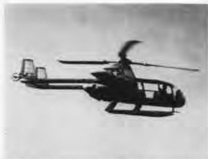
HIGH SPEED Whirlybird, the McDonnell XV-1 attains 200 mph. Development of new vertical take-off convertiplane is being sponsored by the Army, administered by the Air Force.
