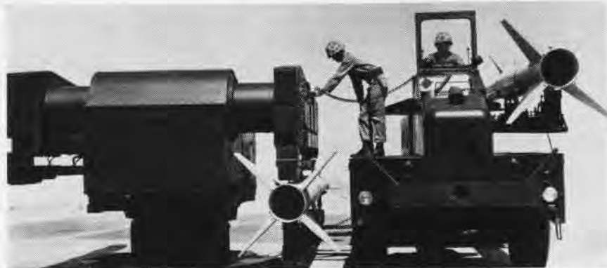
A MARINE CORPS ordnanceman activates a Terrier missile launcher after loading. The missile truck can transport two missiles. After a missile is placed on the launcher, the launcher is pointed continuously by the fire control system so that firing will effectively hit the target.
