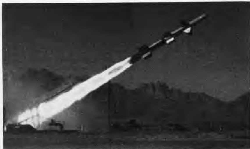
TALOS MISSILE zooms skyward from proving ground to lock onto a target. It is guided by a mechanical brain called a steering intelligence system. When within lethal range, a proximity fuse detonates its warhead. Talos, with nuclear capability, will join the fleet next year as a major armament on the missile cruisers Galveston , Little Rock and Oklahoma City .
