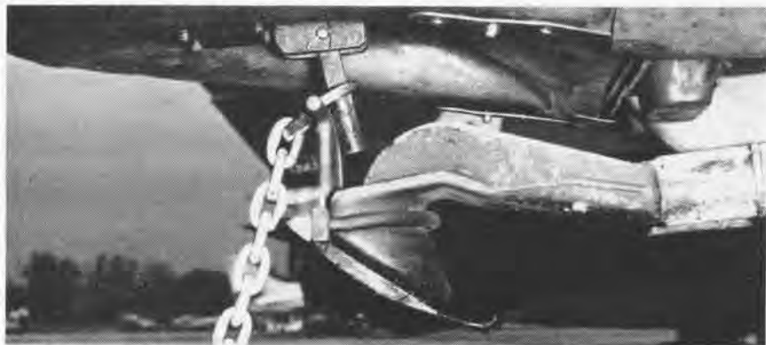
SKYRAY JURY-RIGGED tow-point fitting utilizes tailhook attachment to secure Mk. 8 tow ring, 5/16" chain leader. Described tow rig and banner are recommended for F11F and F3H models.
