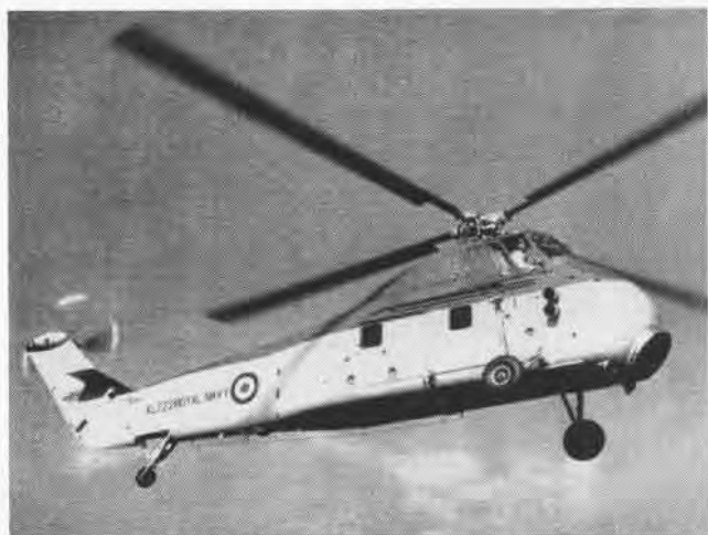
WESSEX IS FIRST PRODUCTION COPTER WITH FREE TURBINE POWER
