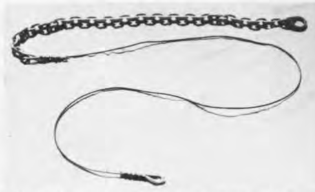
MODEL OF TOW cable rig devised for high speed tow use. Minimum scope of 3500' 3/16" wire cable micropressed to 60' length 5/16" link high carbon chain is recommended. Mk. 8 tow ring is welded to leader.
