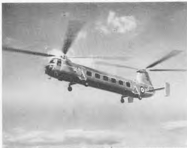
BRISTOL 173 WAS BUILT FOR RESEARCH OF TANDEM-ROTOR DESIGN
