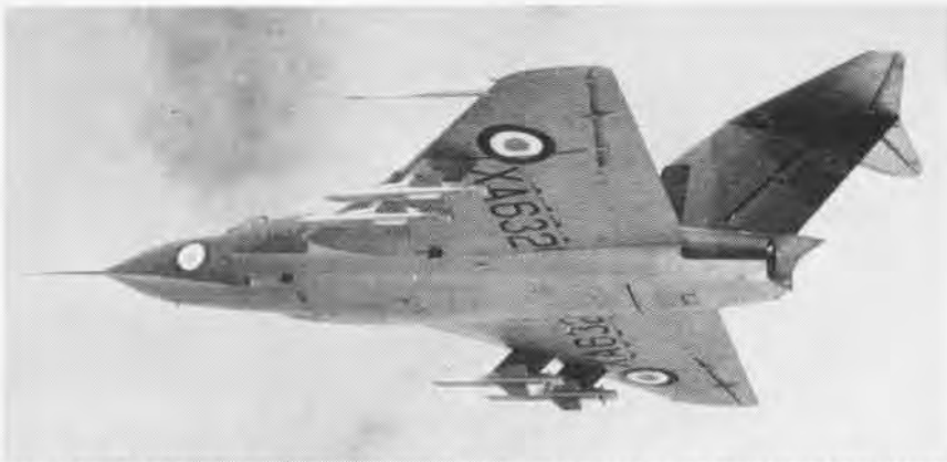
GLOSTER AIRCRAFT'S TWIN JET JAVELIN SHOWN EQUIPPED WITH FIRESTREAK MISSILES
