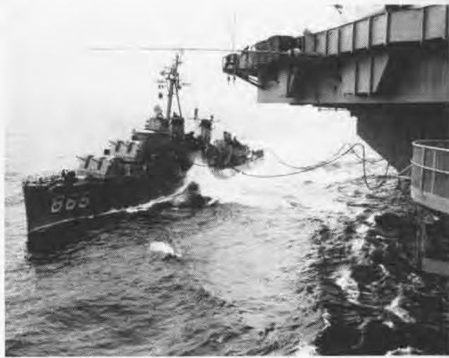
REFUELING WAS an essential part of NATO operations in the North Atlantic. Here USS Ware, DD-865, is refueled alongside the Saratoga.
