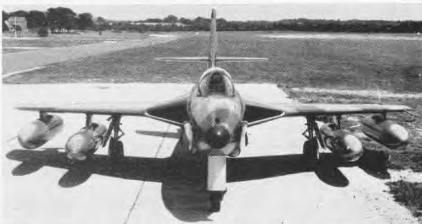
HAWKER HUNTER IS SHOWN WITH AUXILIARY, DISPOSABLE FUEL TANKS HUNG ON WINGS
