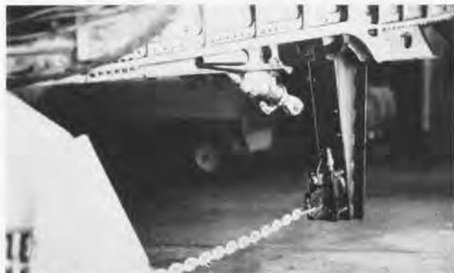
CRUSADER TOW mast , jury-rigged by Armament Test technicians, is attached to F8U-1 catapult fitting. Steel mast has Aero 1A Douglas ejector bomb rack hook for tow; F8U electrical power source for release.
