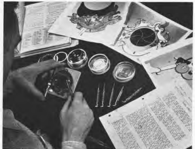
TRAINEE OVERHAULS A GRAPHEX SHUTTER USING TRAINING AIDS
