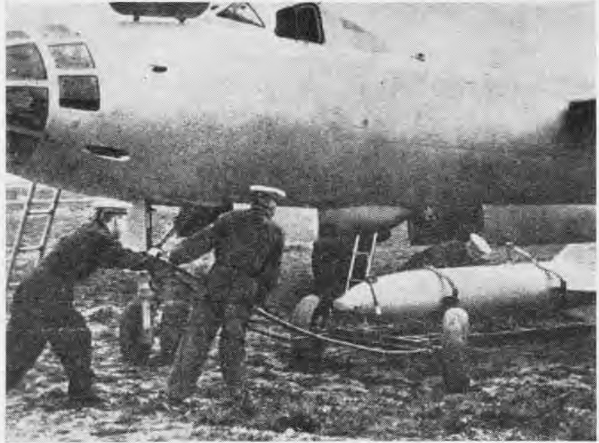
HERE SOVIET NAVY ENLISTED MEN INSTALL A 1000-POUND BOMB ON BEAGLE AIRCRAFT
