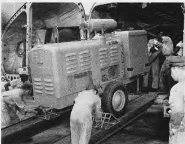
UNLOADING the power unit must be done meticulously and brakes are used as the unit comes down when handlers signal a need to slow it.
