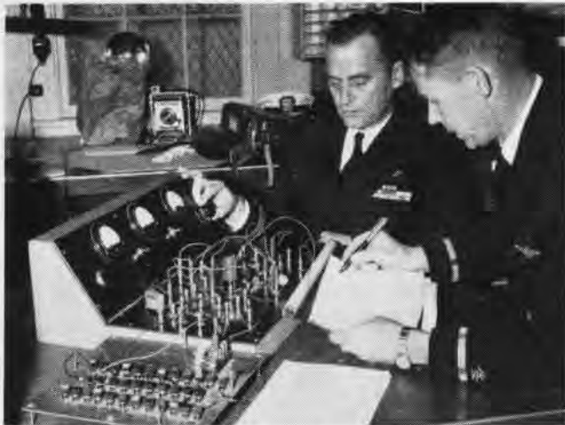
KUBE AND GUSTAFSON work out the design for a new electronic component on a "bread board" which they built to speed development.
