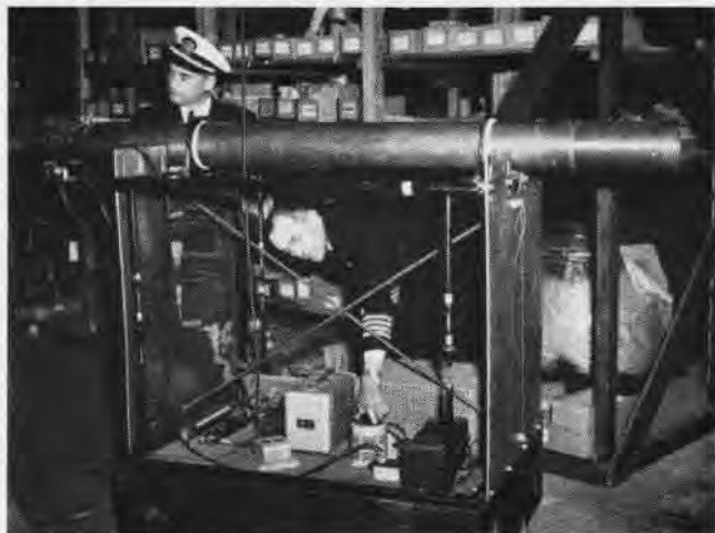
THE LIGHT GUN which projects impulses to "light bucket" across the field at NAS Anacostia is calibrated by Capt. Barr and Ltjg. Kube.
