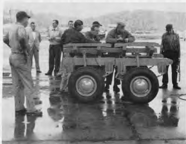
THIS GIVES an excellent view of one of the dollies. Here it is folded up so that it can be carried in the space for it on the R4Q.
