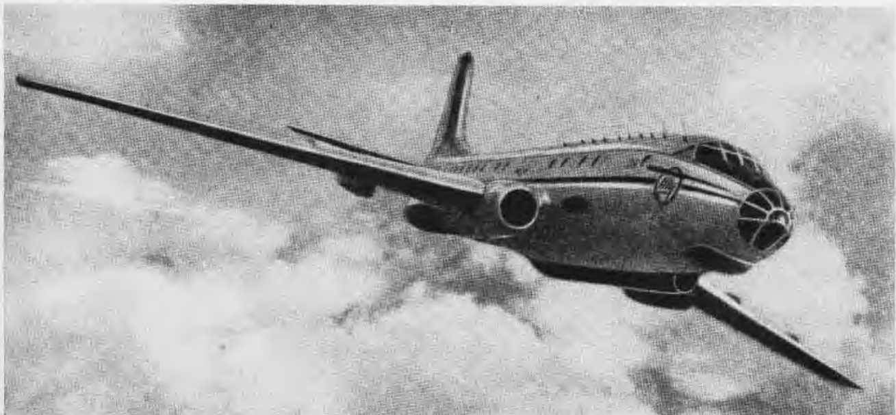
THE CAMEL (TU-104) IS A TWIN JET TRANSPORT VERSION OF THE BADGER BOMBER WITH THE SAME WINGS, NOSE, TAIL AND ENGINES
