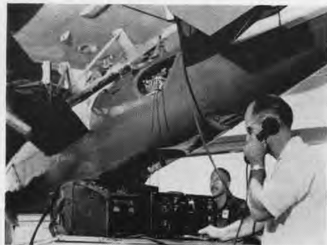
JUST BEFORE a Firebee mission, the autopilot system is given a complete functional check while drone is attached to the parent aircraft.
