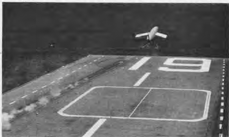
A REGULUS MISSILE IS LAUNCHED FROM THE USS HANCOCK, AIDED BY STEAM CATAPULT
