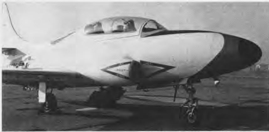
LATEST ADDITION to the Navy's jet instrument training program is the T2V. It will supplement the TV-2, now in service, with the first deliveries set for early 1957. The plane above was used as part of an instrument evaluation program at Moffett Field. Greatly improved low speed stability is provided by a boundary layer control system. It is equipped for carrier operation.
