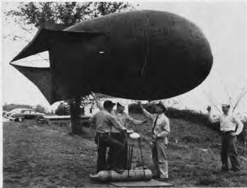
A KITE-BALLOON , used as a target to study visibility range problems, is readied for launching by Chief Ledbetter and his crew. Balloons in various shades are used.
