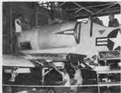
O&R DISMANTLES A4D FOR PILOT OVERHAUL
