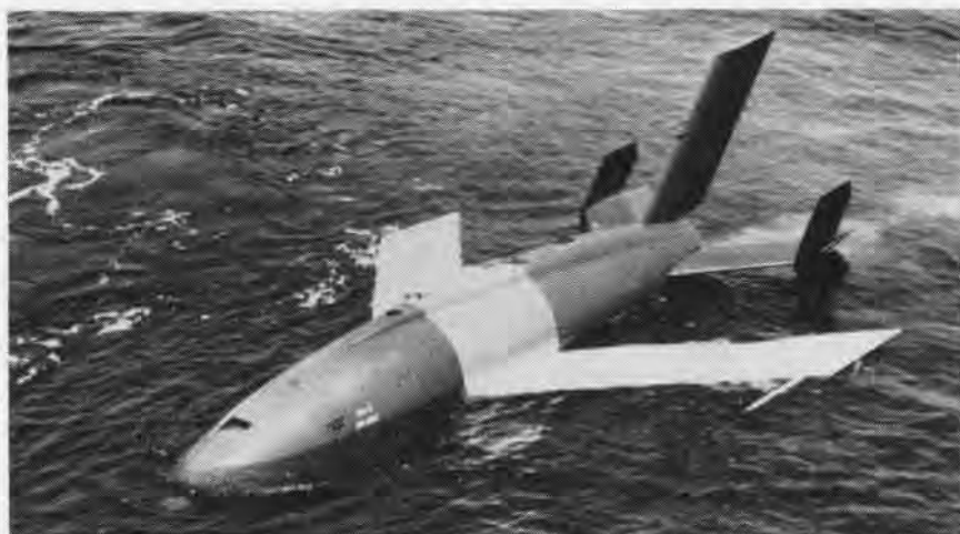
SINCE THE NAVY KDA-1 version of the Firebee will see extensive use over water, special flotation devices were incorporated in this model to insure recovery after parachuting into sea.
