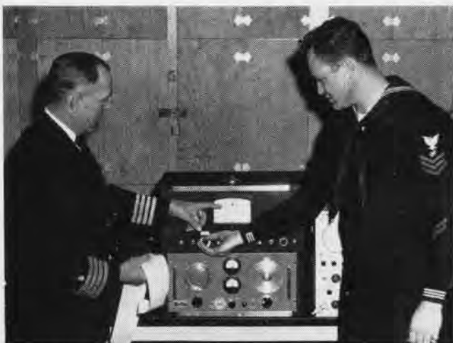
CAPT. BARR and Sikes observe the pulse rate and electrocardiogram on a subject who is doing his regular work at a remote location.
