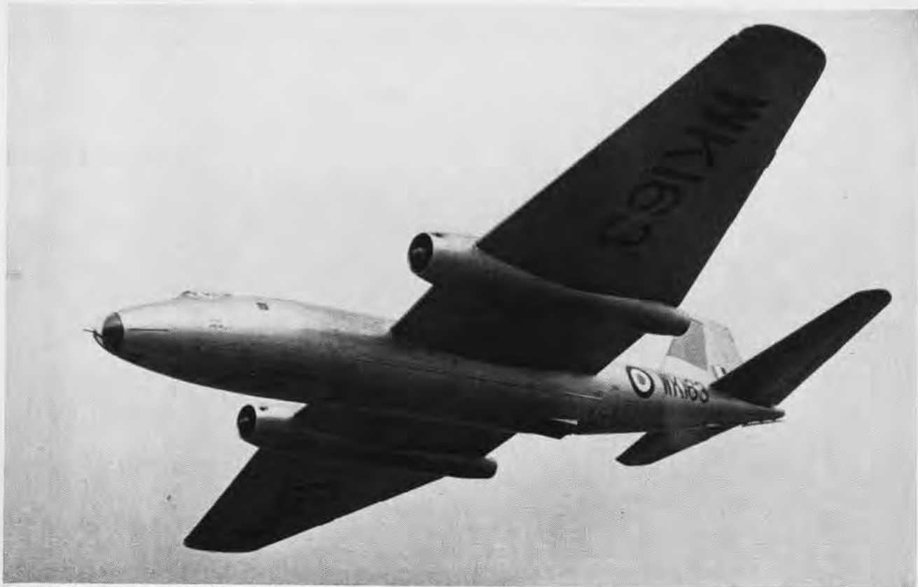
ELECTRIC'S CANBERRA HAS BEEN CONVERTED INTO A FLYING TEST BED FOR THE NAPIER SCORPION AIRCRAFT ROCKET ENGINE
