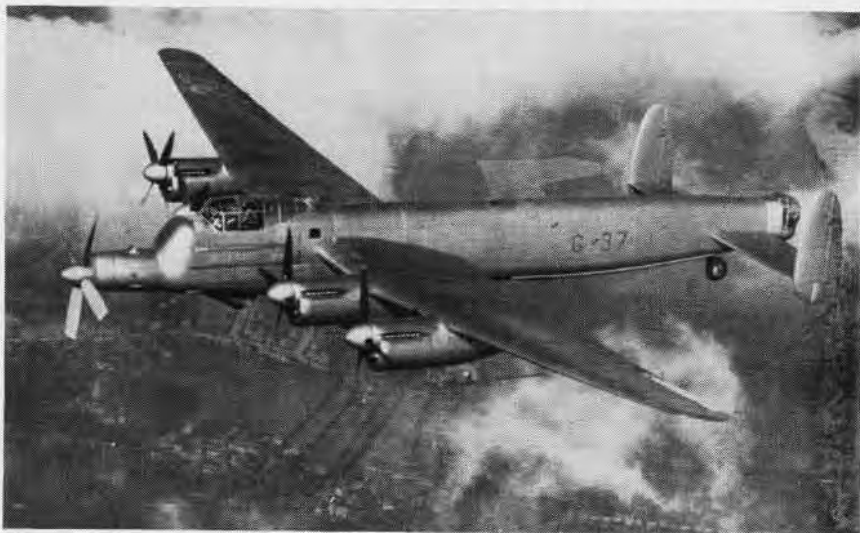
TYNE TURBOPROP, MOUNTED IN NOSE OF A LINCOLN TEST BED, DEVELOPS 4470 EHP
