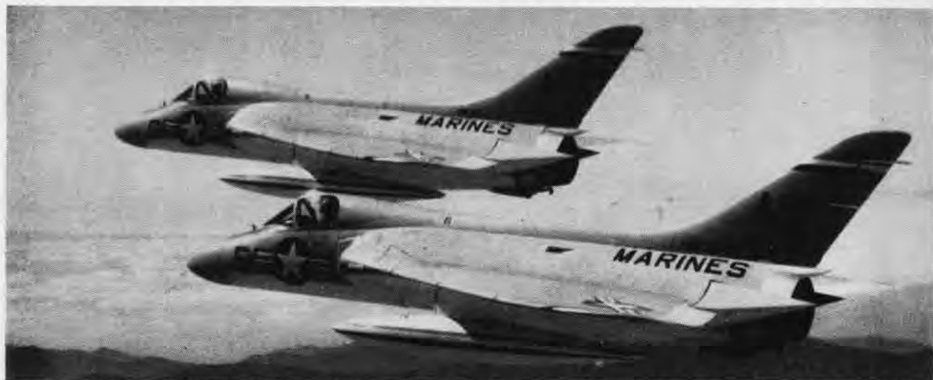
TWO OF VMF-115'S SKYRAYS PRACTICE FORMATION FLIGHT OVER THE MOJAVE DESERT. F4D'S GROSS WEIGHT IS 19,000 POUNDS
