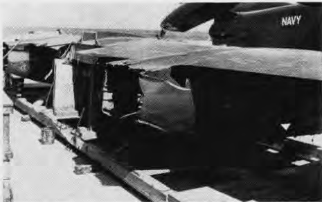
THOUGH THE wing assembly received relatively little damage, the entire wiring system, about seven miles of wire, had to be replaced.
