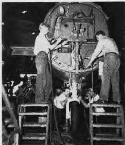
SOME MINOR alterations were necessary to get a perfect fit of the two grafted sections.
