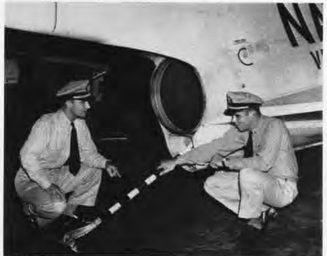
VITAL IMPORTANCE of the F9F-8P tailhook which helps arrest forward thrust of several tons of bucking airplane is emphasized by Clark.
