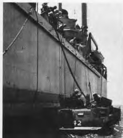
LVT (LANDING vehicle, tracked) gets gas supply, first step of USMC bulk fuel system.
