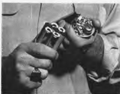
A MINITRACK transmitter and battery pack which will be installed inside each satellite.
