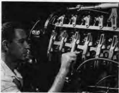
A TECHNICIAN ADJUSTS VARIABLE STATOR
