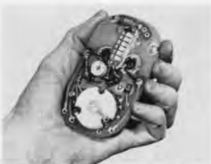
A COMPLETELY transistORIZED UHF Beacon Transmitter the size of a standard sardine can has been announced by Fairchild Controls Corporation. It can send radio signals continuously for 25 miles for a period of 24 hours.
