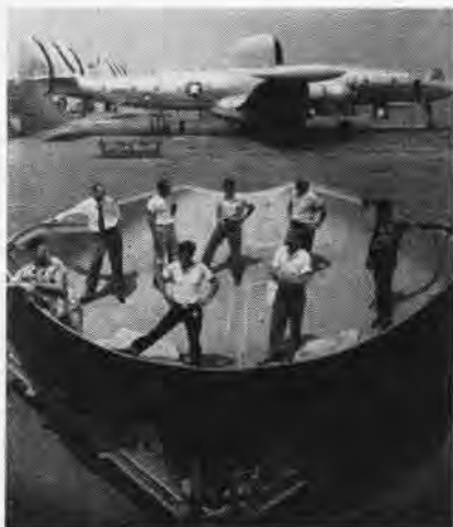
RUB-A-DUB-DUB , eight men in a tub! This is a "swimming-pool-sized" lower radome for a WV-2 Early Warning Constellation. The radar it houses can detect distant planes and ships.
