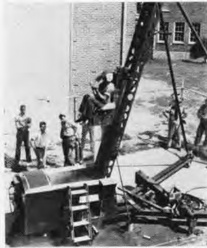
ACCELERATION testing unit of the center investigates the problems of seat ejection.
