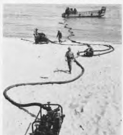
NAVY LANDING craft, vehicle-personnel, hooks up fuel lines to a beach unloading station.
