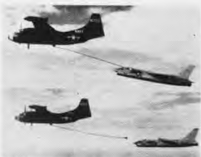
A NEW VALUE of the variable incidence wing of the F8U Crusader is demonstrated during refueling. At bottom is shown how a pilot can fly flat, staying behind the tanker instead of mushing as shown in the top picture.
