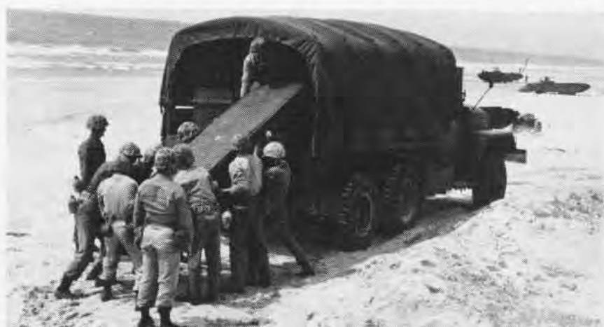
MARINE FUEL TEAM unloads aluminum chest which contains 10,000-gallon capacity collapsible bulk fuel tank. The LVT will pump contents of its 850-gallon tank into this container.
