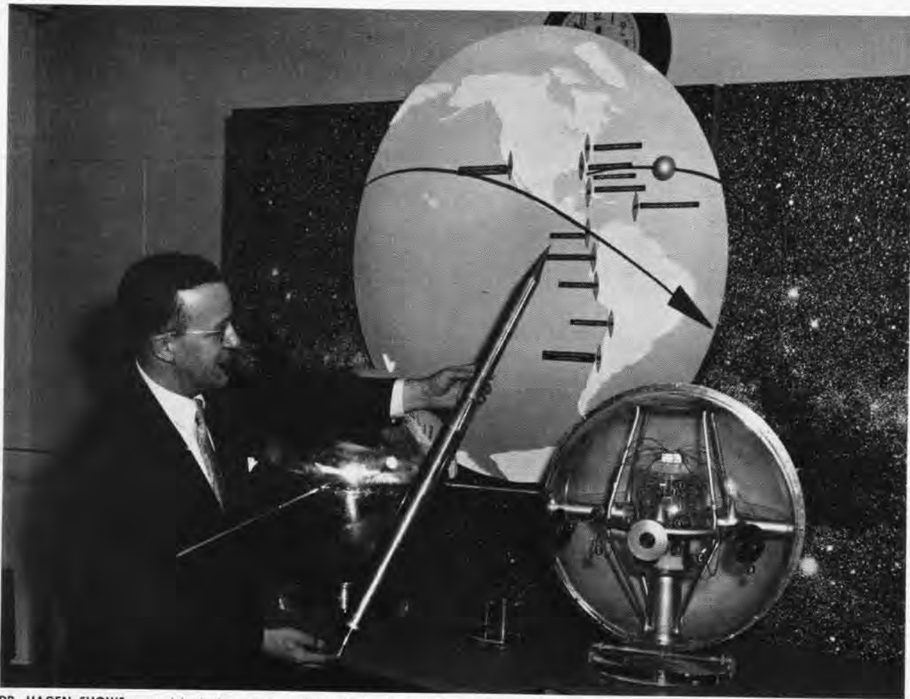
DR. HAGEN SHOWS a model of three-stage rocket which will propel the satellite into the earth's upper atmosphere and put it in its orbital path. Arrow shows probable orbit of the "moon" and the markers designate locations of the various radio tracking stations.
