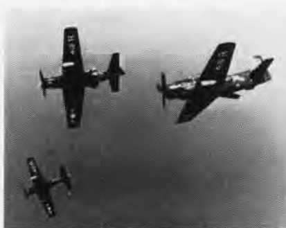
DIVE BRAKES VISIBLE ON THE EARLY AD-3'S
