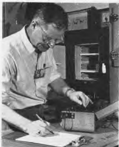
TESTS ARE made of erosion gage which will record effect of particles on "moon's" skin.
