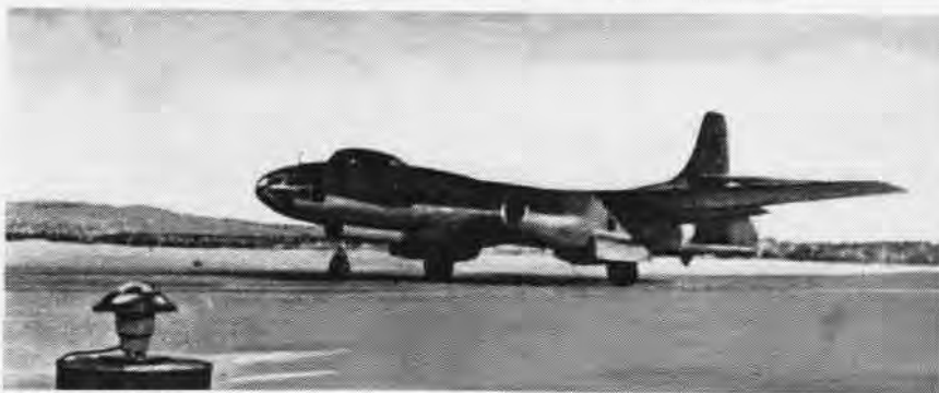
THESE PICTURES of the Bosun, an aircraft used by Soviet naval aviation, reveal a smooth high tailed configuration. Its performance is similar to the Beagle, another USSR Navy plane. The twin jet Bosun has a long, sleek fuselage, armament in the tail and a radome under the fuselage. In an article describing the Bosun and its crew, the Soviet reporter stated that the flyers "steadfastly work in the severe conditions of the north" and thereby "increase their flying mastery."
