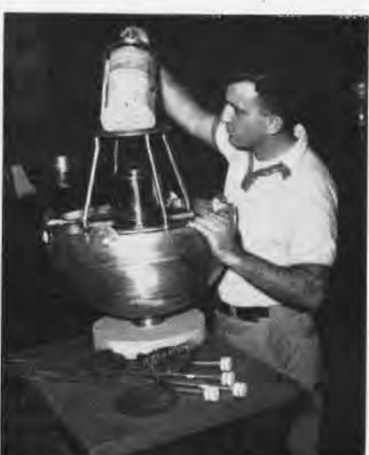
PLASTIC FOAM-encased electronic package is inserted into gold plated container at NRL.
