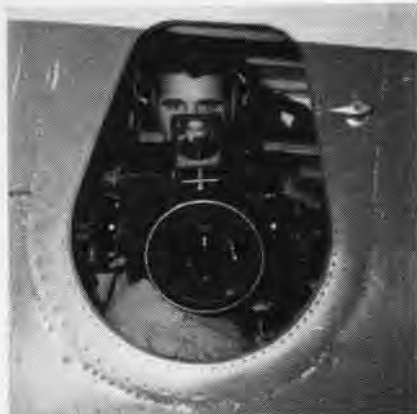
TO TAKE oblique aerial photos, R. Park, PH2, lines up "eyes" of his F-56 aerial camera.
