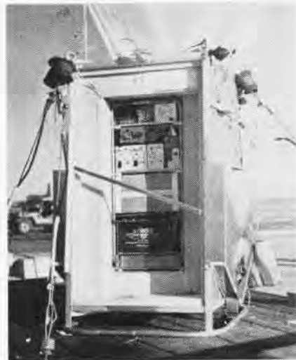
SIX HUNDRED pounds of instrumentation were carried to record and transmit weather data.
