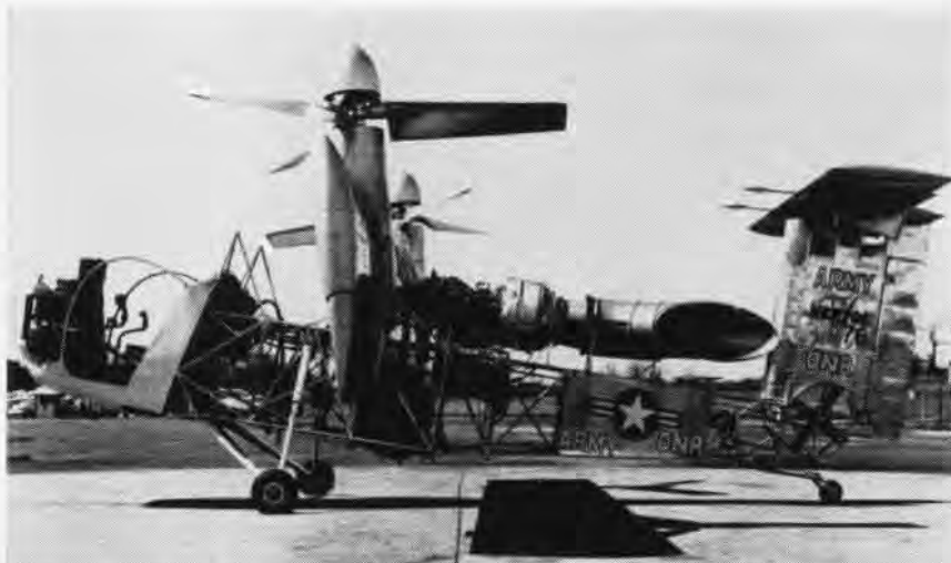
THE FIRST TILT-WING VTOL research aircraft is now undergoing functional tests, according to Vertol Aircraft Corporation. The aircraft, funded by the U. S. Army and developed in cooperation with the Office of Naval Research, is powered by a Lycoming T-53 gas turbine engine aft of the cockpit and atop a tubular fuselage structure. Wing and two counter-revolving rotor propellers are tilted as a unit through a 90° arc for vertical take-off and landing or level flight. Conventional airplane controls become effective when the wing is tilted to a horizontal position.
