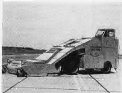
THE FRUEHAUF COLE-VAC AIRFIELD CLEANER
