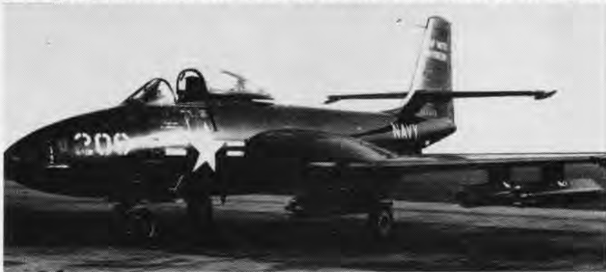
ZUNI ROCKETS IN TRANSPORTABLE LAUNCHERS MOUNTED UNDER WINGS OF JET AIRCRAFT
