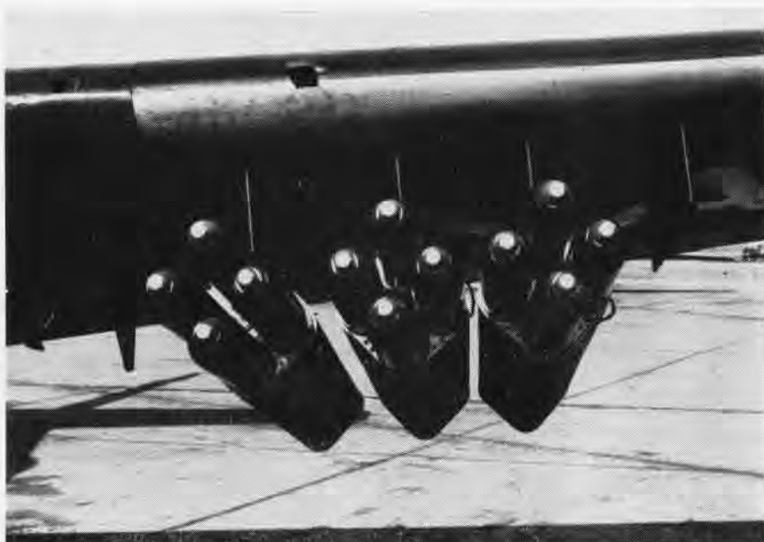
ZUNI'S FOLDING WINGS SUBSTANTIALLY INCREASES THE NUMBER OF ROCKETS CARRIED
