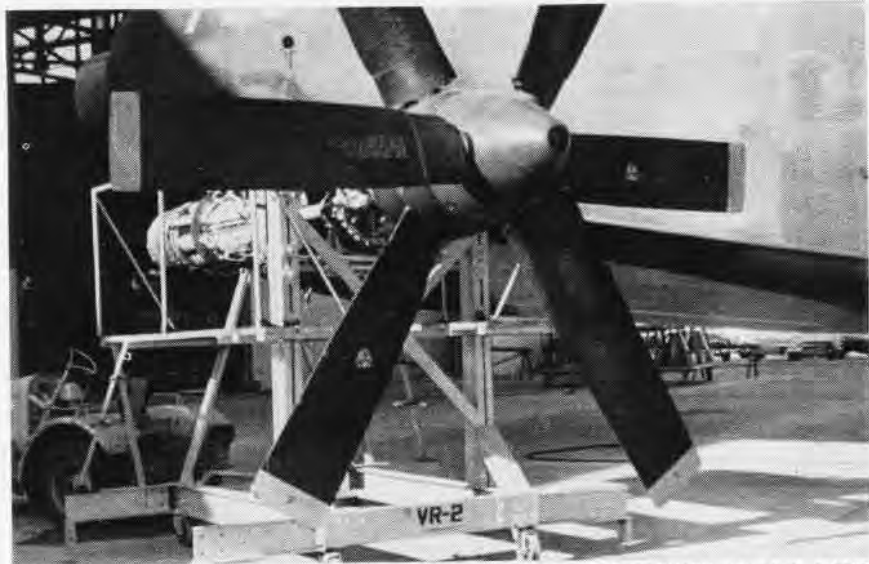
R3Y'S ALLISON T-40 TURBOPROP ENGINE AND PROPELLER ARE SECURED IN THE STAND
