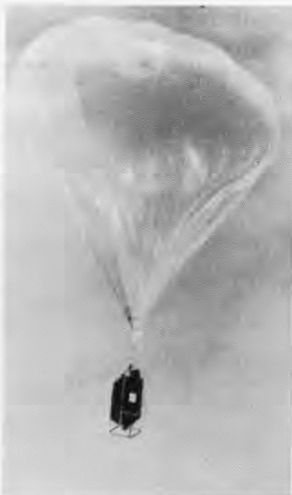
RELEASED , the plastic balloon ascends to a 30,000-foot level and travels with the wind.
