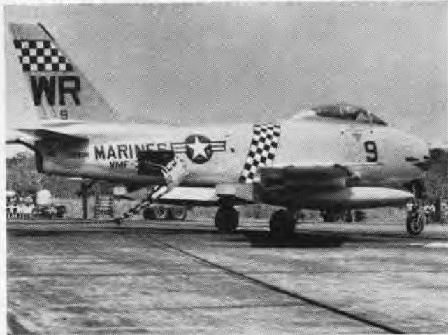
FURY CATCHES 'MOREST' CABLE; WILL COME TO HALT AFTER 310 FEET
