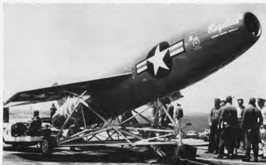
THE REGULUS can be steam-catapulted from the decks of aircraft carriers. This new capability was made possible by a launcher cart which was developed by Chance Vought for the Navy.
