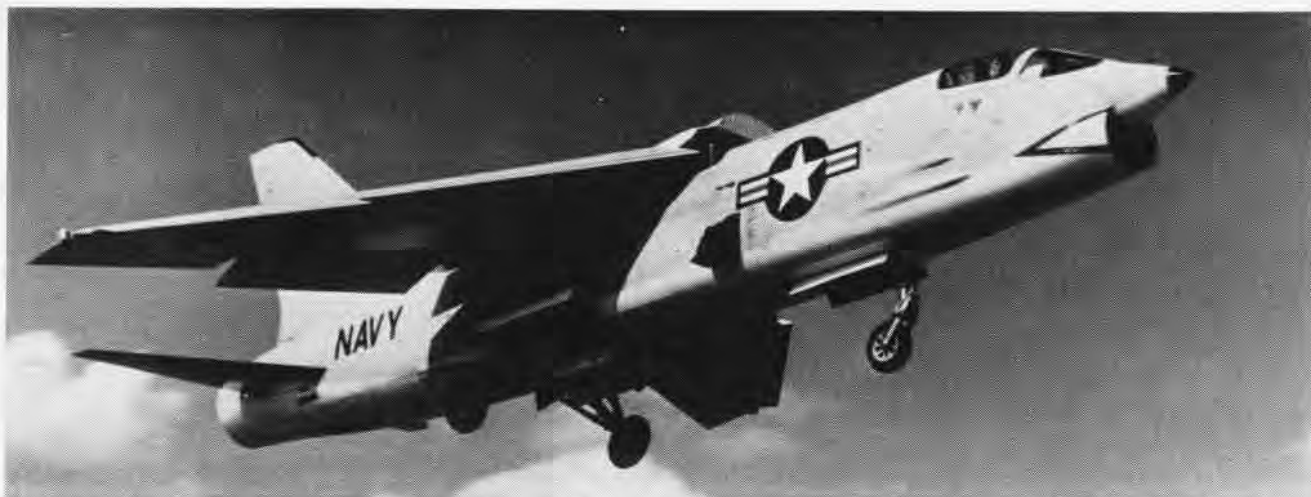
F8U-1 CRUSADER , Chance Vought's number one plane, comes in for a landing with its incidence wing in low-speed position. Black spot on side of fuselage below wing leading edge is a ram air turbine for emergency use should either hydraulic or electrical systems fail.
