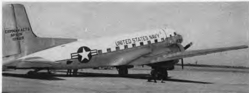
THIS R4D-8 is the only U. S. Navy plane assigned to Spain. It averages 250 flight hours a quarter. Here the "Trolley" waits at the U. S. Naval Station, Rota, for an outgoing cargo.
