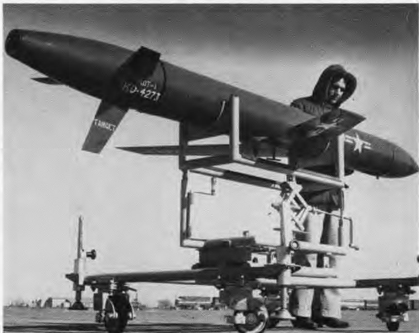
TEMCO'S NEW rocket-powered target drone, the XKDT-1 is about 12 feet long and 10 inches in diameter. The drone is a low-cost, expendable target which can be launched from a carrier-based plane. Top speed of the XKDT-1 is slightly less than Mach 1 at 50,000 feet.
