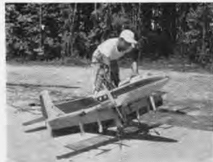
AN NACA scientist checks model of a four-engine VTOL model to be used in stability tests.
