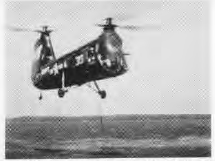
DIPPING sonar gear in play, HUP-2 hovers over surface of water, pinging and listening.
