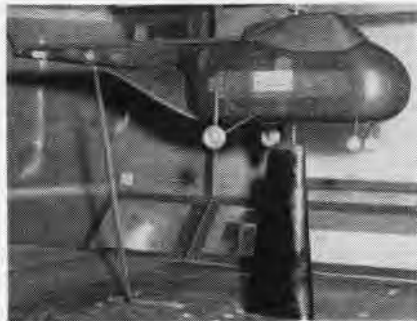
THIS IS a 1/10th scale wind tunnel model which is used to study characteristics of the S-55.
