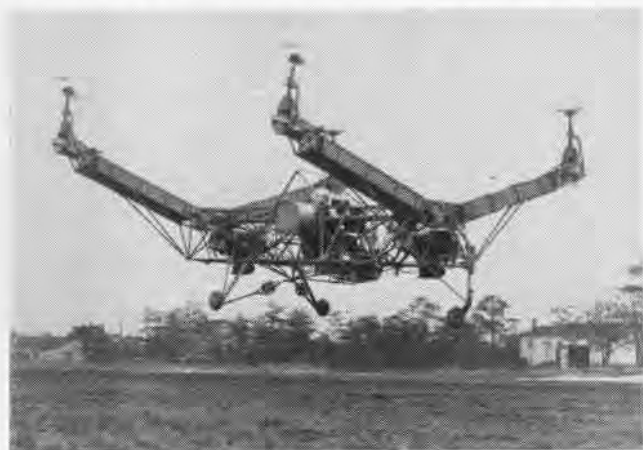
FIRST FLIGHTS of the Quadrotor Flying Test Bed, designed by Convertiplanes, Inc., proved ease of handling and freedom from vibration.
