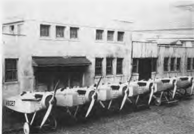
PARKED OUTSIDE an early production building at Long Island City plant, these then modern VE-7's were awaiting engine run-up tests.
