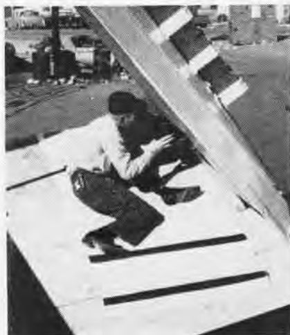
TO PROTECT upper wing of AD during servicing of outboard wing guns, Marvin R. Young, AO1, of VA-145, NAS Miramar, devised a 100x42-inch canvas cover working surface. Strips of wood at one end serve as foot braces.
