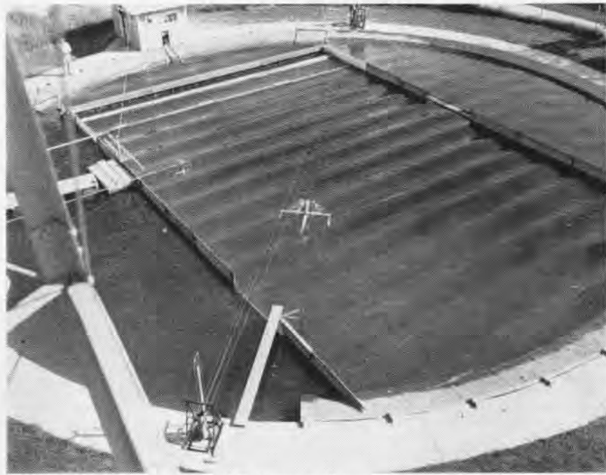
MODEL SEAPLANE being towed at 135 degrees to direction of wave travel. Waves are five feet long, and the height-length ratio is one to twenty. Compare size of man to size of basin.
