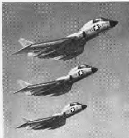
THE TAIL-LESS , swept-wing F7U Cutlass went into production for Navy, early in 1950.
