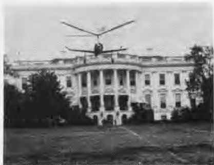
ONE OF the early autogyros, an XOP-1, built by Pitcairn, landed on the White House lawn.
