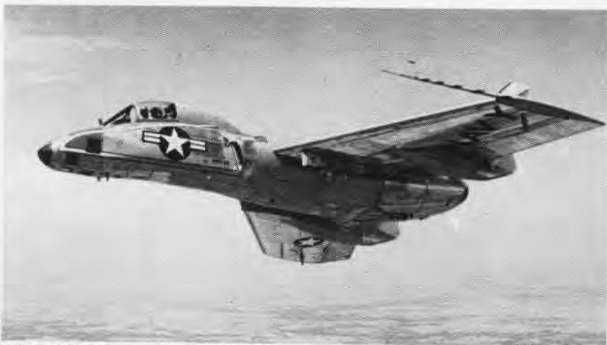
PHOTO VERSION of the F7U-3 Cutlass packs five cameras in its elongated nose. It also carries a large number of flares in the area normally occupied by guns of the fighter version.
