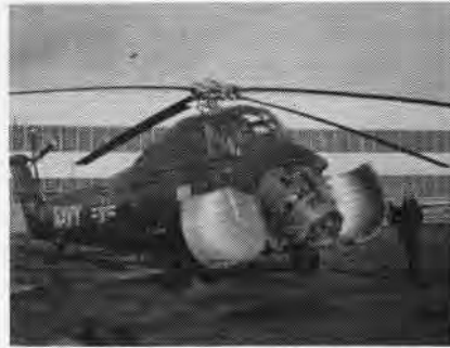
CLAM SHELL doors in this Sikorsky copter are designed to give maximum engine accessibility.
