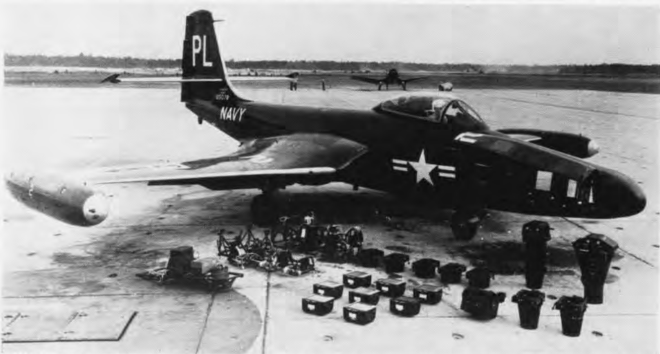
INSTALLED IN THE PHOTO-BANSHEE'S NOSE, THESE AERIAL CAMERAS CAN MAKE DAY OR NIGHT, OBLIQUE OR VERTICAL PHOTOS
