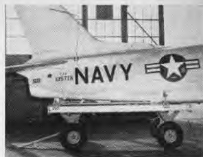
TAIL SECTION on transportation trailer after being rolled from the positioning trailer.
