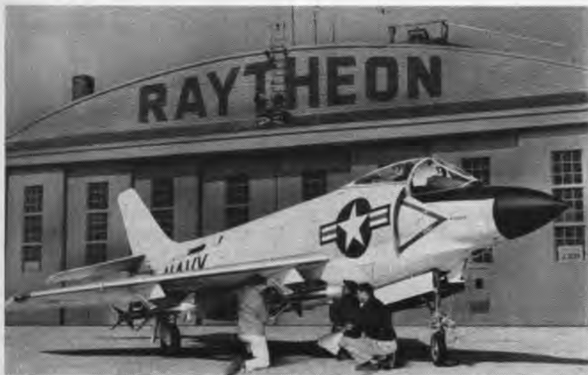
SPARROW III GUIDED missiles are being installed on this F3H-2M. The new missile will augment Sparrow I now in operational use with the Fleet. Sparrow I, a supersonic air-to-air missile, is some 12 feet long, weighs 300 pounds, and goes faster than 1500 mph within seconds after being launched. The Sparrow II is an experimental missile not intended for Fleet use.
