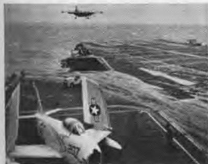
AJ-1 SAVAGE receives a "cut" from the Forrestal's LSO prior to an arrested landing.
