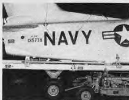
POSITIONING trailer is attached to transport trailer. Adapters hold the tail section.
