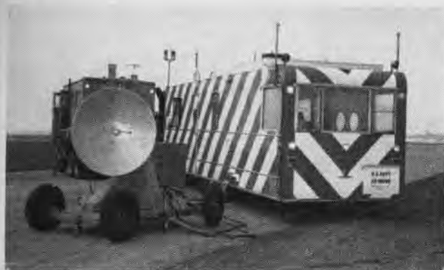
THE NAVY'S automatic carrier landing system, developed and built by Bell Aircraft Corporation, is a combination of radio and radar.
