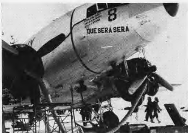
PRE-HEATERS ARE USED TO WARM R4D ENGINES AT MCMURDO STRIP
