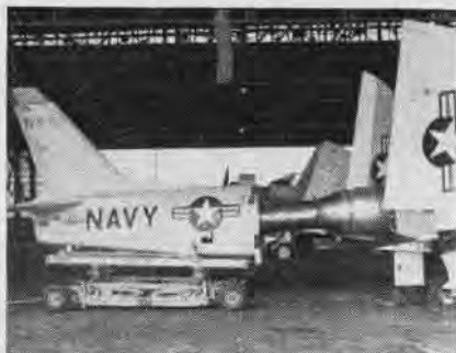
THE POSITIONING trailer is used here to remove tail section of F1 in tests at Patuxent.
