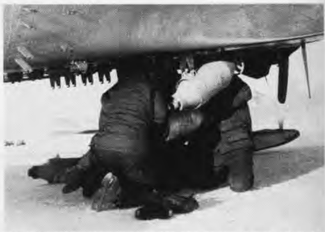
CREWMEN LOAD JATO BOTTLES ON R4D BEFORE PLANE TAKES OFF
