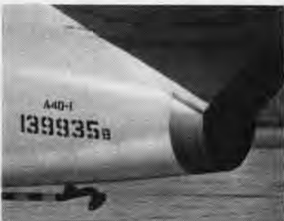
WHAT DOES the "B" stand for after this BuNo? The question was asked of numerous officers who might be likely to know, but didn't. An answer came from BuAer's Maintenance that it signified the plane had received certain necessary modifications and changes.
