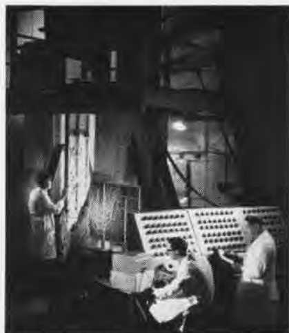
COMET COMPONENTS are being tested in a special fatigue-testing machine designed by de Havilland engineers. It can apply a fatigue load of 100 tons 500 times a minute.
