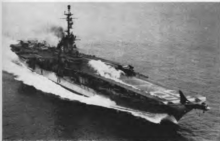
AN A3D SKYWARRIOR takes off from the USS Shangri-La . Although the plane was designed for complete carrier operation, it is still a heavy plane requiring the big push of steam catapult.
