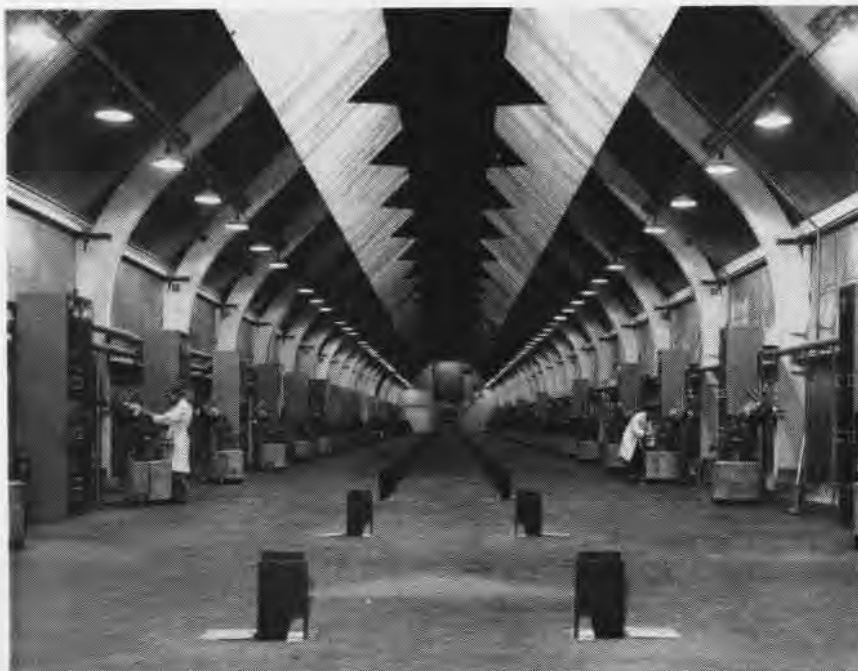
FREE FLIGHT OF MISSILE AND ROCKET MODELS IS STUDIED IN AEROBALLISTICS LAB
