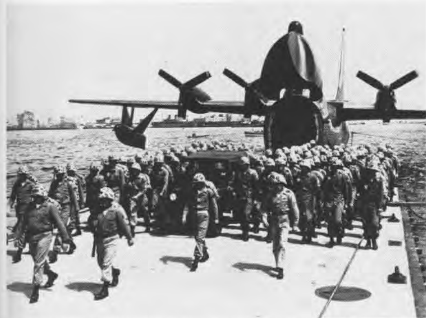
R3Y-2 CALLED 'FLYING LST,' CAN DISCHARGE MEN AND CARGO DIRECTLY ON THE BEACH
