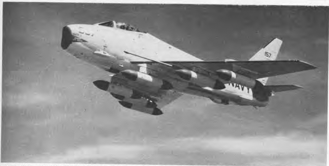
FJ-4B ATTACK AIRCRAFT CARRIES LOAD OF SIX ROCKET PACKS. AFTER DELIVERING THE STORES, THE PLANE DOUBLES AS A FIGHTER
