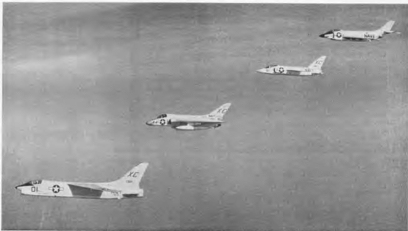
BEARING THE XC MARKING OF VX-3, THESE JETS ARE NOW UNDERGOING EVALUATION. L. TO R. ARE THE F8U, F4D, F11F, F3H-2N
