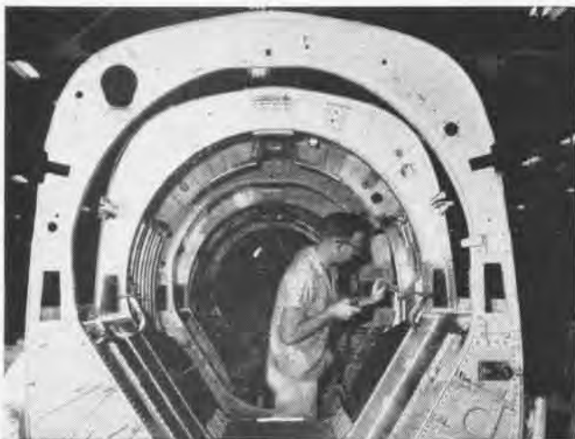
CRUSADER'S CENTER FUSELAGE IS SUB-ASSEMBLED IN FACTORY
