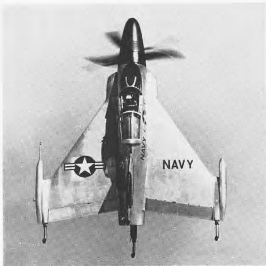
XFV-1 POGO WAS WORLD'S FIRST VERTICAL TAKE-OFF AND LANDING FIXED-WING PLANE
