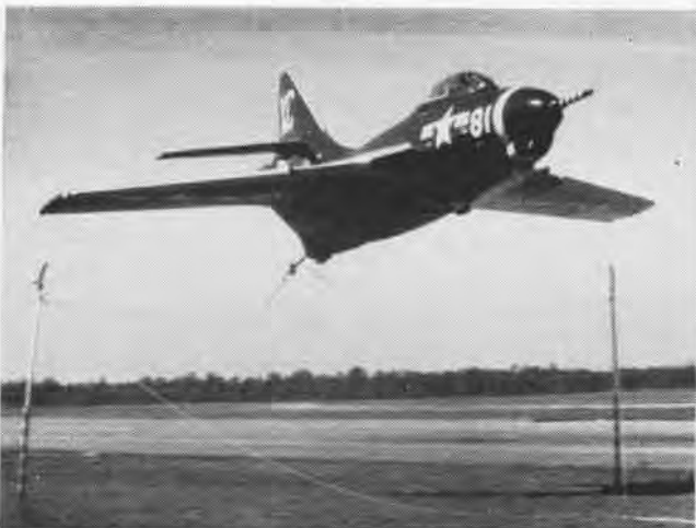
F9F-8 OF VX-3 MAKES SNATCH PICK-UP OF DART TOW TARGET
