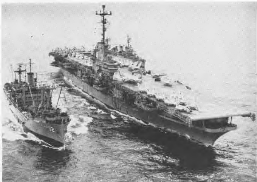
TO MAINTAIN full operational readiness of the Lake Champlain during Sixth Fleet exercises in the Mediterranean, the supply ship Altair, AKS-32, comes alongside for at-sea replenishment
