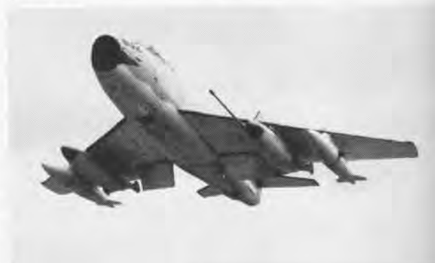
FOUR EXTERNAL FUEL TANKS GIVE FURY 'BRAVO' A HIGH RANGE
