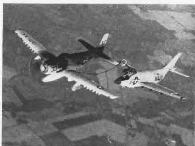
VX-3'S AD-6 AND F3H-2N TESTING AIR-TO-AIR REFUELING METHOD
