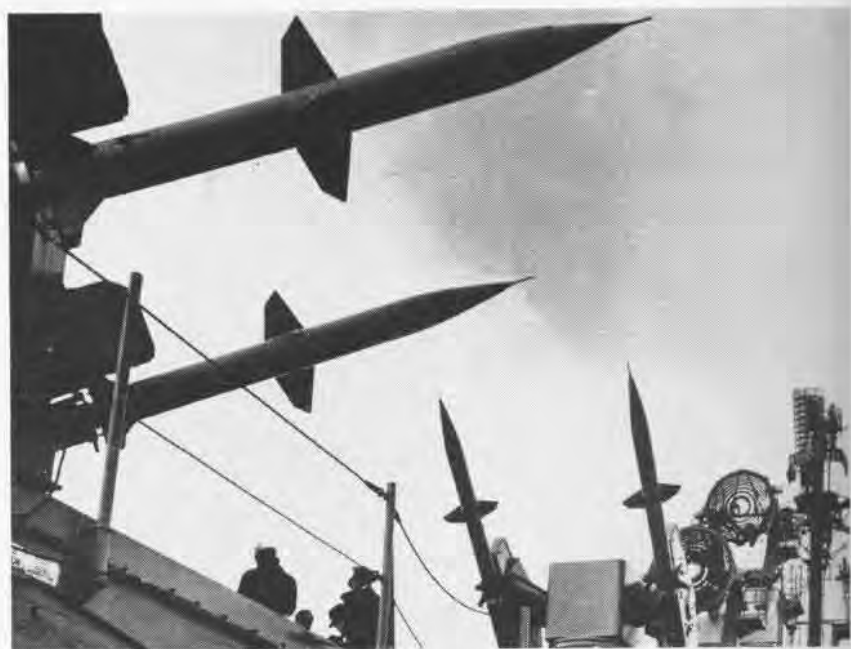
THE TERRIER, ABOARD USS BOSTON, IS A SURFACE-TO-AIR ANTI-AIRCRAFT GUIDED MISSILE
