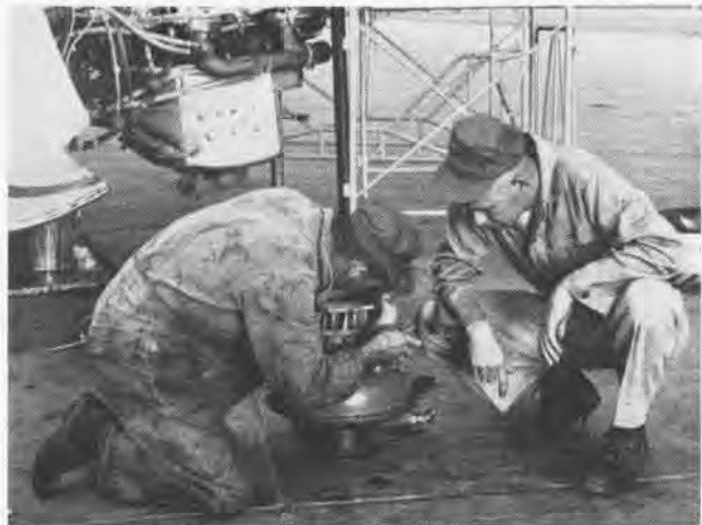
MAG-36'S MAINTENANCE squadron men perform an engine overhaul on an HUS helicopter, one of largest in use by USMC on West Coast.
