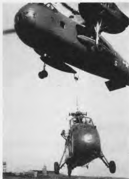
HR2S LIFTS HUS IN TEST AT NEW RIVER
