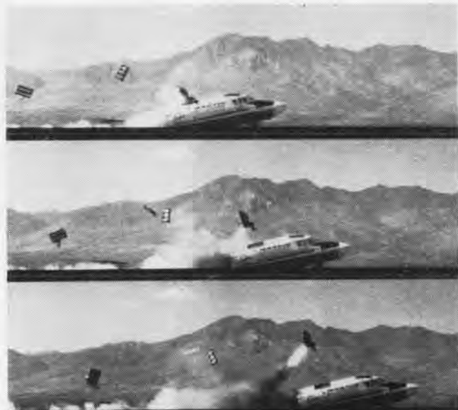
P6M SEAT IS ROCKET-PROPELLED CLEAR OF AFT HATCH POSITION
