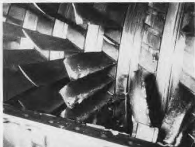
BLAST CAUSED BY AFTERBURNER CUT-IN SHEARED COMPRESSOR BLADES IN THIS JET. THE PROBLEM WAS TO LEARN CAUSE AND CURE
