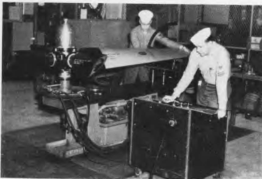
FASRON-103 Propeller Shop personnel have found a way to save up to four man-hours in checking a propeller dome without removing the complete propeller assembly from the aircraft. Their solution was to take a scrapped prop, cut off three blades about 20 inches from the hub, and remove the fourth blade. A new blade is inserted into the missing slot to test pitch angle. Dome leaks, blade pitch angle and fuel flow can be tested in the shop before prop installation.
