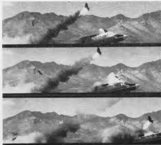
ROCKETS PROPEL FIRST SEAT AS SECOND SEAT EMERGES FORWARD
