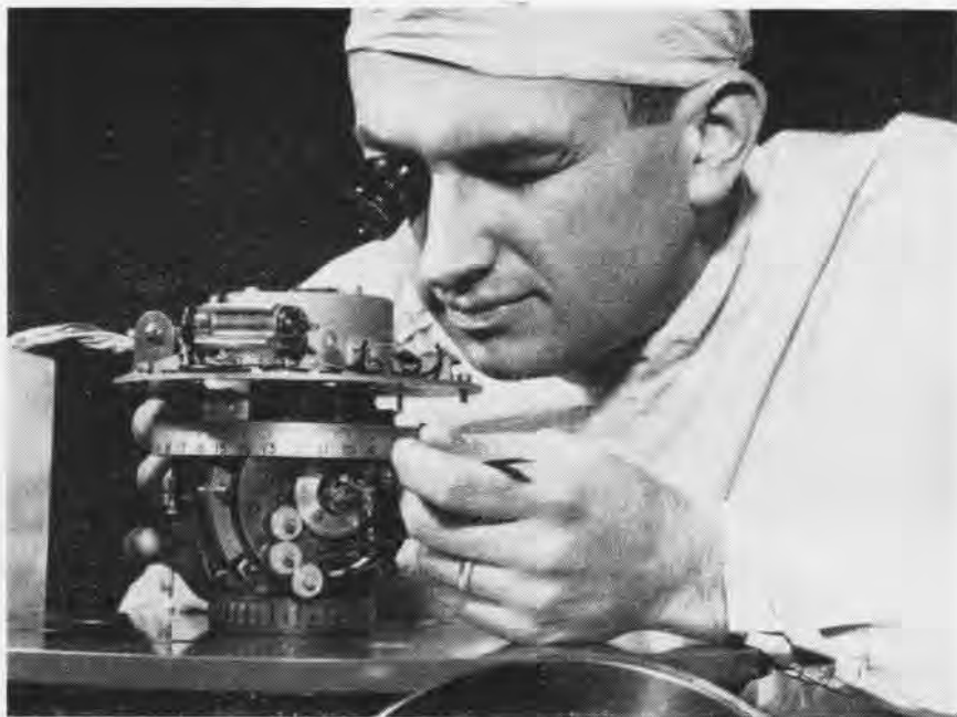
A 'SIMPLE' GYRO IS CHECKED IN DUST FREE CHAMBER BY SPERRY ENGINEER J. WILSON
