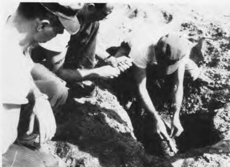
LINEAR CHARGE IS PLACED ON CASING TO OPEN CASE WITHOUT EXPLODING FILLER
