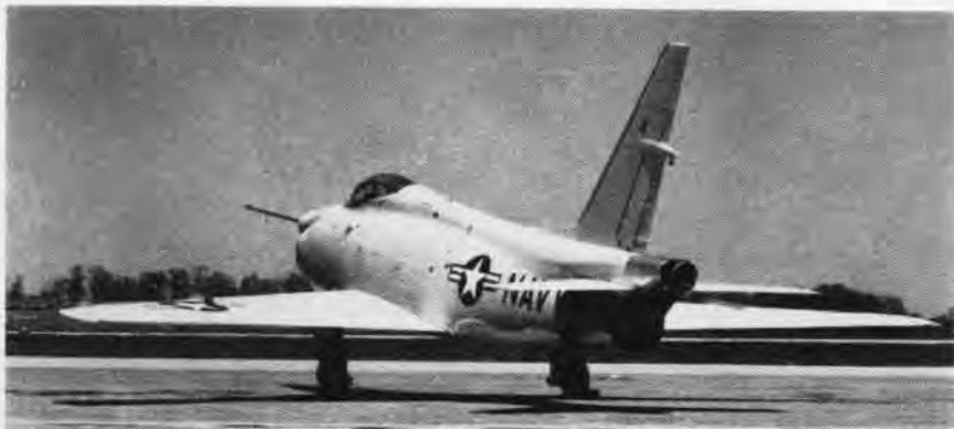
ROCKET-POWER -augmented F1-4F Furies, featuring a new North American Aviation rocket engine, the AR-1, are currently being tested at the Naval Air Test Center, Patuxent River. The AR-1, which operates in conjunction with the Fury's standard turbojet engine and burns hydrogen peroxide and conventional JP-4 fuel, gives significant increases in speed and altitude. The Fury shown is standard F1-4, modified as an experimental aircraft to test rocket power.
