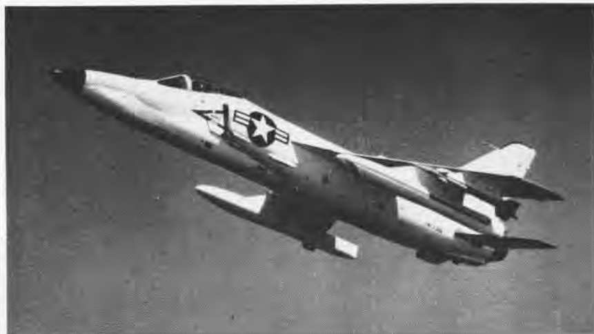
GRUMMAN F11F-1 Tiger packs a mighty wallop, the deadly Sidewinder air-to-air missile. The carrier-based fighter, first to incorporate the "area rule" (pinched waist) concept in its fuselage design, has recently completed a full demonstration of its Sidewinder lannobing capability in all flight conditions. The Sidewinder is a Navy infra-red weapon that can be used by current carrier-based fighters and attack aircraft to augment their offensive capabilities.
