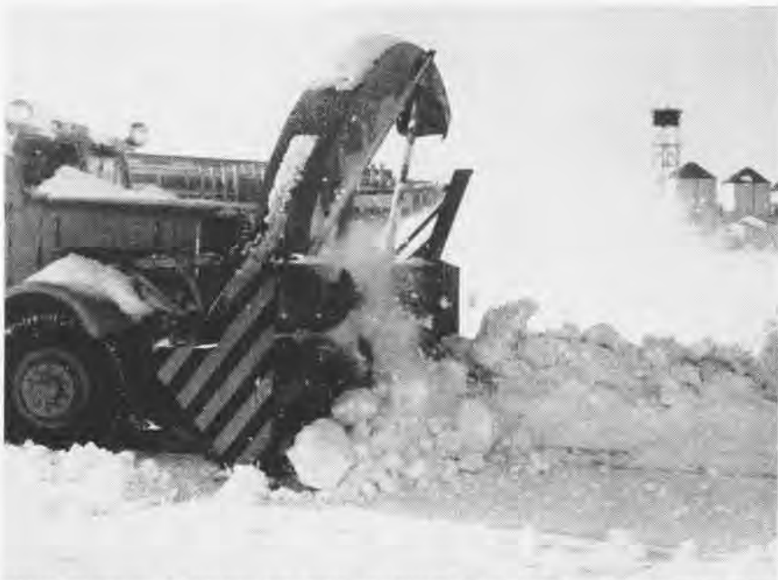
BLADES MOUNTED ON SNOWPLOW CHURN UP HARD PACKED SNOW ALONG RUNWAY EDGES
