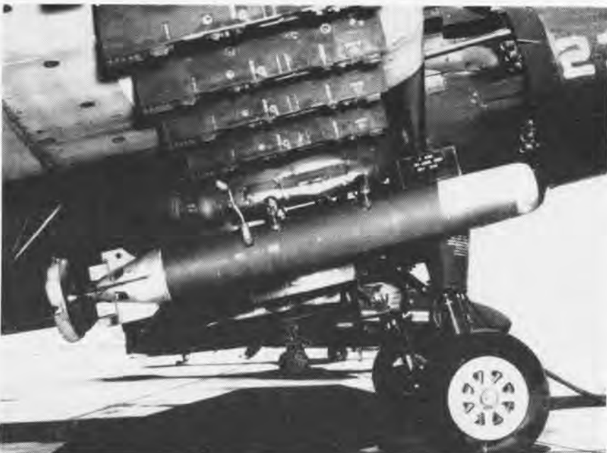
THE NAVY'S LATEST acoustic torpedo, the Mk. 43, developed by the Navy can drop into the sea, track down and sink submarines. It is already operational with the fleet. Constructed of light weight materials, it can be launched as easily from aircraft as from surface ships. The acoustic-homing type torpedo is actually a submersible guided missile and is capable of searching to great depths for enemy targets. It was developed for BuOrd by the Clevite Corporation.
