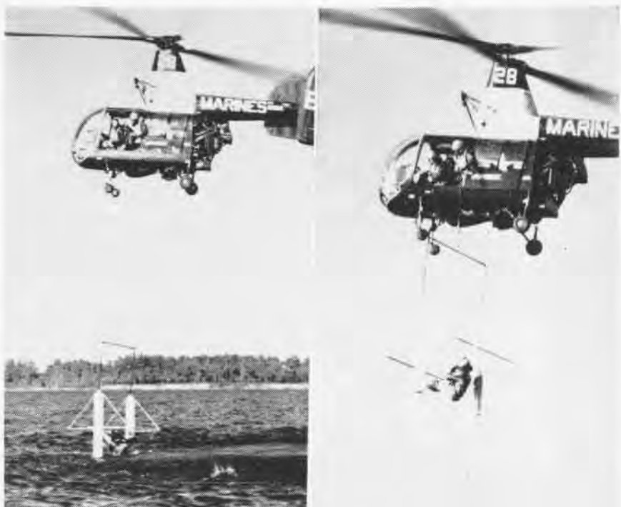
GETTING SCOOPED! Marine Sgt. W. M. Hughes, a simulated casualty, draws a free ride as he takes part in the evaluation trials of a new helicopter rescue hoist at Camp Lejeune, N. C. Employing the air-sea rescue method recently developed by the Naval Medical Field Research Laboratory, the 'copter lifted Sgt. Hughes by coming up behind and using its net as a scoop.
