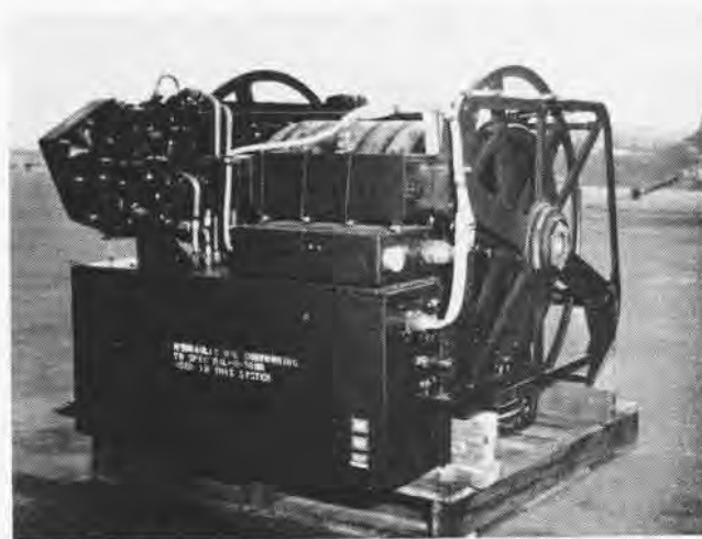
ONE OF FOUR hose reel units used in pods on wing of R3Y. Each reel has hose capacity of 105 feet. Fuel flow rate is 250 gpm.
