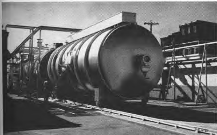
VACUUM TEST CHAMBER built by Convair at San Diego under $1 million Air Force contract can house fuselage of F-106A Delta Dart interceptor for high-speed heat and high-altitude pressure tests. Half of test chamber is mounted on wheels so it may be rolled away from
