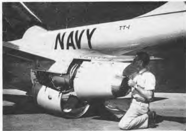
THE POWER PLANT IS A CONTINENTAL J-69-T-9 TURBOJET ENGINE
