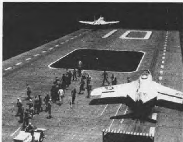
AS WHITLOCK takes off, deck crew gets prepared to launch an F9F-8 Cougar. Ship can launch ready planes on "cats" four seconds apart.
