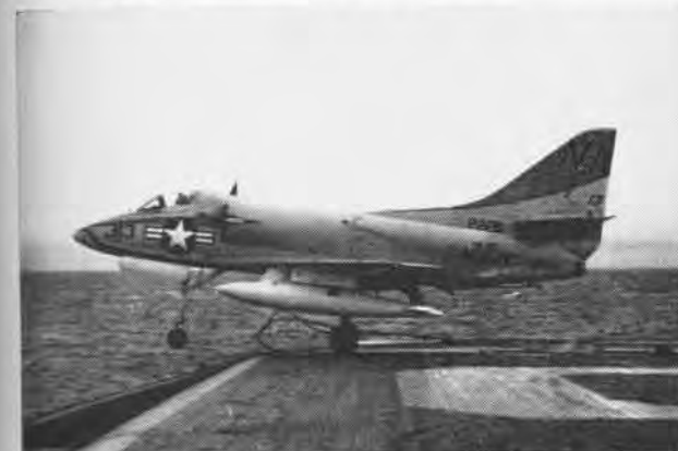
CATAPULT BRIDLE falls free of VA-113 Skyhawk following steam cat shot on Hancock during carquals. Note assortment of 13's on A4D.
