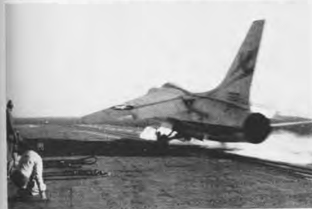
INITIAL ACCELERATION of the world's fastest carrier fighter blurs aircraft as catapult crew watches first West Coast carrier ops of F8U-1.
