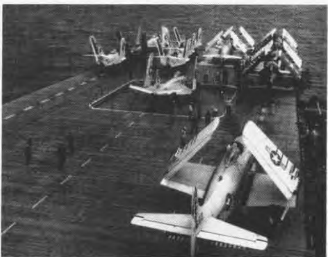
WINGS FOLDED, Whitlock's Banshee takes elevator to the carrier's hangar deck where maintenance crew will ready it for next mission.
