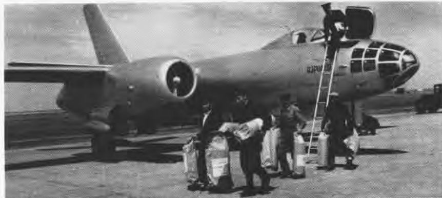
AT A SOVIET airport, all hands get the mail off. Prior to the introduction of the new Camel (Tu-104), twin-jet transport, the Soviets pioneered domestic air routes with converted Beagle twin-jet bombers (Il-28's). The Beagles were used to carry high priority light freight and mail.
