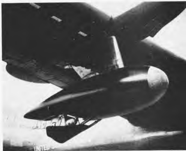
STREAMLINED fiberglass aluminum honeycomb core pods beneath R3Y engine nacelles house individual hose reels, drogue rewind gear.
