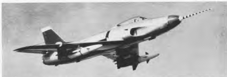
ATTACK MISSILES for the Royal Swedish Air Force are shown mounted on the Saab-32 Lansen all-weather attack aircraft. These Swedish-developed air-to-surface guided missiles, designated type 304, are now undergoing intensive trials before their introduction into actual SAF service.
