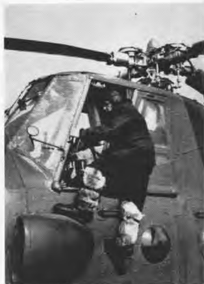
THE HOUND helicopter is widely used by the USSR and her satellite air forces. It has a four-blade motor and can carry a lightweight jeep which enters the copter through clam-shell doors in the aft end of the fuselage.
