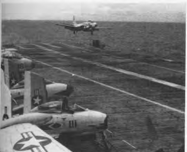
RETURNING pilot takes a "bolter," goes around again. Angled decks, mirror landing system, steam "cats" make carrier operations safer.
