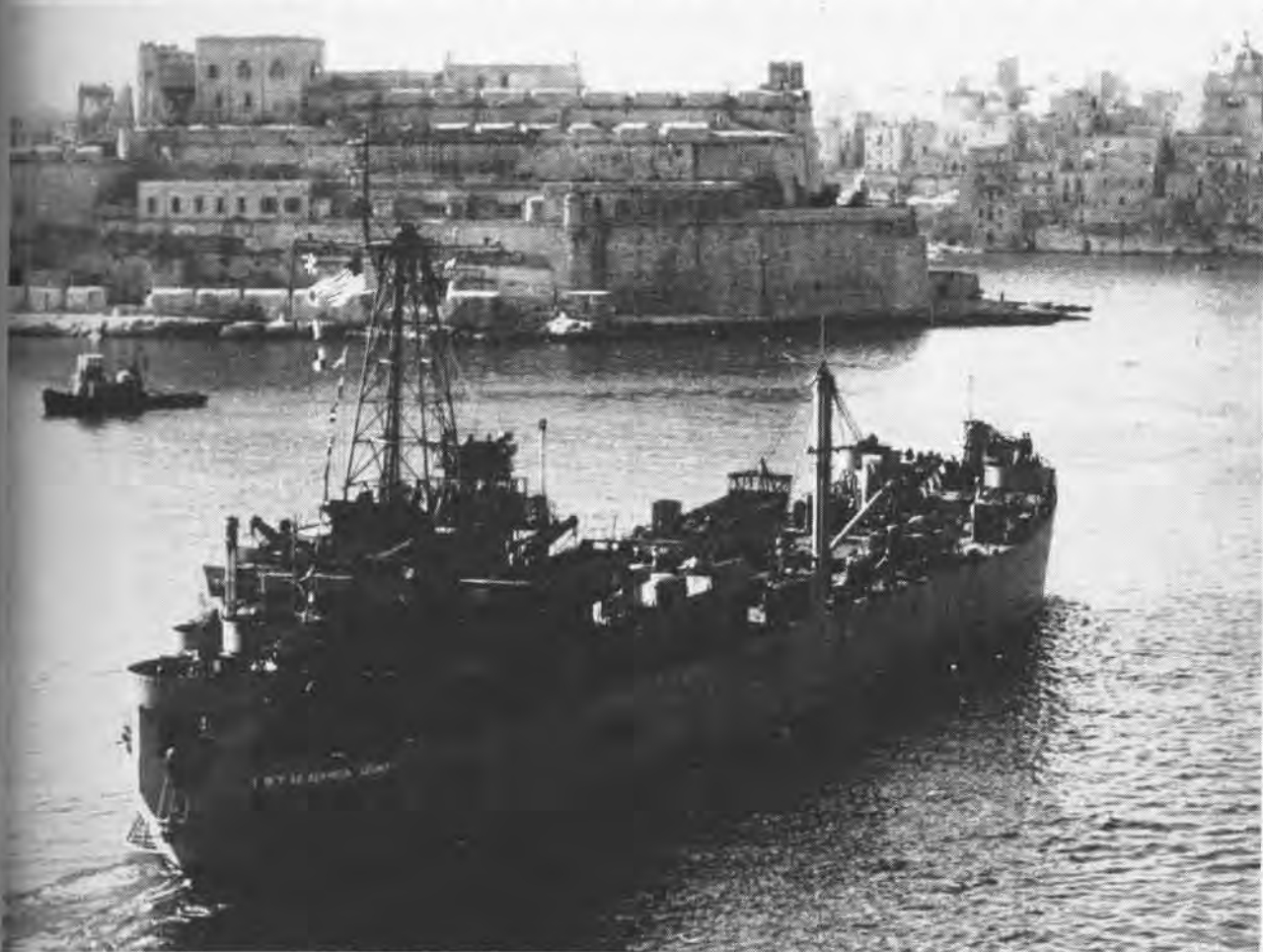
USS ALAMEDA COUNTY, converted from LST-32 to AVB-1, is Navy's first Advanced Base Ship. She can land men and equipment to place a
