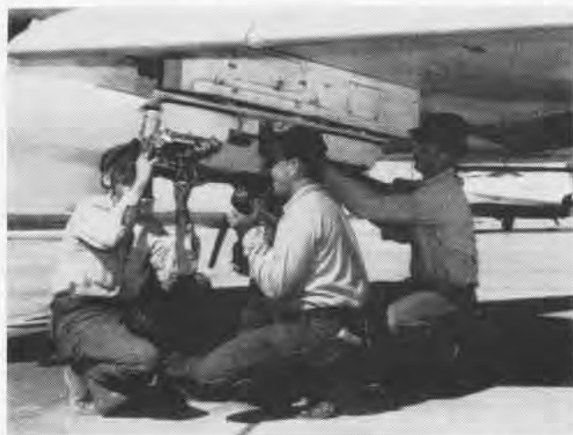
ORDNANCE CREW loads bombs on A4D-1. During Gitmo deployment VA-72 dropped over 3500 of these 25-pound practice bombs on targets.
