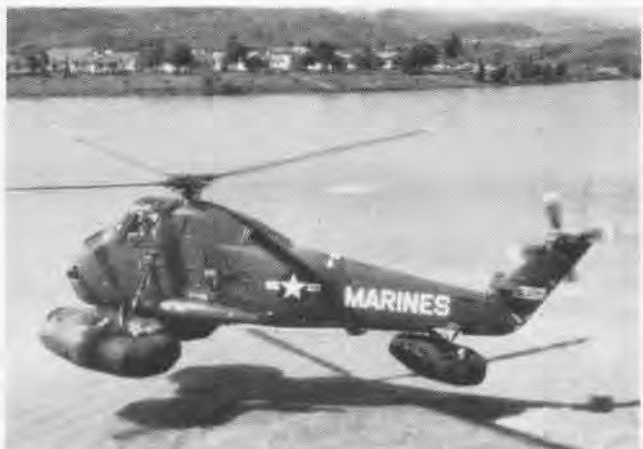
"Hussy" down on Lake O'Neill at Camp Pendleton. First Lt. R. A. Bruton, flying with Col. Johnson, made the second landing (left). This modified HUS-1 permits landing at sea in emergencies and may also be used in rescue and search missions. The HUS-1A can land on relatively rough water and may be towed by surface craft at sea.
