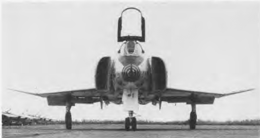
LATEST NAVY JET , the McDonnell F4H-1 taxis out (top) prior to first flight at Lambert-St. Louis Municipal Airport. Designed to fly at speeds better than twice the speed of sound, the two-place, carrier-based interceptor is powered by two GE J-79 jet engines. The new F4H features a 45-degree sweptback wing and a horizontal tail that slopes downward at 23 degrees to provide for superior handling characteristics at all speeds. The plane is 56 feet long with a wingspan of 38 feet 5 inches. Capable of all-weather operations, it will, company officials say, carry improved missiles and is rigged for conventional or nuclear bomb delivery.
