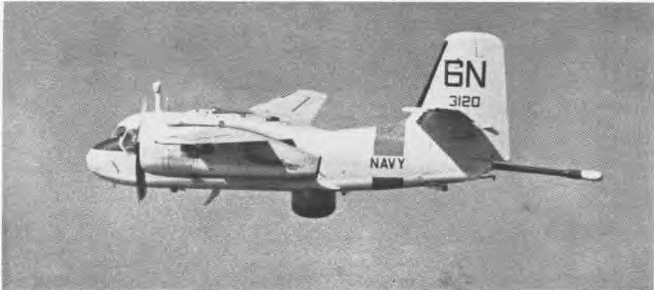
THE HUNTER—THIS CLOSE-UP OF THE S2F TRACKER SHOWS RADOME AND STINGER, EYES AND EARS OF THE PLANE, IN EXTENDED POSITION
