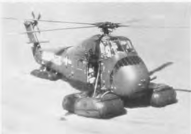
EMERGENCY WATER LANDINGS have been proved feasible for the HUS-1 in water landing tests made by Marine Air Group 36, stationed at MCAS El Toro, California. Col. R. J. Johnson, commanding officer of MAG-36, became the first West Coast helicopter pilot to make such a landing with the pontoon-equipped "Hussy." At right, the colonel sets the
