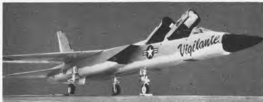
NORTH AMERICAN Aviation A3J Vigilante , all-weather attack weapons system designed for carrier operations, is powered by two General Electric J79-2 engines, each of which develops 15,000 pounds thrust. Scheduled for its first flight this summer, the two-place aircraft was christened by Admiral Arleigh A. Burke, Chief of Naval Operations, during special ceremonies at Columbus. The A3J features boundary layer control, automatic bombing-navigation system.
