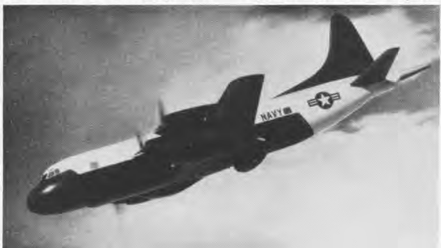
SUB-HUNTER VERSION of Lockheed's prop-jet Electra is shown as it will look when configured for fleet use. As the Navy's first turbine-powered ASW plane, it will be fitted with four Allison Model T56 engines developing a total of 16,200 hp at takeoff. The bulge beneath the fuselage accommodates radar installation and the plastic-cone-shaped tail extension houses "MAD" unit which locates submerged metallic objects by noting deviations in normal magnetic fields.
